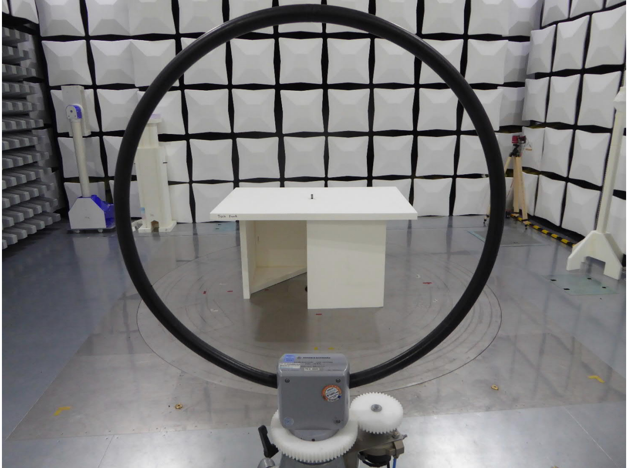
Test setup semi anechoic chamber TX spurious emissions from 9 kHz to 30 MHz
