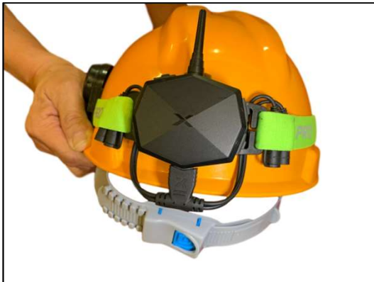
Completed helmet mounting set-up
