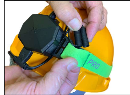
Insert 3.5mm connectors under strap and over into left and right strap pockets
