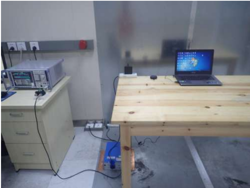
FCC RADIATED EMISSION TEST SETUP
