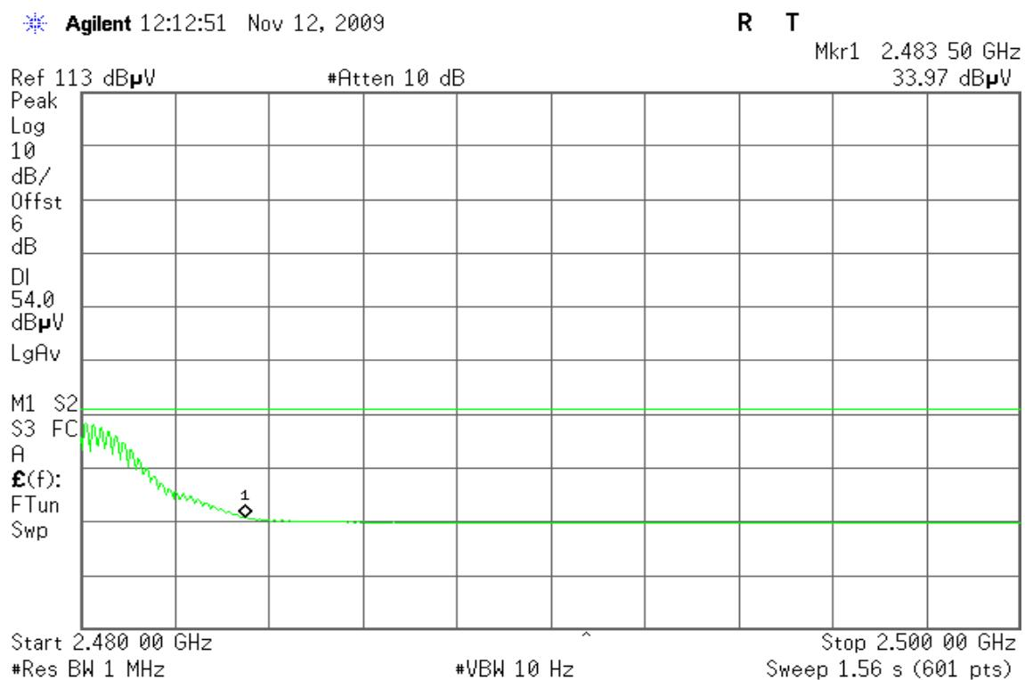
**Band Edges (Bluetooth 8DPSK / CH Low)****Detector mode: Peak****Polarity: Vertical**
