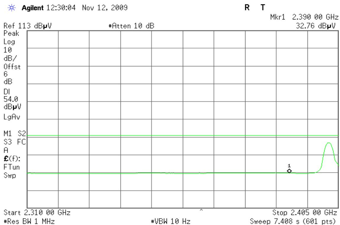
**Band Edges (Bluetooth 8DPSK / CH High)****Detector mode: Peak****Polarity: Vertical**
