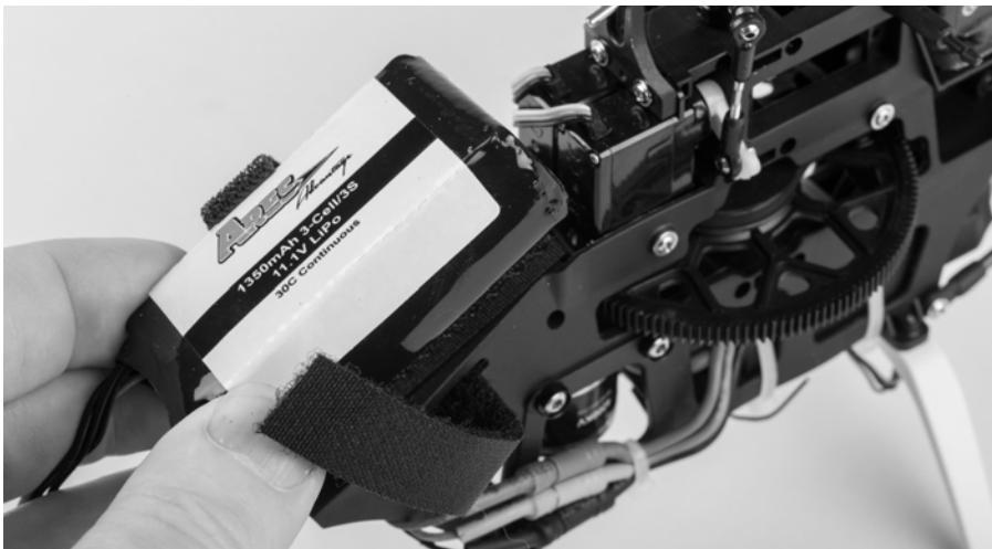
Attach the battery to the airframe using the included hook and loop tape. Secure the battery with the the hook and loop strap. Once the battery is in place it can now be connected to the ESC battery plug.
