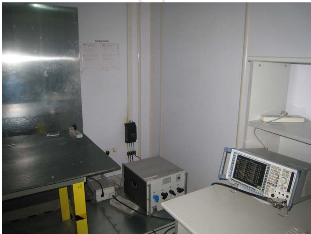
Conducted Emission Test Setup
