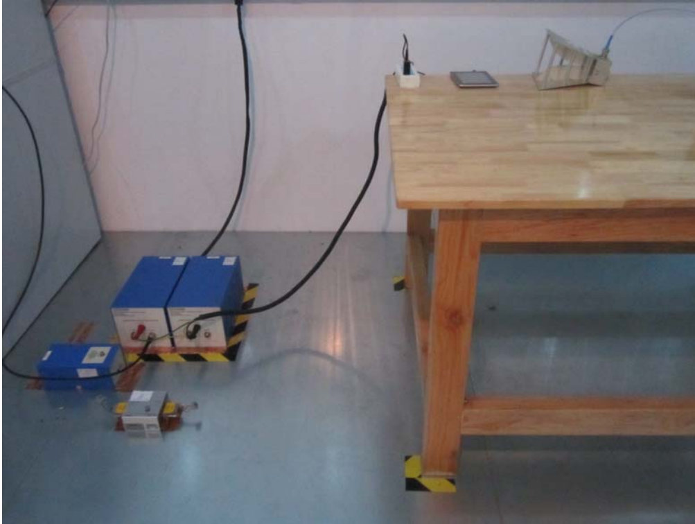
Conducted Emissions Test Setup Front View
