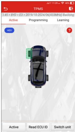
2. For universal sensors, place the TPMS antenna of the tool alongside the valve stem, point toward the sensor location, and tap **Activate** on the screen.
