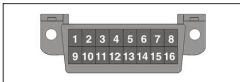
Note: Some 1994 and 1995 vehicles have 16-pin connectors but are not OBD II compliant. Only those vehicles with a Vehicle Emissions Control Label stating “OBD II Certified” are OBD II compliant.
