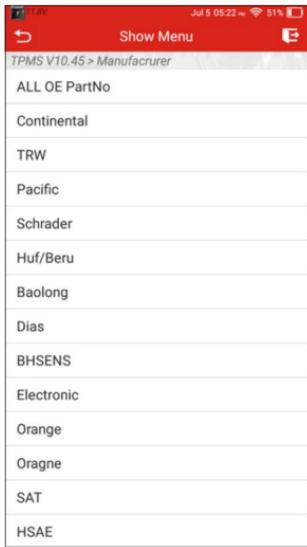
Tap the target sensor manufacturer to enter. Check the original manufacturer number on the body of the sensor, and tap the corresponding OE number on the screen to enter the following screen.
