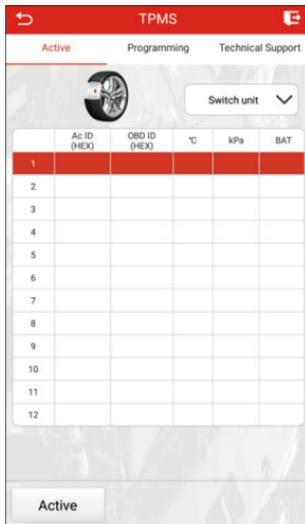
Tap **Activate** to trigger and check the sensor data.
