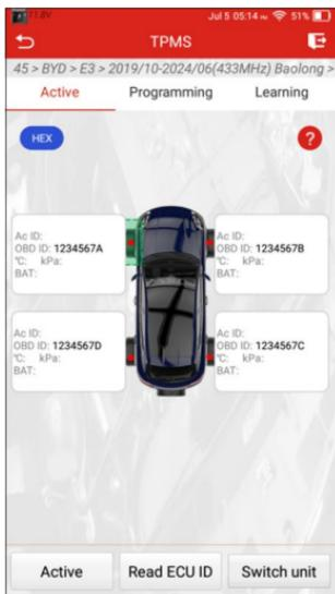
5. Place a new LAUNCH-specific sensor close to the TPMS antenna, select the desired wheel position and tap **Copy by OBD** to enter the following screen.
