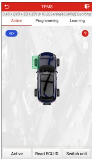
2. Tap **Read ECU ID**. Connect the tool to the vehicle's DLC port and tap **OK** to start reading the sensor IDs and positions for viewing.
