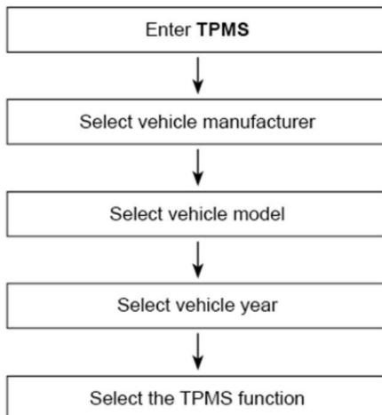
\*Note: For indirect TPMS vehicle, only the Relearning function is supported. For vehicle using Direct TPMS, it generally includes: Activation, Programming and Relearning. The available TPMS functions may vary for different vehicles being serviced.
