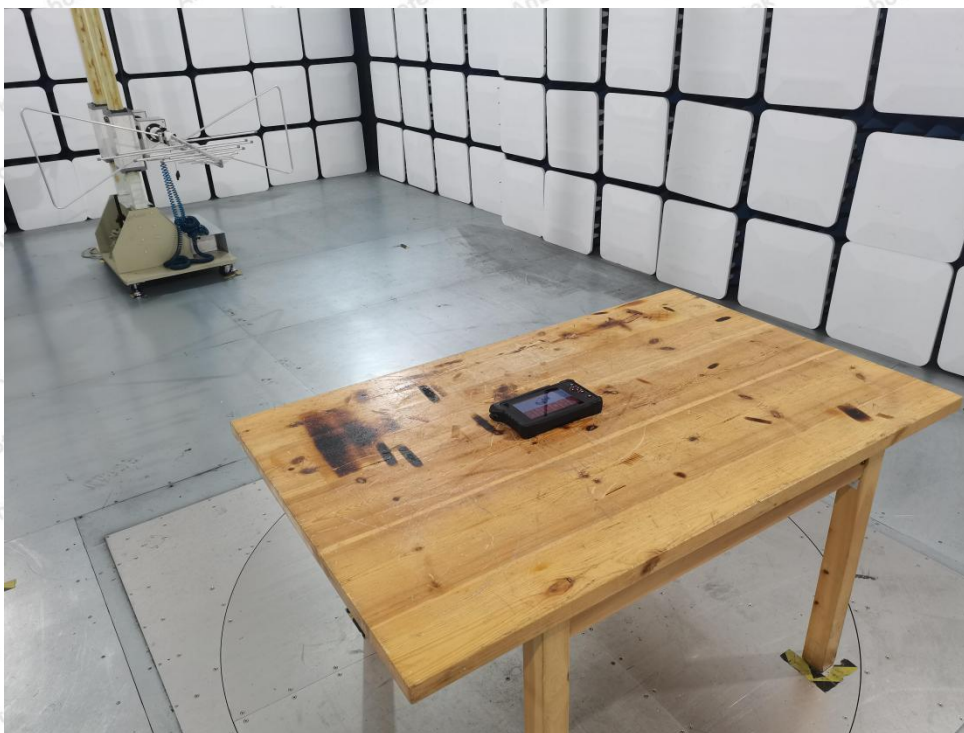
Photo of Radiation Emission Test
