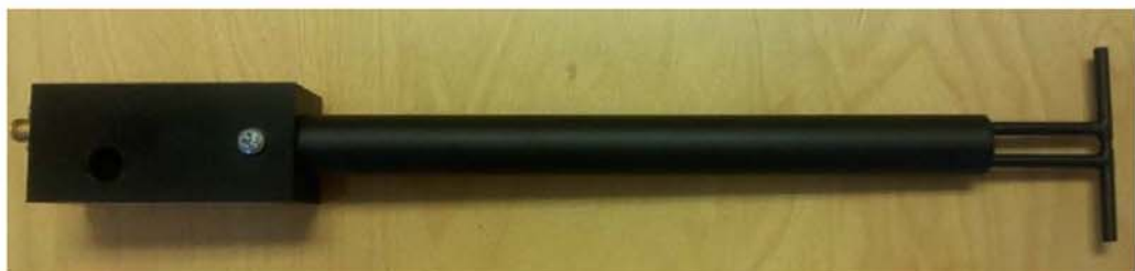
Figure 1 – MVG COMOSAR Validation Dipole
