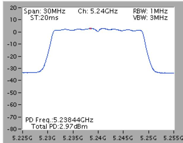
Power Density Plot on Configuration IEEE 802.11ac MCS0/Nss1 40MHz / Chain 1 + Chain 2 /
