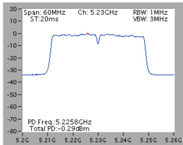
Power Density Plot on Configuration IEEE 802.11ac MCS0/Nss1 VHT 80MHz / Chain 1 + Chain 2 / 5210 MHz
