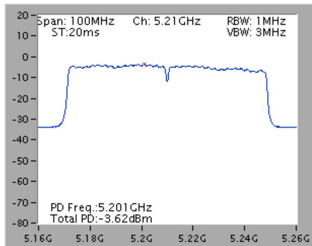
Power Density Plot on Configuration IEEE 802.11a / Chain 1 + Chain 2 / 5180 MHz
