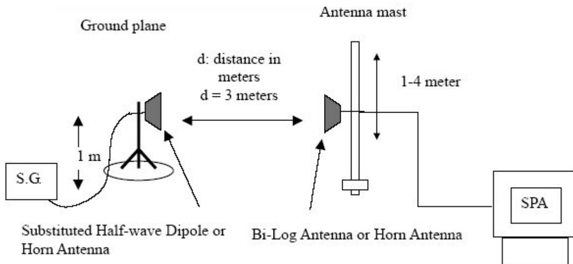
**Test procedure: Based on ANSI/TIA 603C: 2004**
