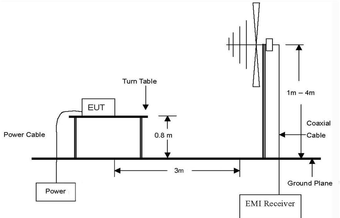
The diagram below shows the test setup that is utilized to make the measurements for emission from 1 GHz to 5 GHz Emissions.
