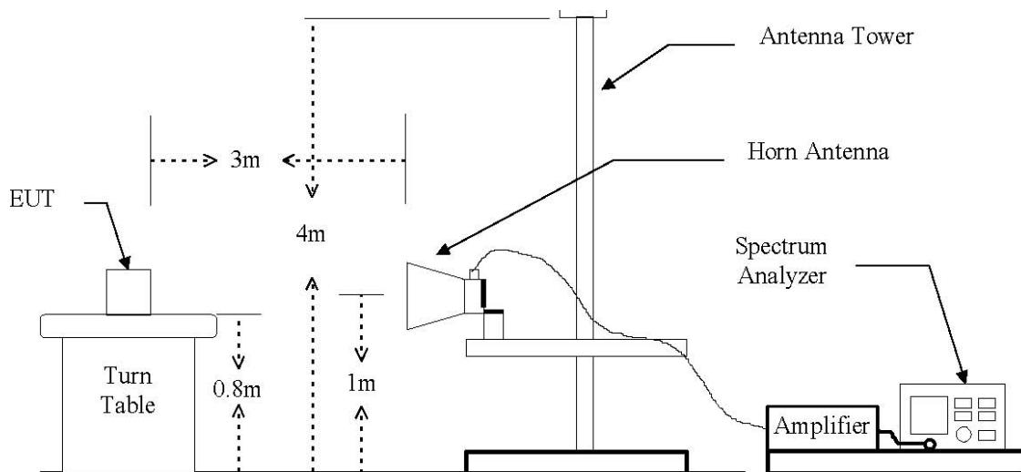
The diagram below shows the test setup for substituted method
