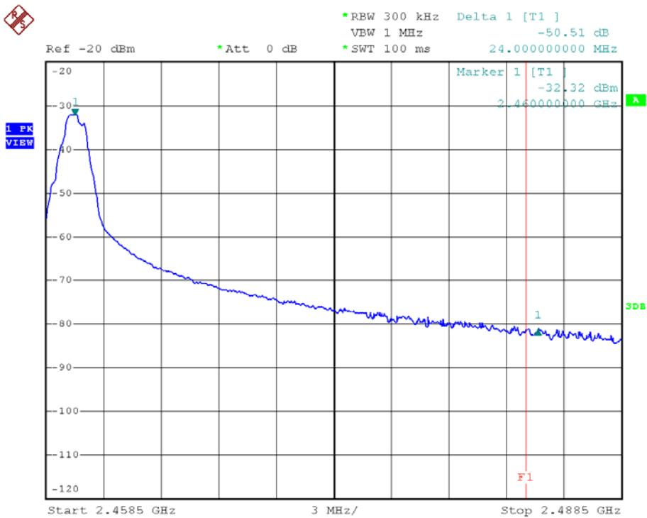
Bandedge Plot – Pursuant to FCC Part 15 Section 15. 249 Requirement (Pass)
