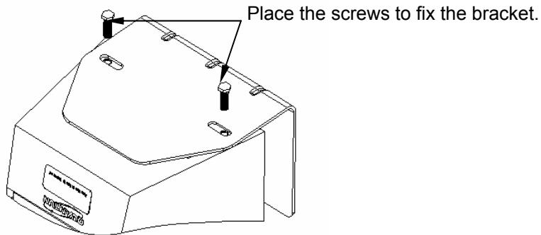
Place the screws to fix the bracket.
