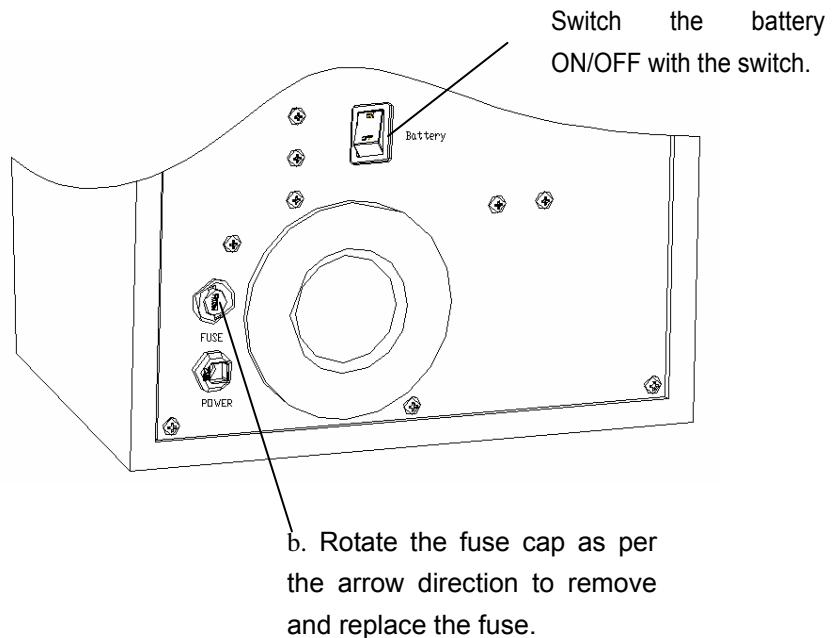
Switch the battery ON/OFF with the switch.
