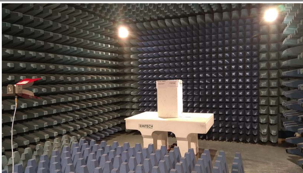
TEST SETUP PHOTO(S) RADIATED EMISSIONS ( F > 1\text{GHz} )
