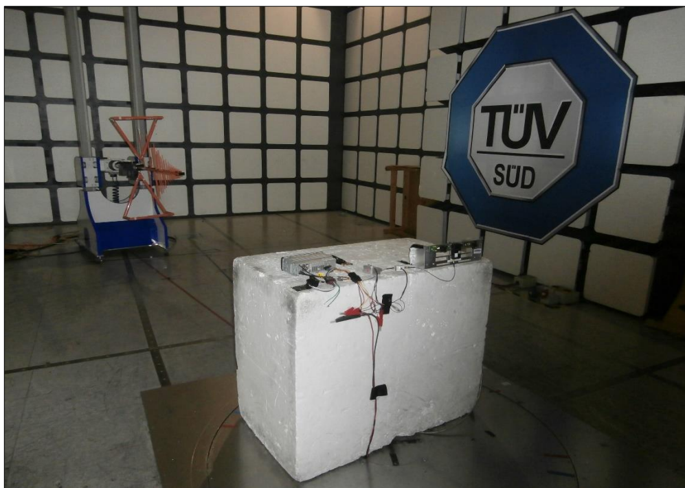
Figure 10 - Test Setup - Below 1 GHz
