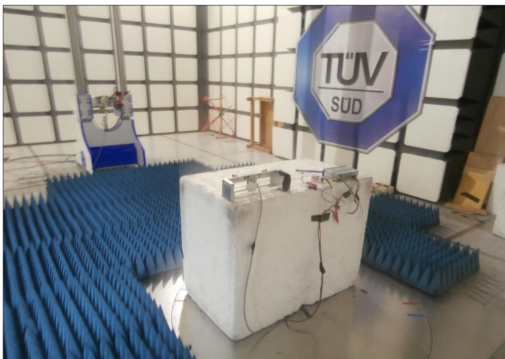
Figure 11 - Test Setup - Above 1 GHz
