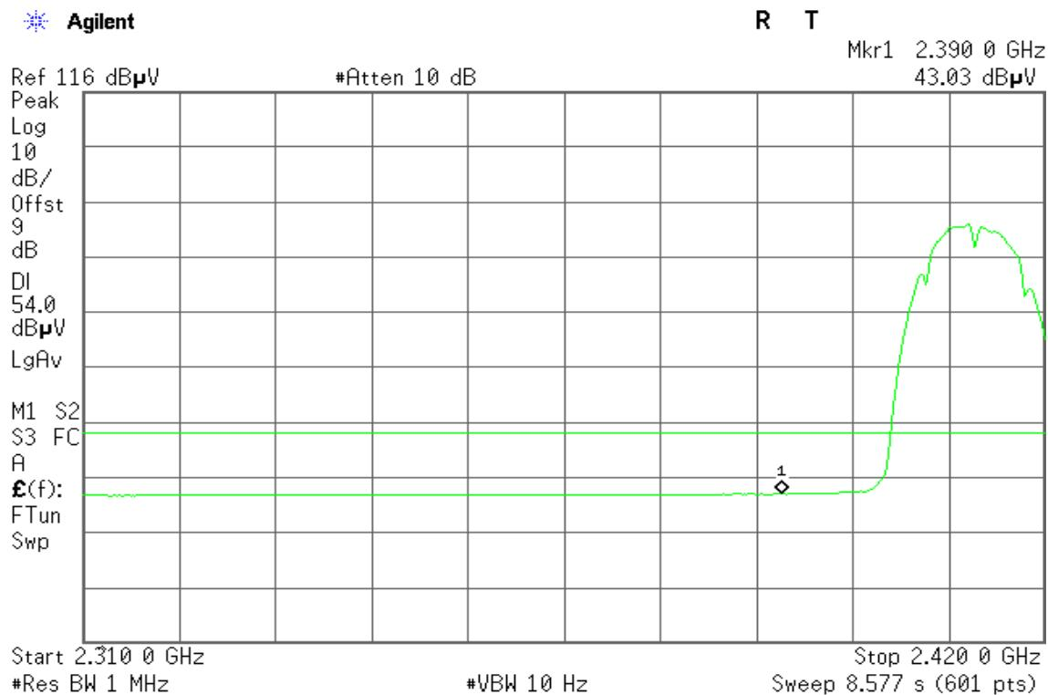
**Band Edges (IEEE 802.11b / CH High)****Detector mode: Peak****Polarity: Vertical**
