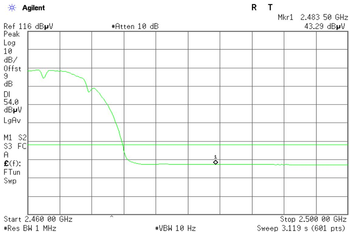
**Band Edges (IEEE 802.11g / CH Low)****Detector mode: Peak****Polarity: Vertical**
