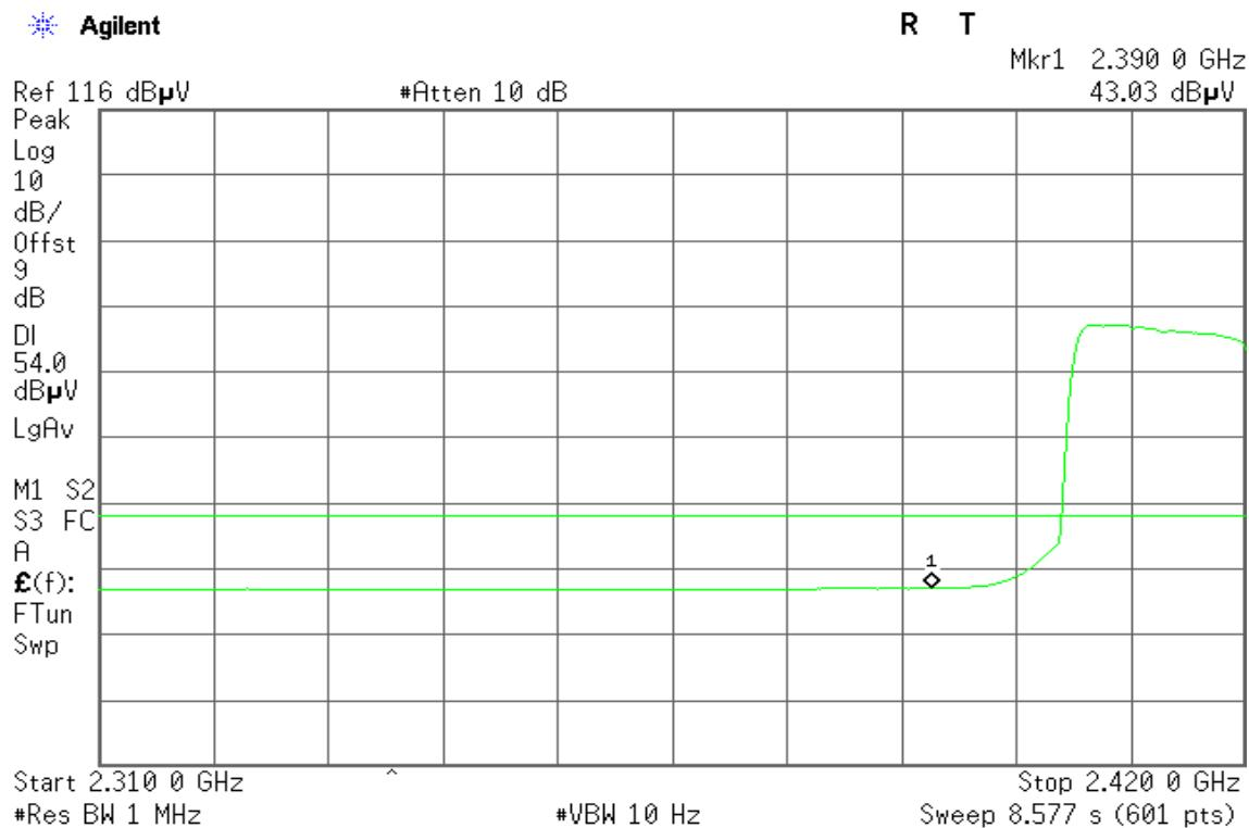
**Band Edges (IEEE 802.11g / CH High)****Detector mode: Peak****Polarity: Vertical**
