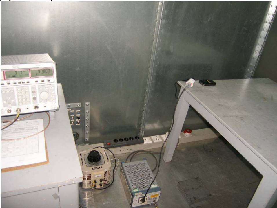
Photograph 2: Set-up for Conducted Emissions
