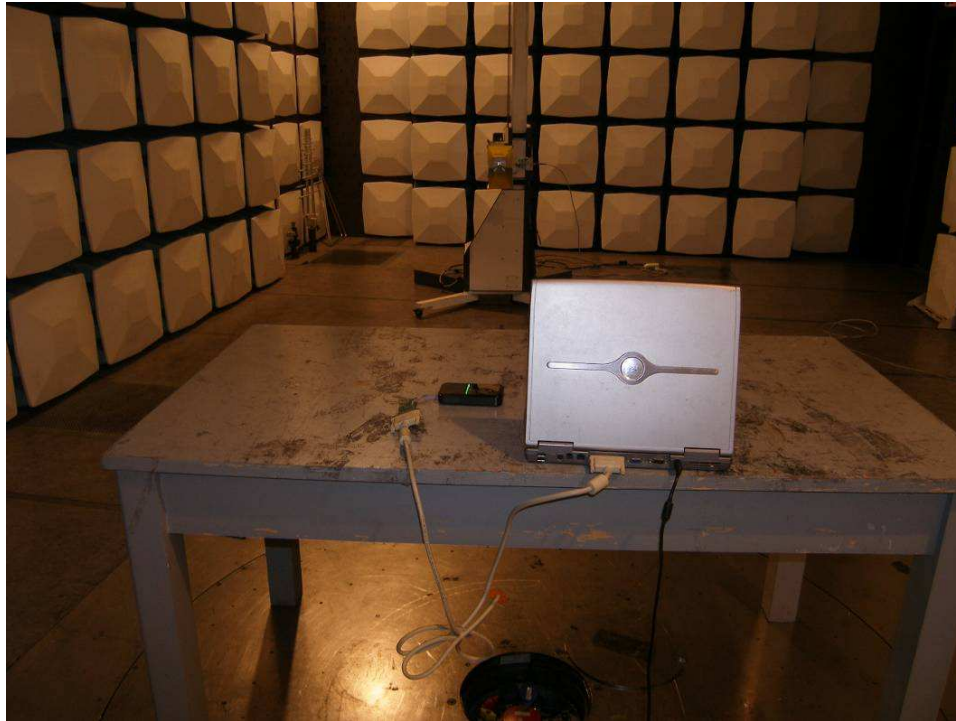
Photograph 6: Set-up for Spurious Emissions (18GHz-26GHz)
