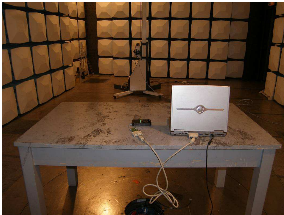
Photograph 6: Set-up for Spurious Emissions (18GHz-26GHz)
