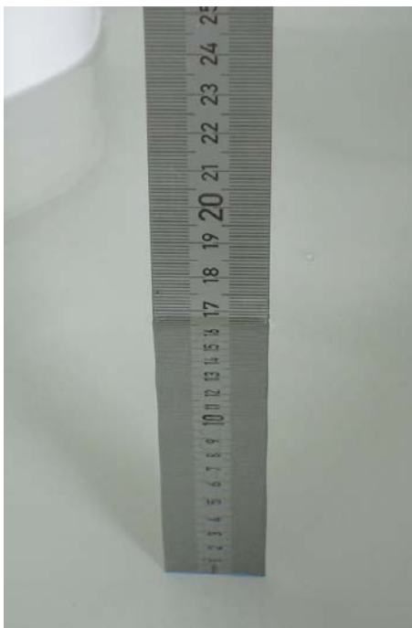
Fig. 15: Liquid depth for IEEE 802.11b body measurements.
