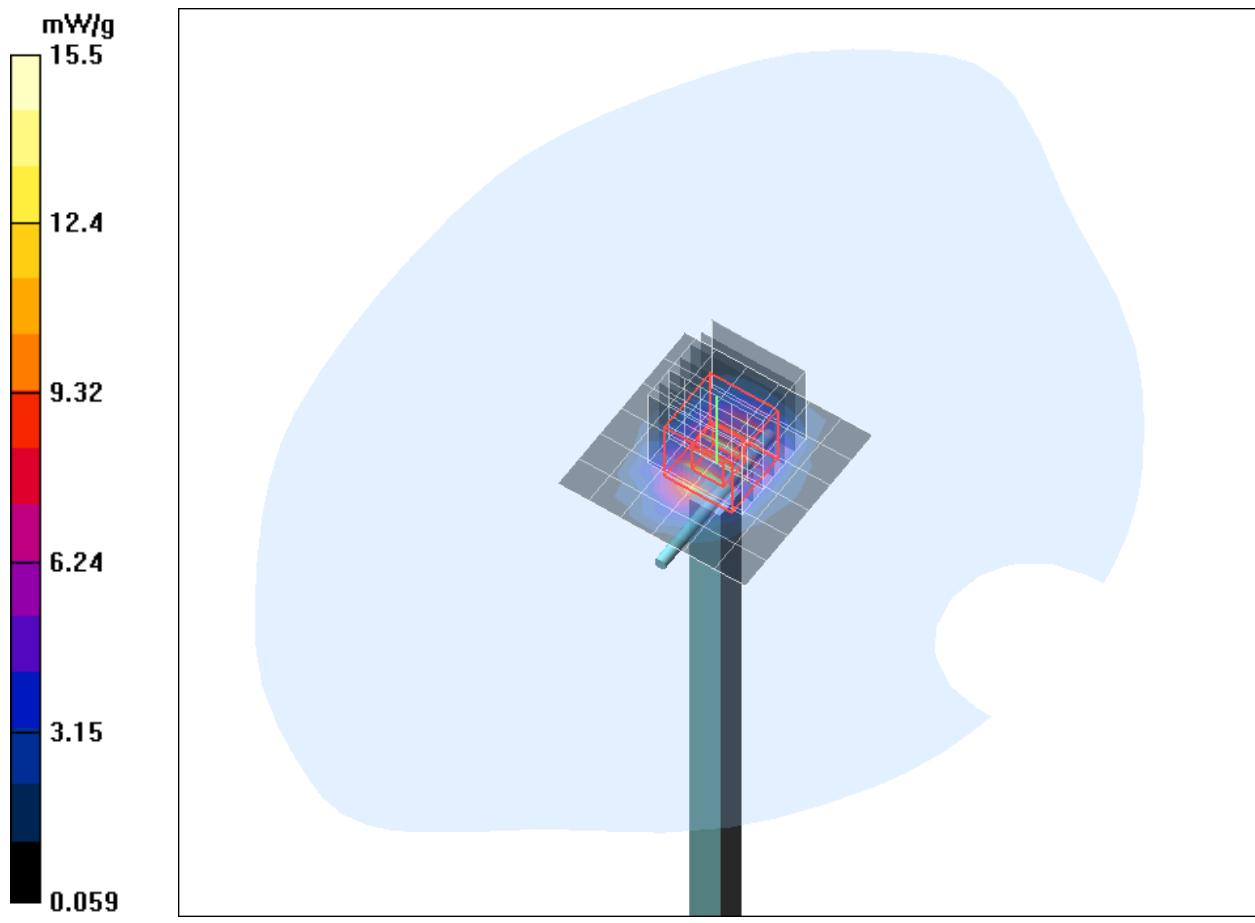
**SAR Result with Body TSL****Test Laboratory: IMST GmbH, DASY Blue (I); File Name: [260913\\_b\\_3536.da4](#)****DUT: Dipole 2450 MHz SN: 709; Type: D2450V2; Serial: D2450V2 - SN:709****Program Name: System Performance Check at 2450 MHz**
