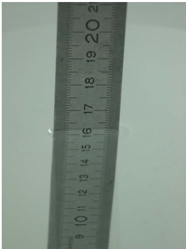
Fig. 12: Liquid depth for IEEE 802.11 body worn measurements.
