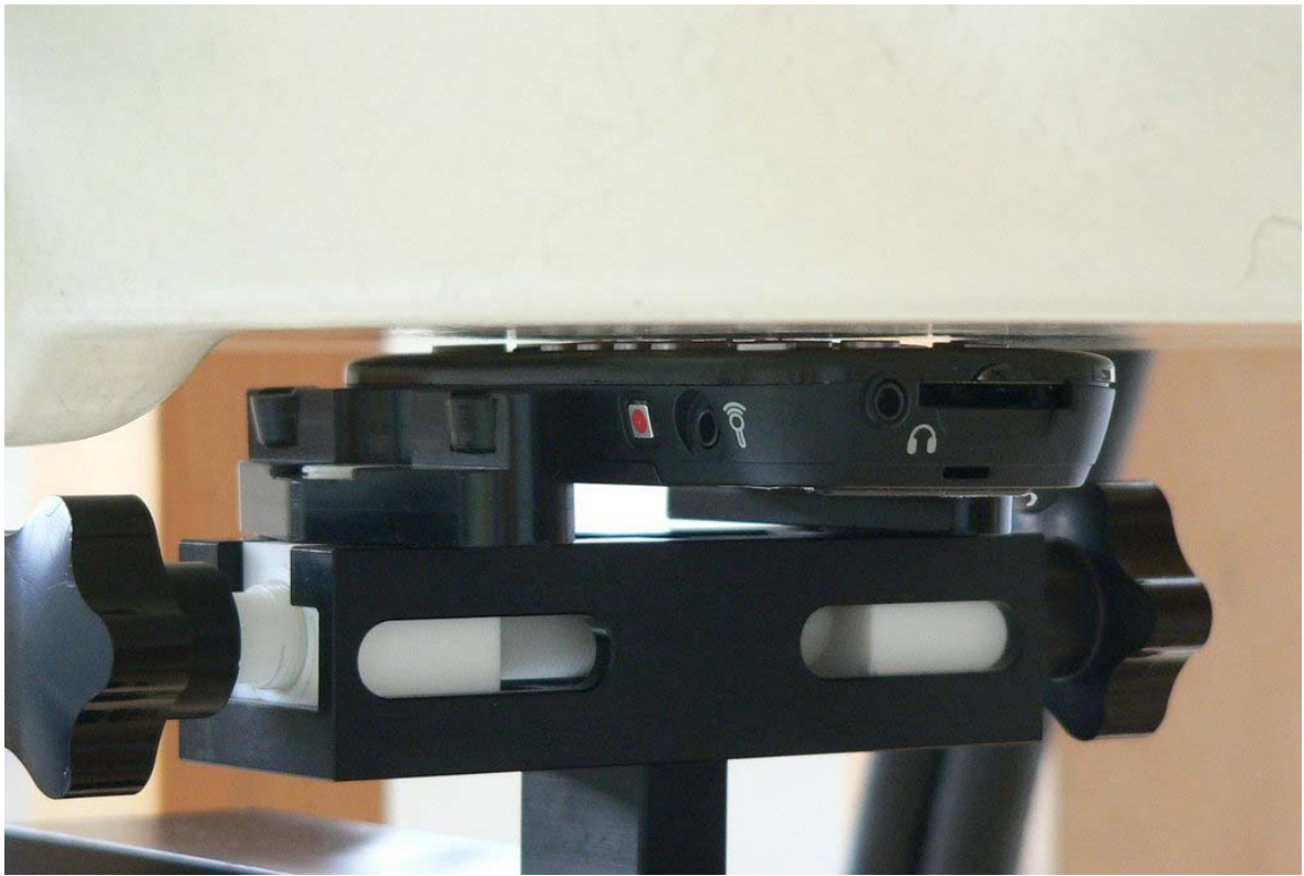
Fig. 10: Body worn configuration, position 1, front towards the phantom.
