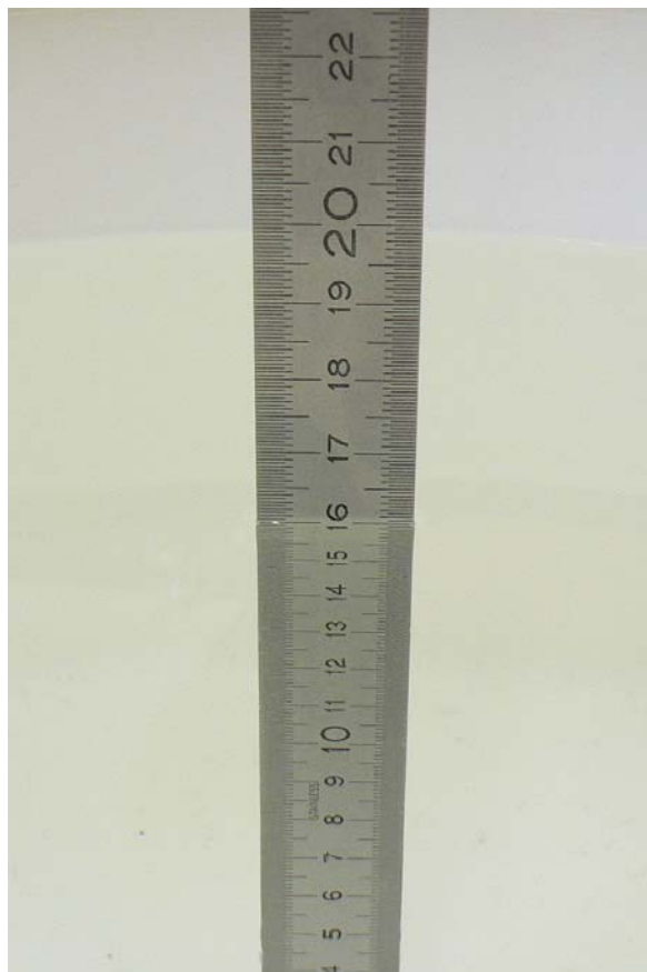
Fig. 14: Liquid depth for IEEE 802.11 head measurements.
