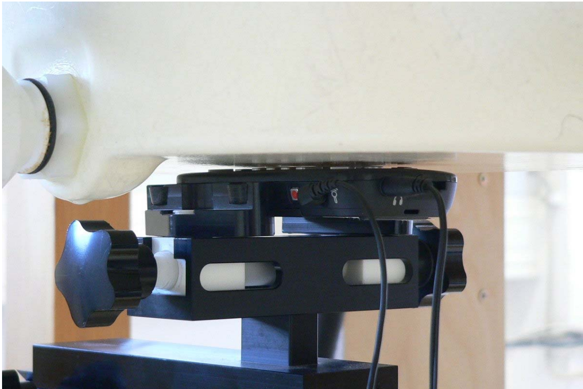
Fig. 12: Body worn configuration, position 1, front towards the phantom, with attached headphones and microphone.
