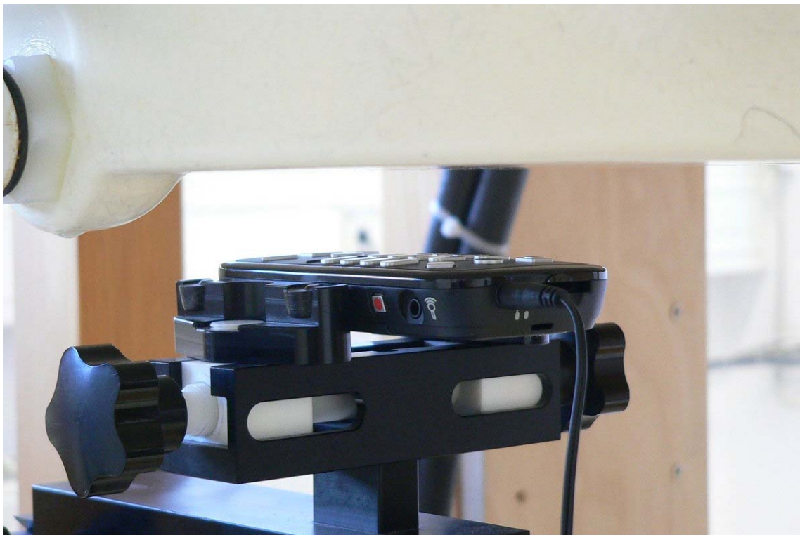
Fig. 13: PTT configuration, position 2, 25 mm distance, front towards the phantom, with attached headphones .
