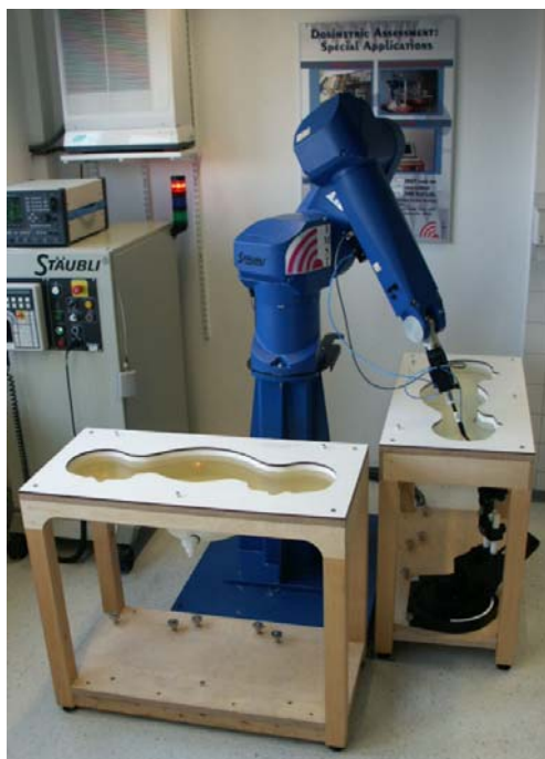
Fig. 3: The measurement set-up with two SAM phantoms containing tissue simulating liquid.
