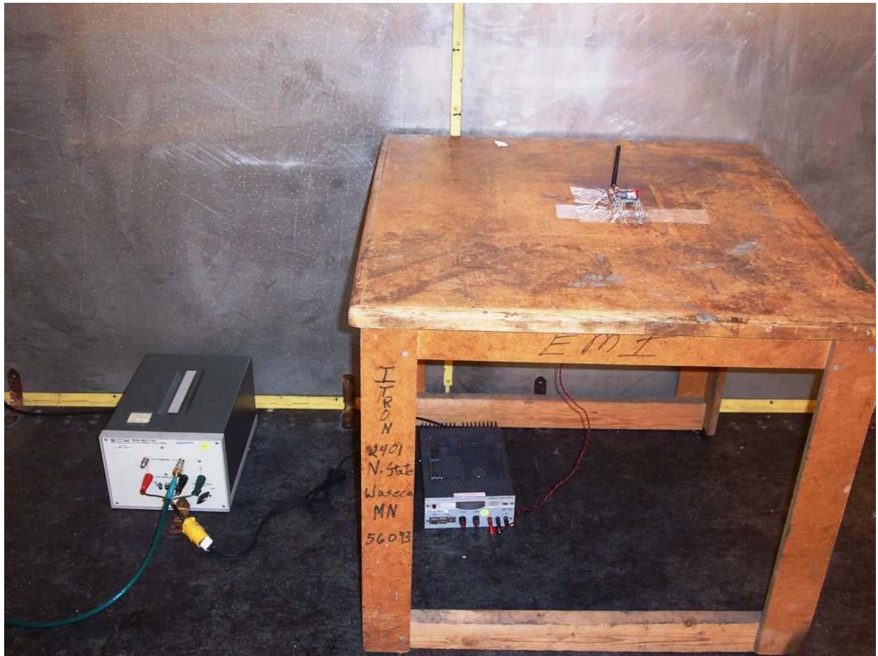
Photo 23: AC line conducted measurement with 2dBi vertical whip
