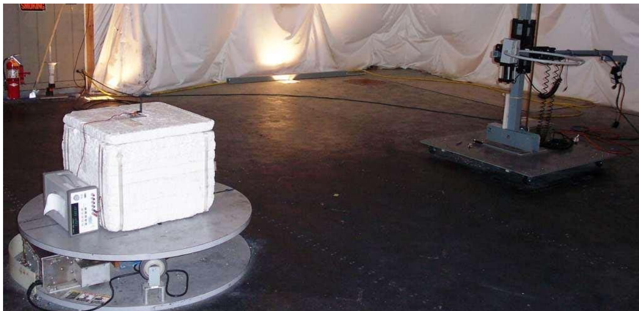
Photo 3: Test setup for radiated spurious between 9kHz and 30MHz with EMCO 6502 Loop Antenna shown and Alektrona AIM4M1 Module. using 2dBi whip in vertical orientation
