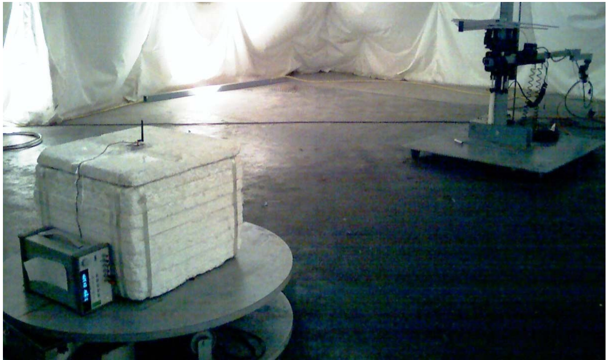
Photo 9: Test setup for radiated spurious between 200MHz and 2GHz with EMCO 3148 Log Periodic in horizontal orientation shown and Alektrona AIM4M1 Module using 2dBi whip in vertical orientation
