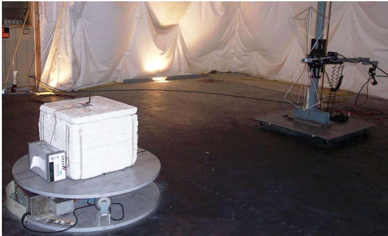
Photo 5: Test Setup for Radiated Spurious measurements between 30MHz and 300MHz using EMCO 3110B Biconical antenna in vertical orientation and Elektrona AIM4M1 Module using 2dBi whip in vertical orientation
