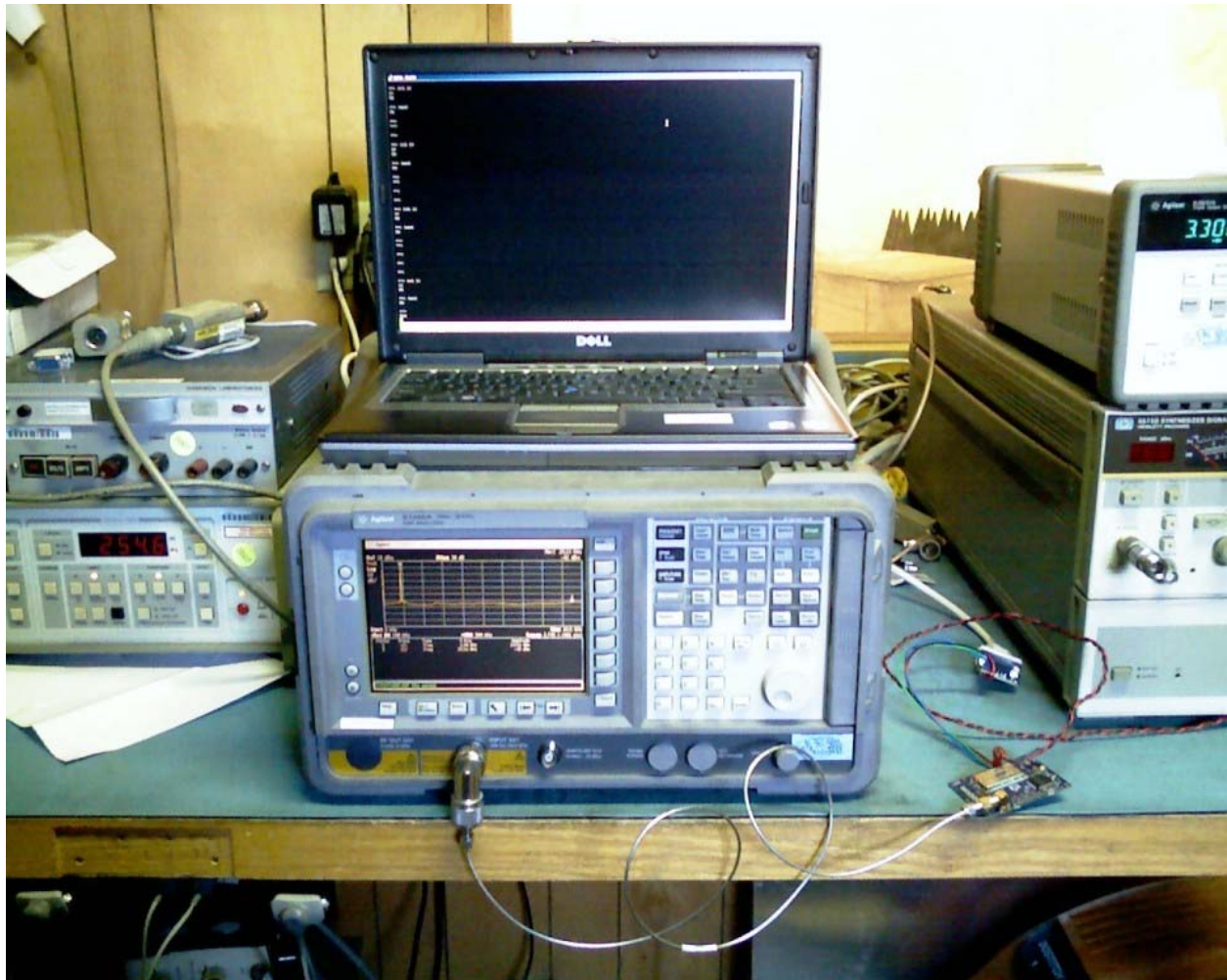
Photo 21: TX conducted spurious measurement with Alektrona AIM4M1 Module board and Agilent E7405A Spectrum Analyzer
