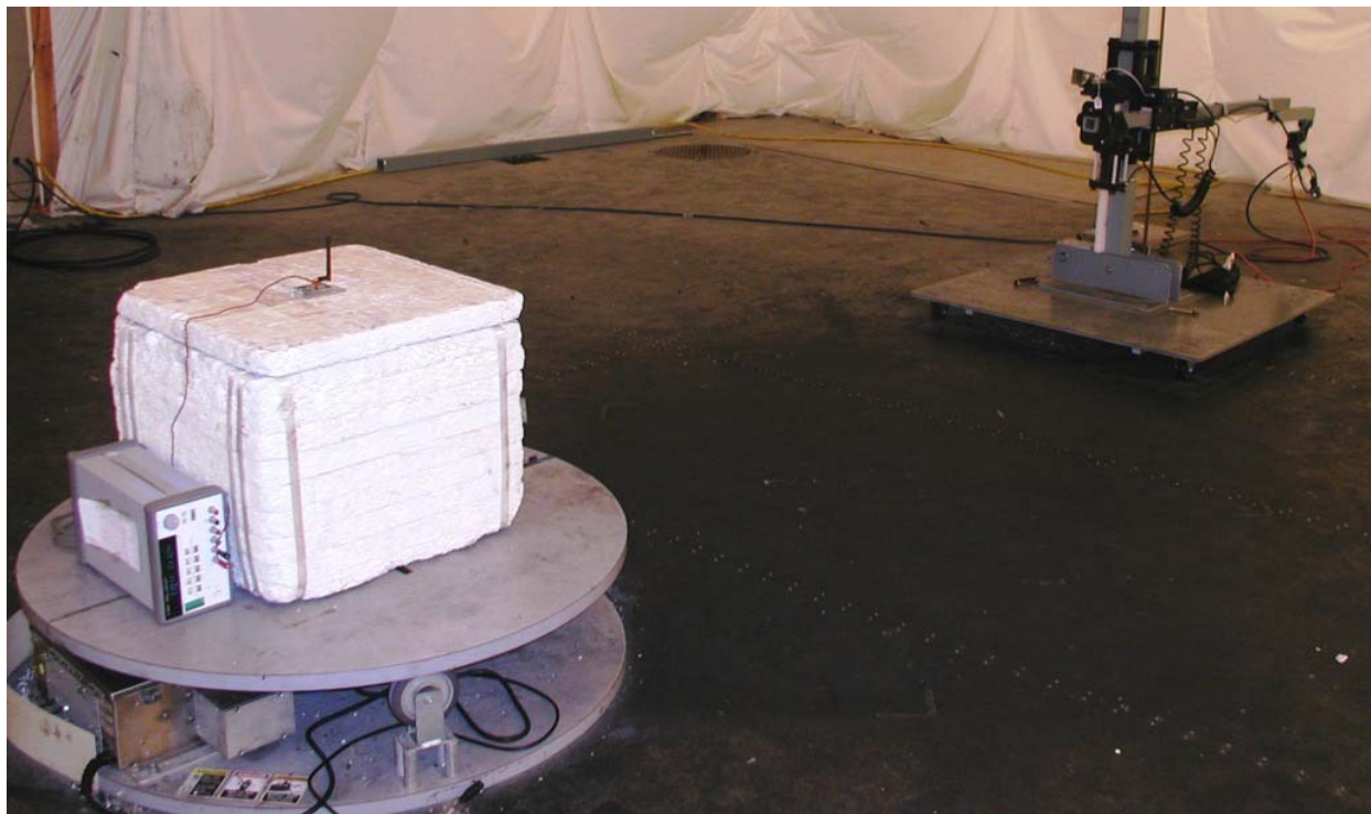
Photo 19: Test setup for radiated spurious emissions above 18GHz with AH Systems SAS-572 horn antenna in horizontal polarity and Alektrona AIM4M1 Module using 2dBi whip in vertical orientation
