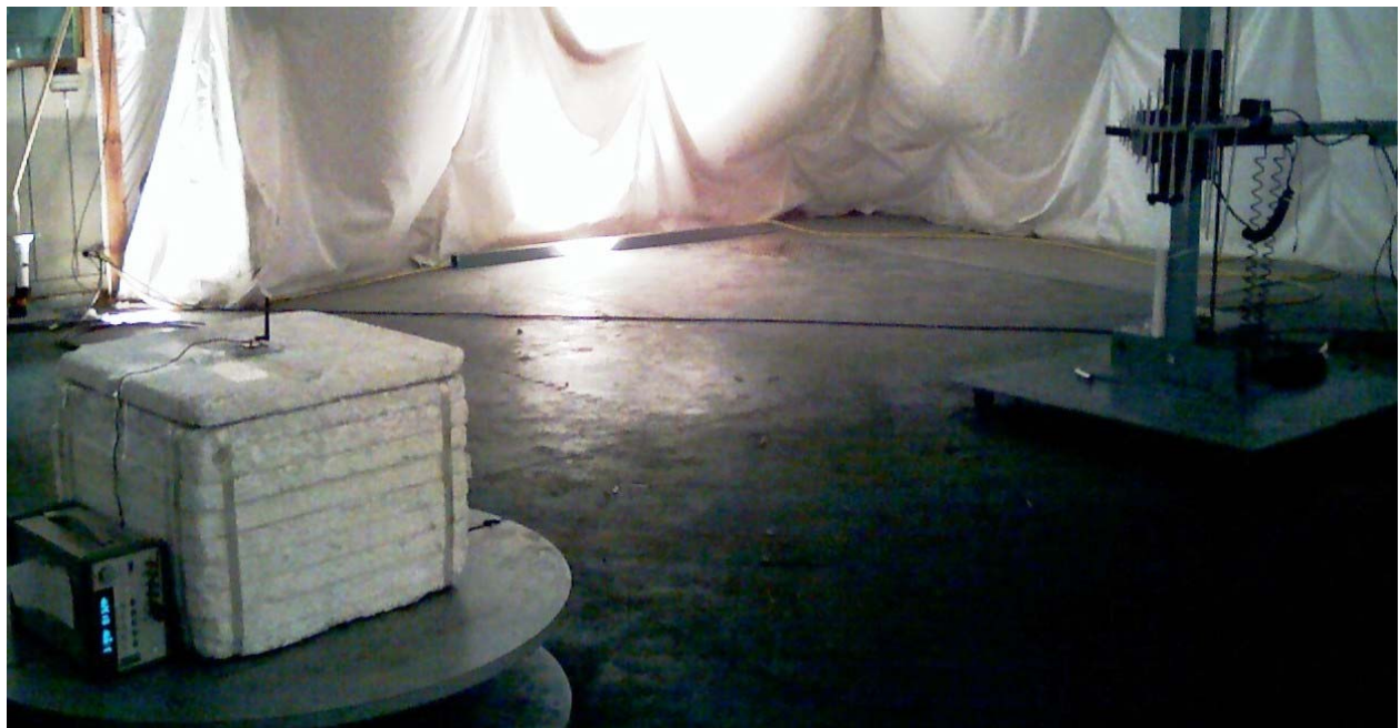
Photo 10: Test setup for radiated spurious between 200MHz and 2GHz with EMCO 3148 Log Periodic in vertical orientation shown and Alektrona AIM4M1 Module using 2dBi whip in vertical orientation
