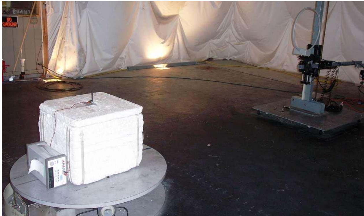
Photo 2: Test setup for radiated spurious between 9kHz and 30MHz with EMCO 6502 Loop Antenna shown and Alektrona AIM4M1 Module using 2dBi whip in vertical orientation
