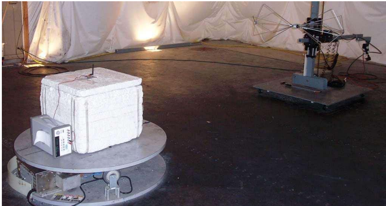
Photo 6: Test Setup for Radiated Spurious measurements between 30MHz and 300MHz using EMCO 3110B Biconical antenna in horizontal orientation and Alektrona AIM4M1 Module using 2dBi whip in vertical orientation
