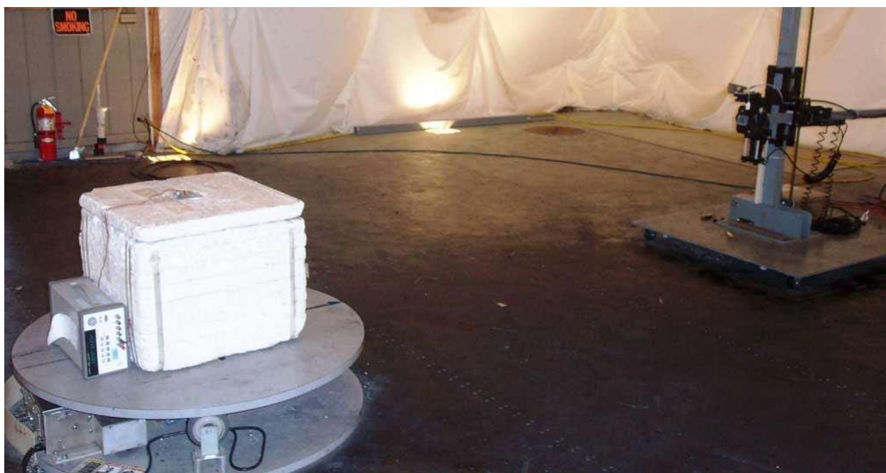
Photo 20: Test setup for radiated spurious emissions above 18GHz with AH Systems SAS-572 horn antenna in horizontal polarity and Alektrona AIM4M1 Module using on board F antenna
