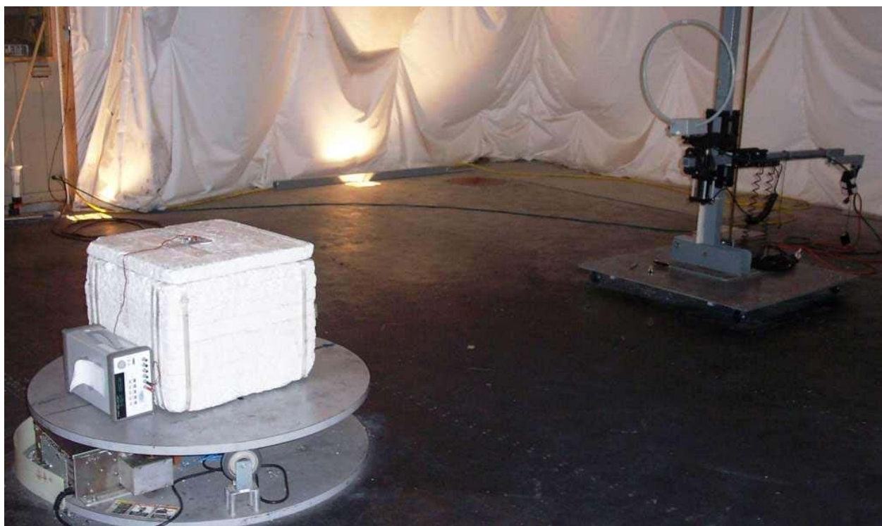
Photo 3: Test setup for radiated spurious between 9kHz and 30MHz with EMCO 6502 Loop Antenna with Alektrona AIM4M1 Module using on board F antenna
