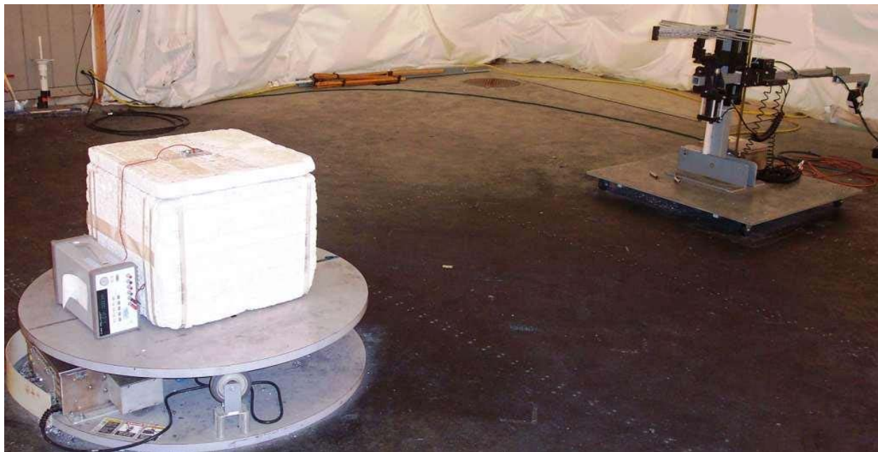
Photo 9: Test setup for radiated spurious between 200MHz and 2GHz with EMCO 3148 Log Periodic in horizontal orientation and Alektrona AIM4M1 Module using F antenna
