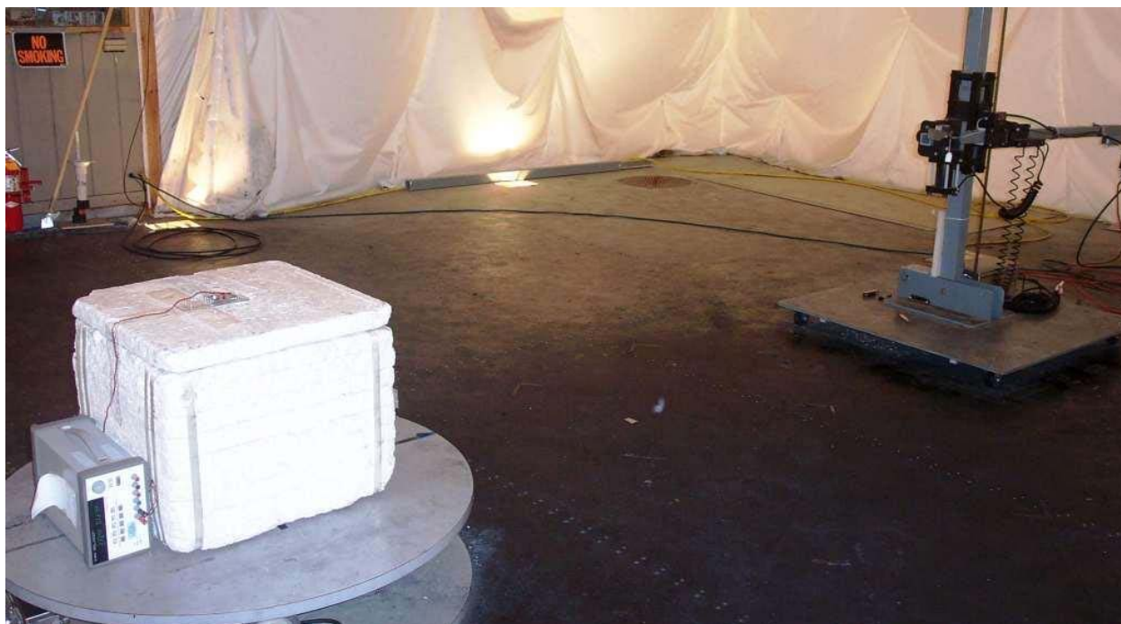
Photo 19: Test setup for radiated spurious emissions above 18GHz with AH Systems SAS-572 horn antenna in vertical polarity and Alektrona AIM4M1 Module using on board F antenna
