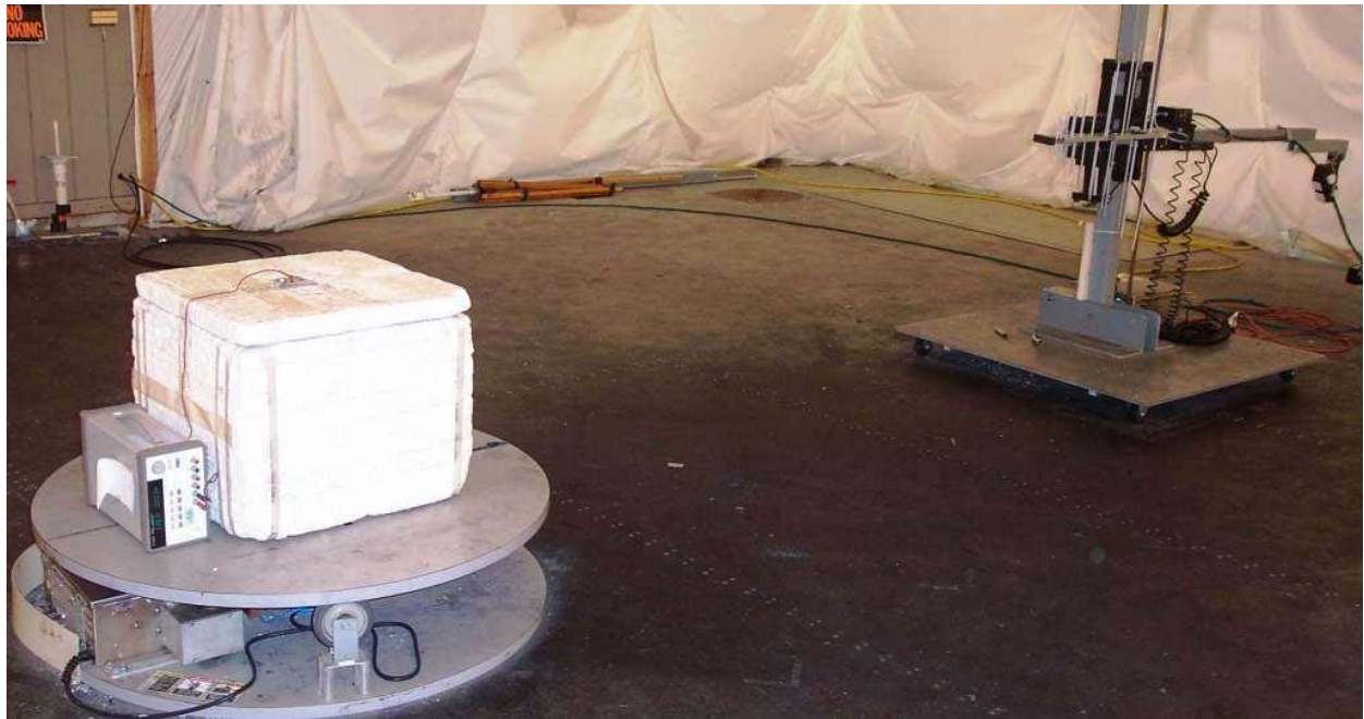
Photo 10: Test setup for radiated spurious between 200MHz and 2GHz with EMCO 3148 Log Periodic in vertical orientation and Alektrona AIM4M1 Module using F antenna
