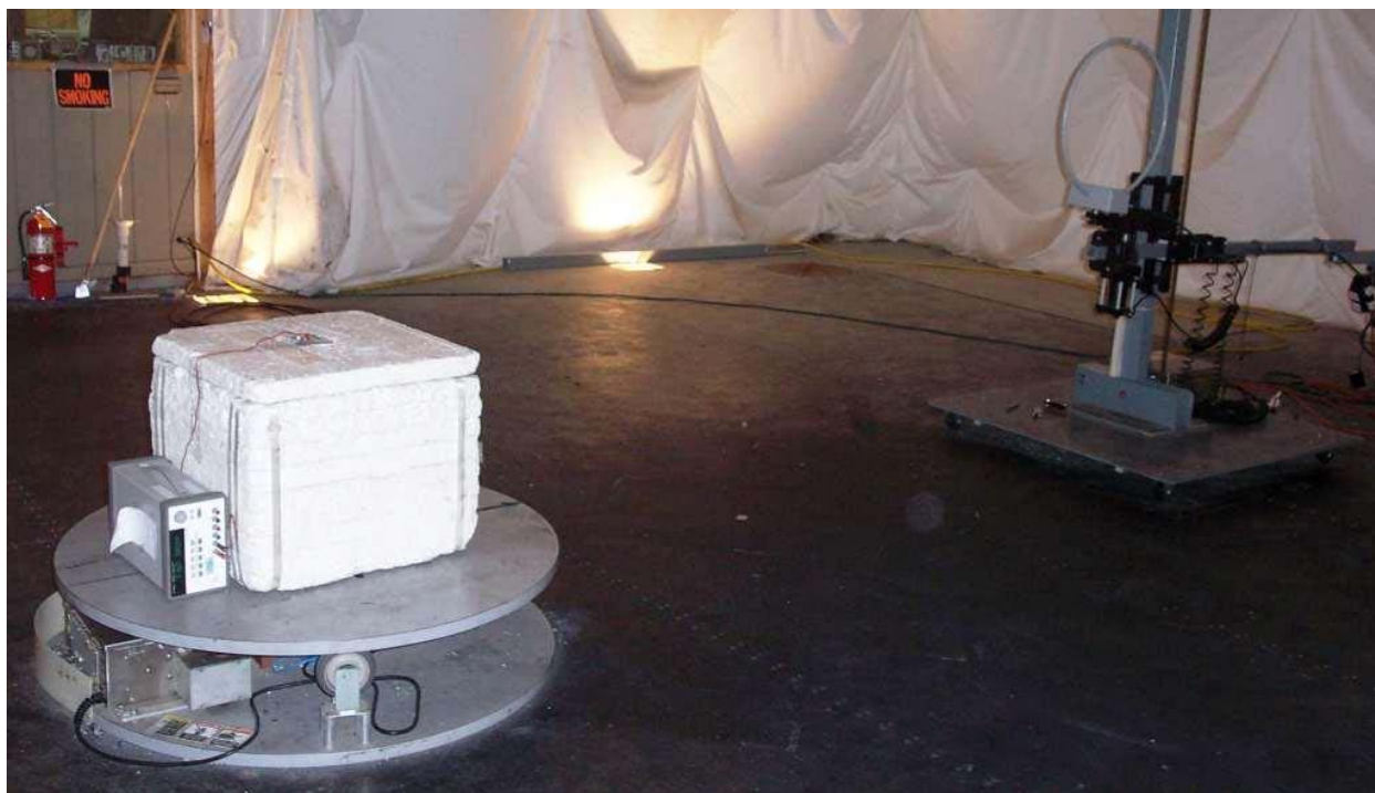
Photo 2: Test setup for radiated spurious between 9kHz and 30MHz with EMCO 6502 Loop Antenna with Alektrona AIM4M1 Module using on board F antenna
