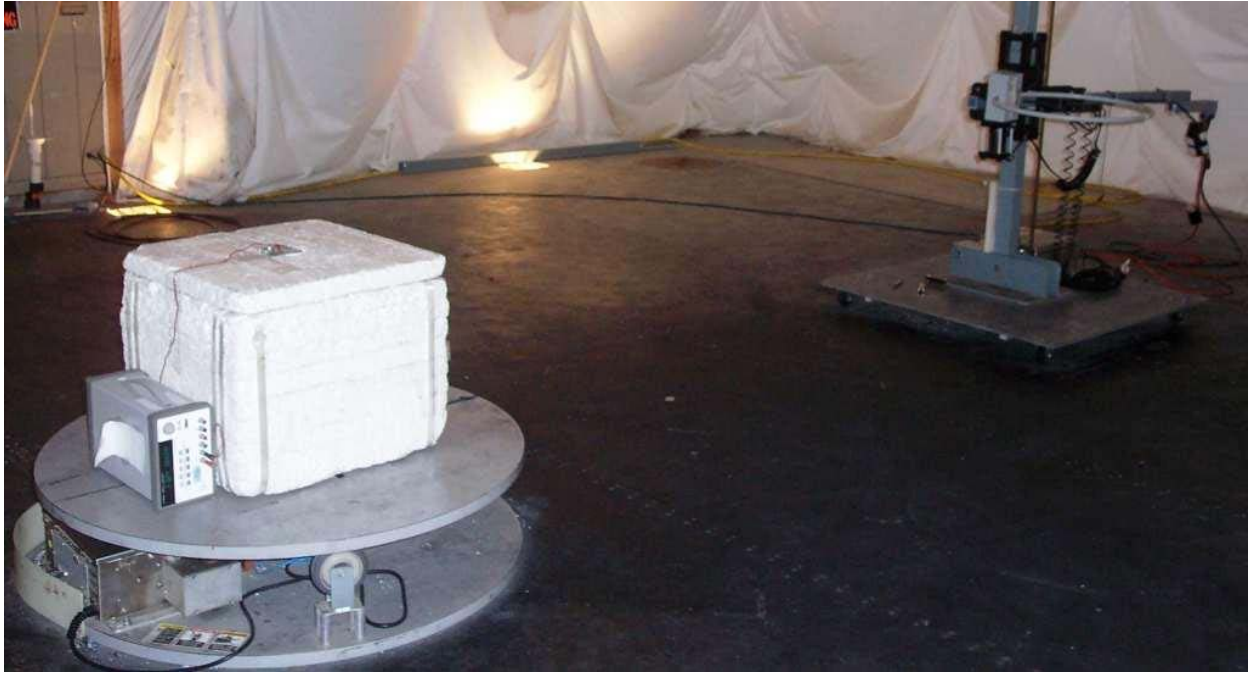
Photo 1: Test setup for radiated spurious between 9kHz and 30MHz with EMCO 6502 Loop Antenna with Alektrona AIM4M1 Module using on board F antenna
