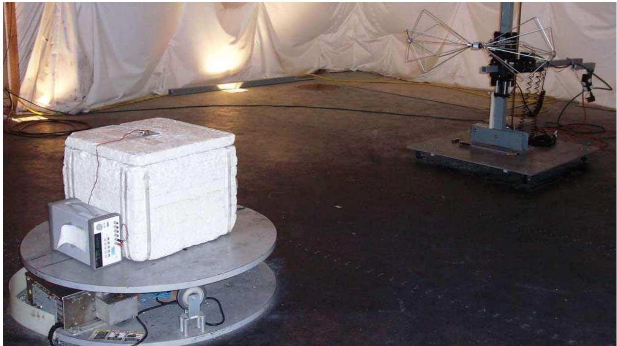
Photo 6: Test Setup for Radiated Spurious measurements between 30MHz and 300MHz using EMCO 3110B Biconical antenna in horizontal orientation and Alektrona AIM4M1 Module using on board F antenna
