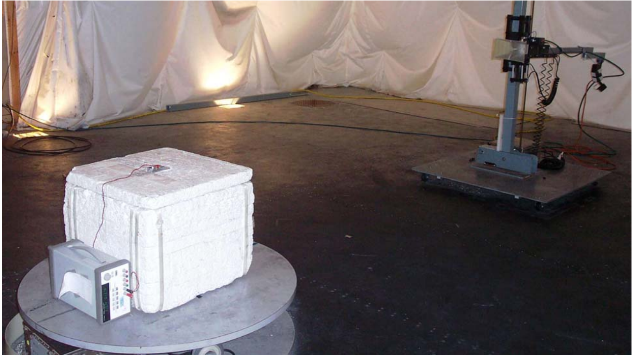
Photo 15: Test setup for radiated spurious emissions below 18GHz with EMCO 3115 horn antenna in vertical polarity and Alektrona AIM4M1 Module using on board F antenna
