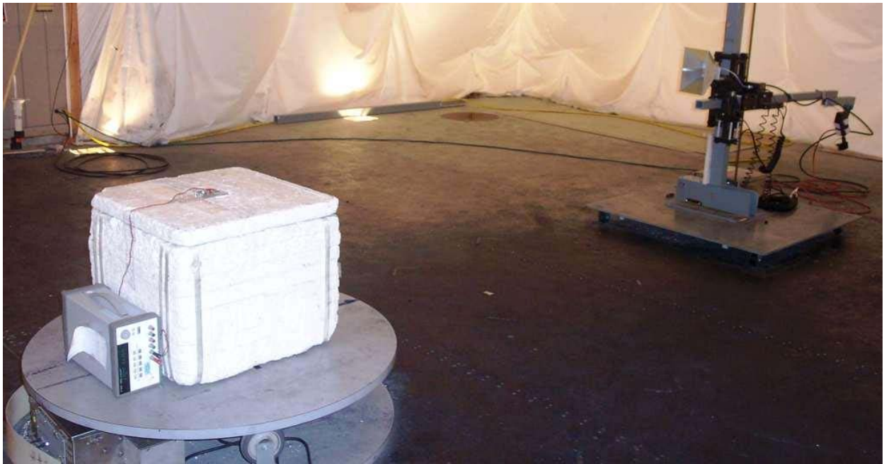
Photo 16: Test setup for radiated spurious emissions below 18GHz with EMCO 3115 horn antenna in horizontal polarity and Alektrona AIM4M1 Module using on board F antenna
