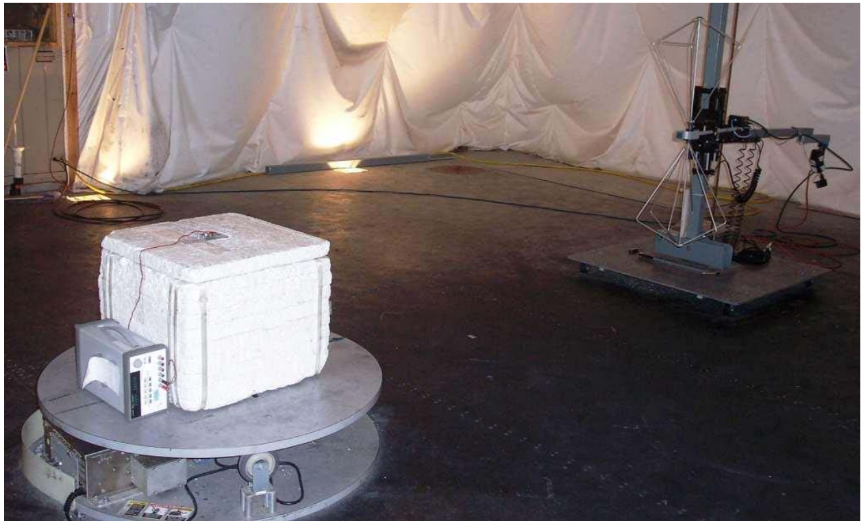
Photo 5: Test Setup for Radiated Spurious measurements between 30MHz and 300MHz using EMCO 3110B Biconical antenna in vertical orientation and Alektrona AIM4M1 Module using on board F antenna
