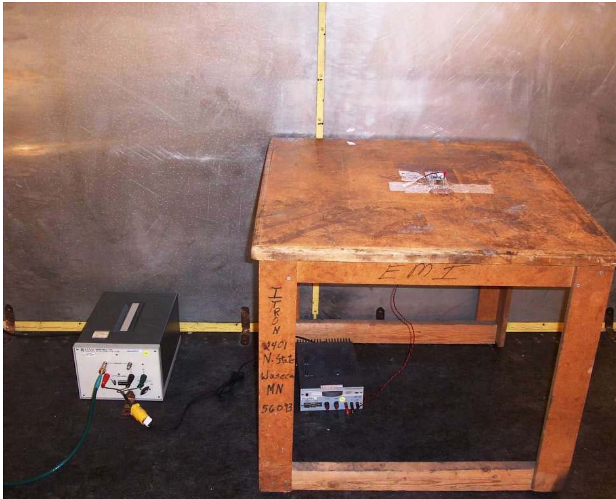
Photo 23: AC line conducted measurement with F antenna
