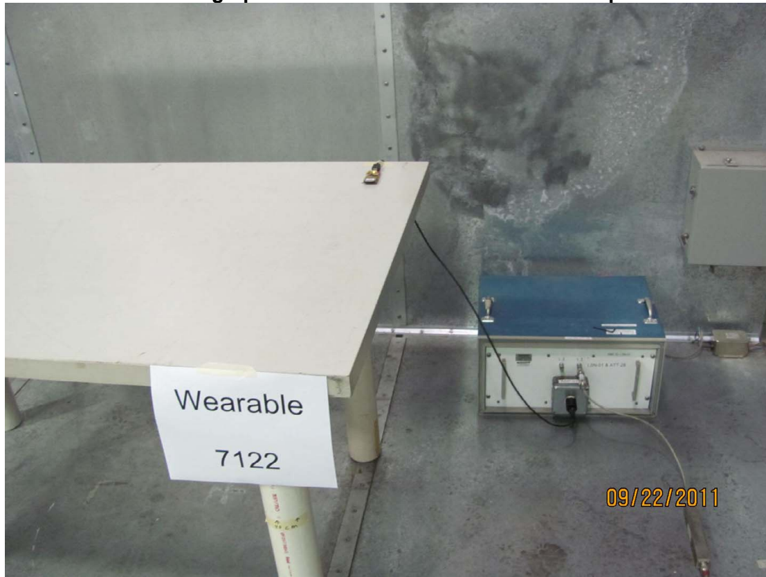
Photograph of Conducted Emissions Test Setup
