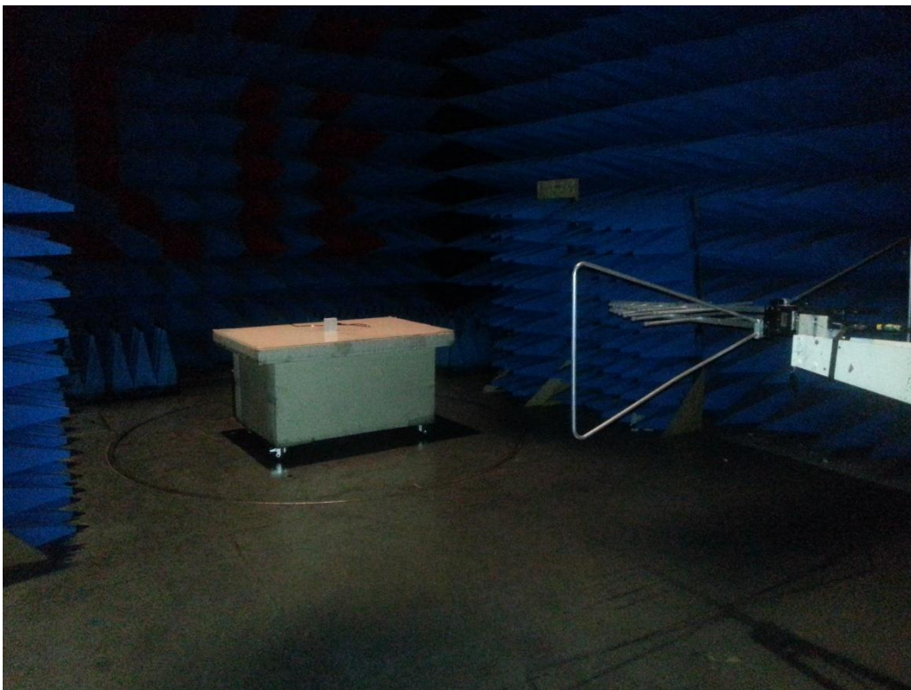
Radiated emissions measurements setup below 1GHz
