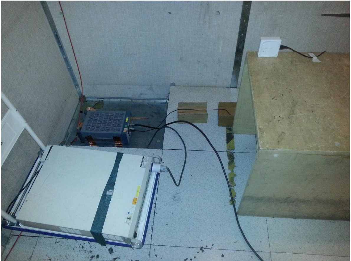
Conducted emission measurement setup
