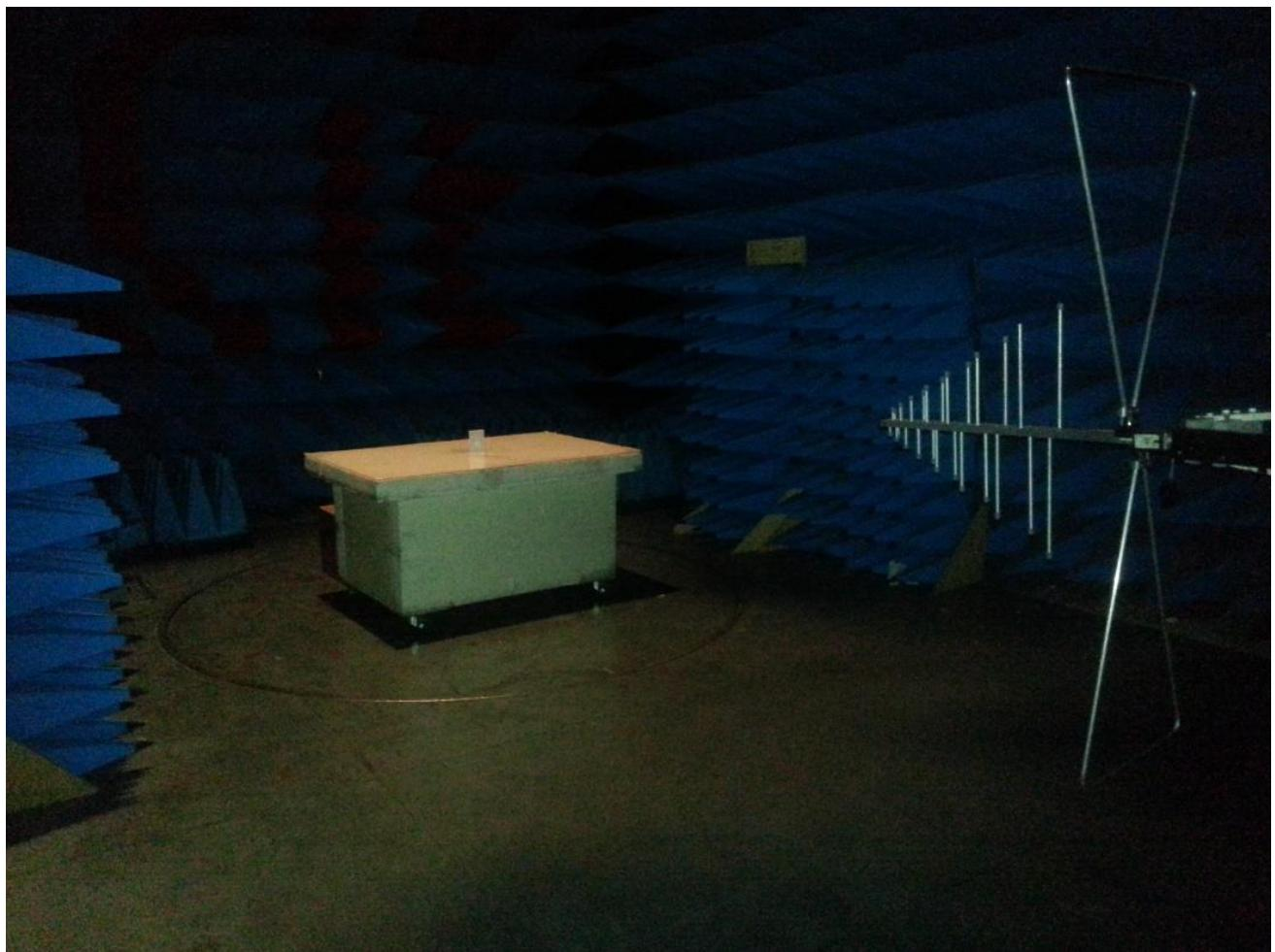
Radiated emissions measurements setup
