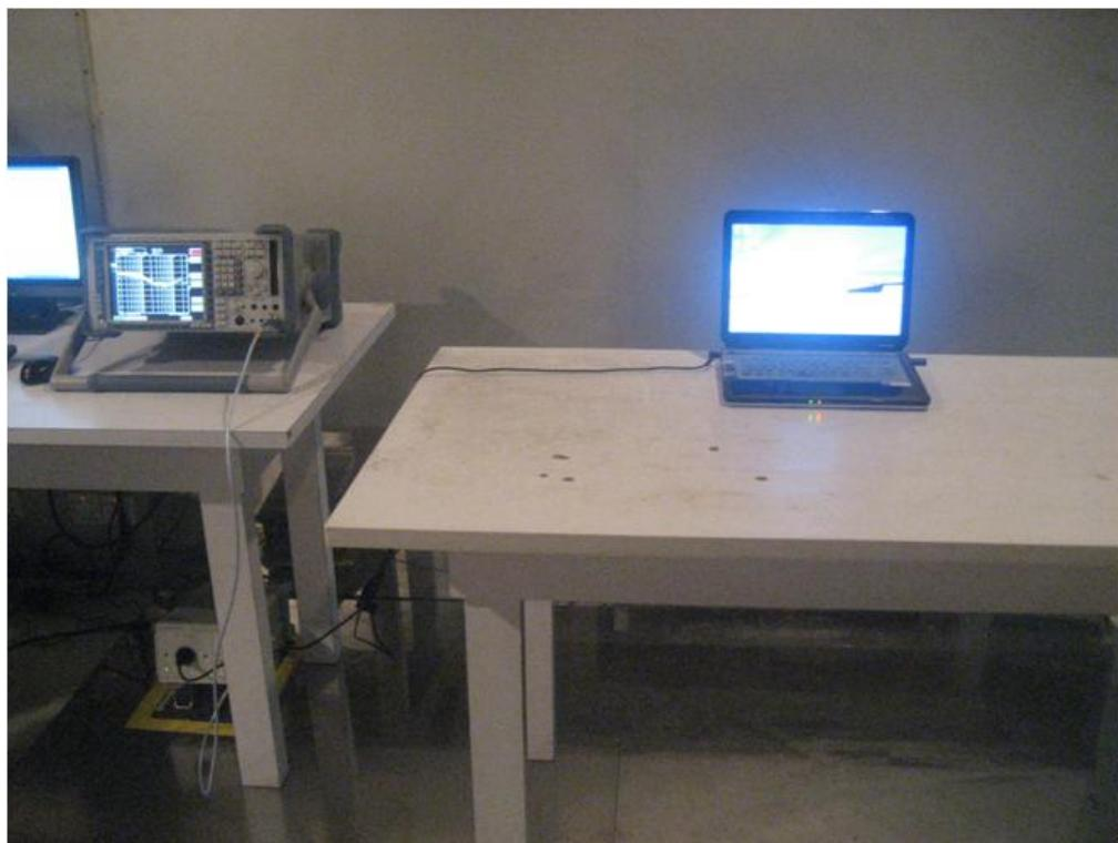
**TEST SETUP OF RADIATED EMISSION (9kHz-30MHz)**
