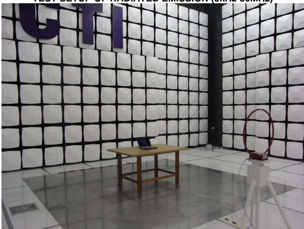
**TEST SETUP OF RADIATED EMISSION (30MHz-1GHz)**
