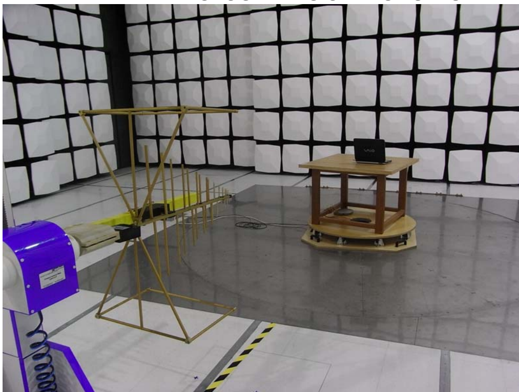
TEST SETUP OF RADIATED EMISSION (30MHz-1GHz)
