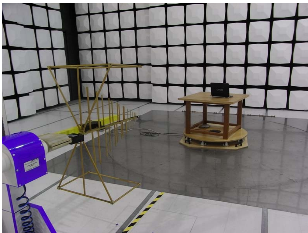
TEST SETUP OF RADIATED EMISSION (30MHz-1GHz)
