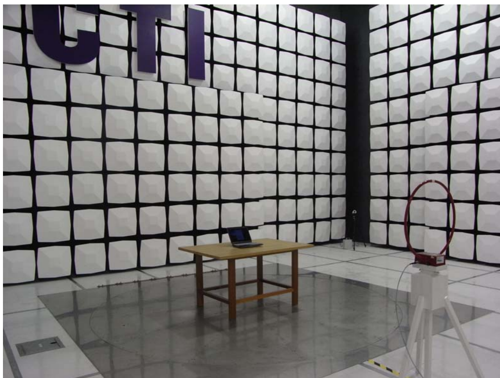
TEST SETUP OF RADIATED EMISSION (9kHz-30MHz)
