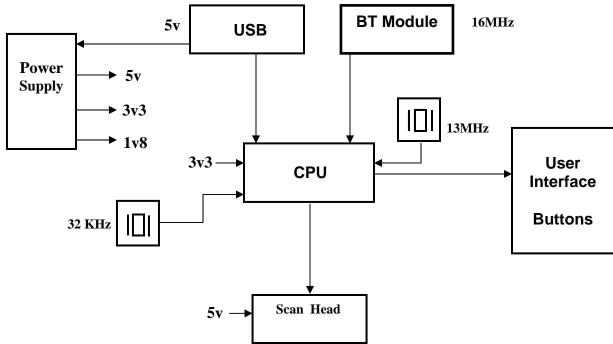
Pressing the scanner buttons will set the resolution and color mode. Next roll scanner device over 8 X 11 1/2 document. Scan head is reading light reflected from the paper. Data from the scan head is then saved onto the internal memory. Connect the scanner device through the USB cable to the PC. Open the scanner software and data is able to transfer to PC from scanner device, through USB cable.
