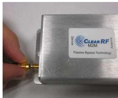
2. Connect the SMA end of the SMA-to-SMA device cable to the Cellular Modem or MDT antenna connection.
