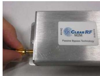
2. Connect the MMCX end of the SMA to MMCX device cable to the Cellular Module.
