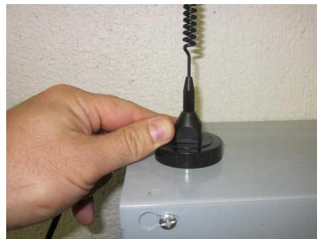
4. Connect the Outdoor Signal Antenna connector to the ClearRF amplifier SMA connector marked "Antenna".
