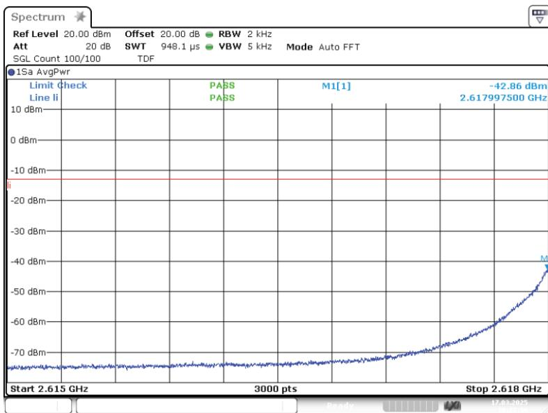
Band: BRS UBS; Frequency: 2.6180 GHz to 2.6900 GHz; Band edge: lower; Mod: GSM; Input power = 3 dB > AGC; Number of signals 2
