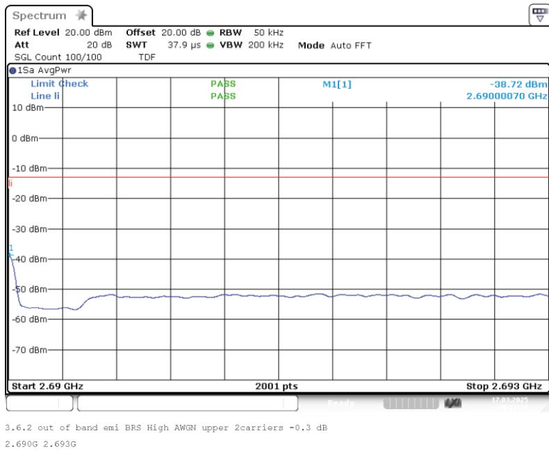
Band: BRS UBS; Frequency: 2.6180 GHz to 2.6900 GHz; Band edge: upper; Mod: AWGN;
