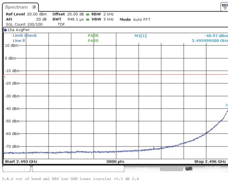
Band: BRS LBS; Frequency: 2.4960 GHz to 2.5680 GHz; Band edge: lower; Mod: GSM; Input power = 3 dB > AGC; Number of signals 1
