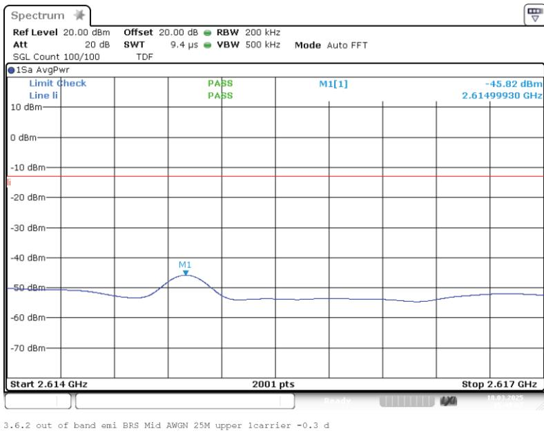
Band: BRS MBS; Frequency: 2.5720 GHz to 2.6140 GHz; Band edge: upper; Mod: AWGN 25M;
