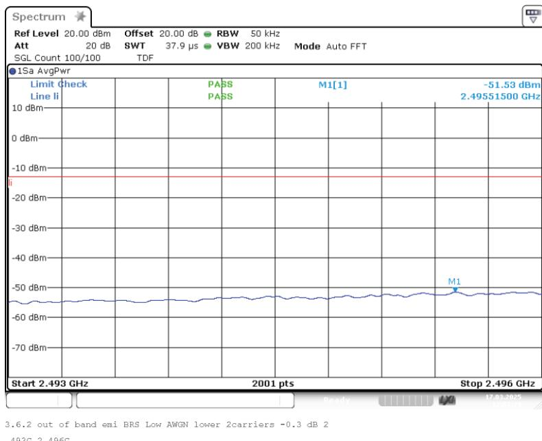
Band: BRS LBS; Frequency: 2.4960 GHz to 2.5680 GHz; Band edge: lower; Mod: AWGN; Input power = 3 dB > AGC; Number of signals 2
