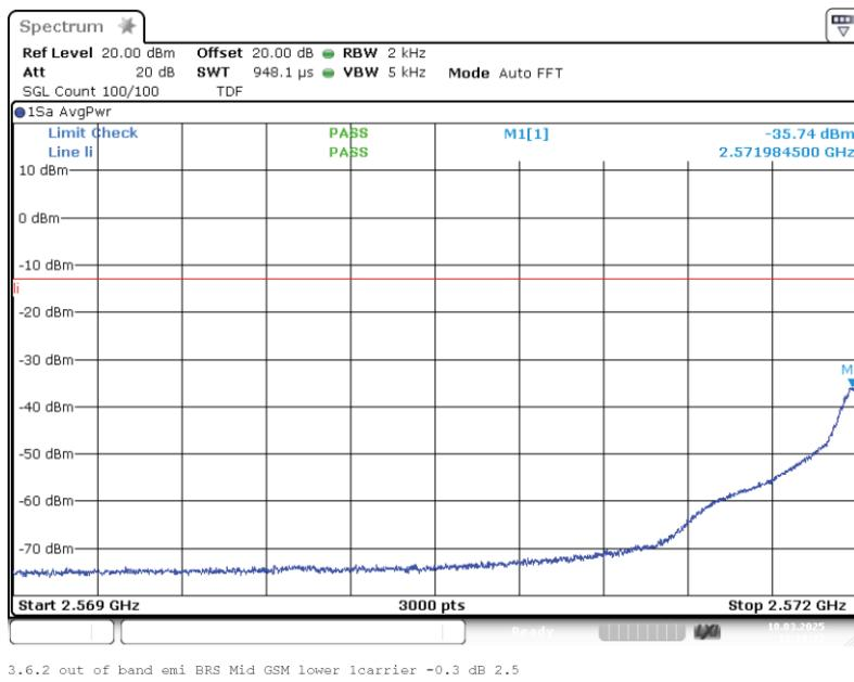
Band: BRS MBS; Frequency: 2.5720 GHz to 2.6140 GHz; Band edge: lower; Mod: GSM; Input power = 3 dB > AGC; Number of signals 1
