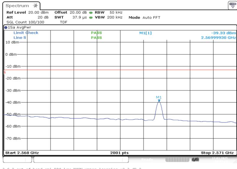
Band: BRS LBS; Frequency: 2.4960 GHz to 2.5680 GHz; Band edge: upper; Mod: AWGN;
