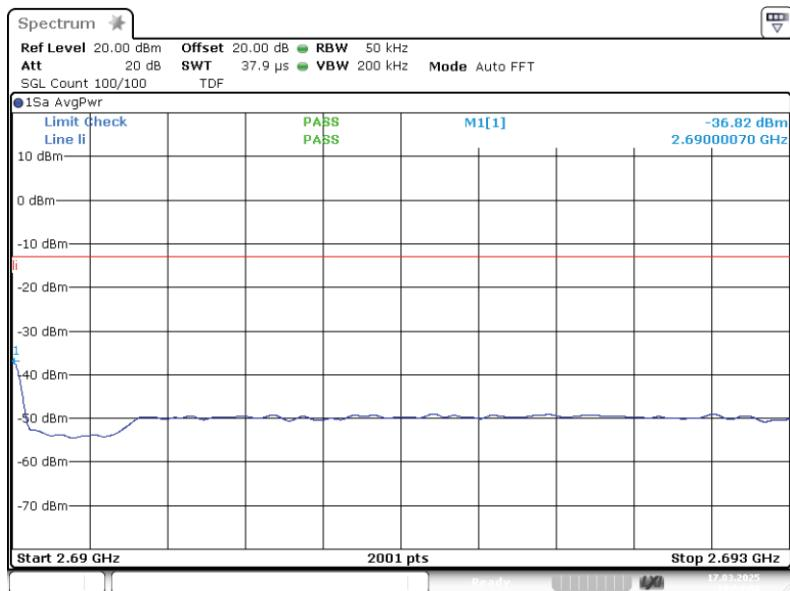
3.6.2 out of band emi BRS High AWGN upper 1carrier -0.3 dB 2
