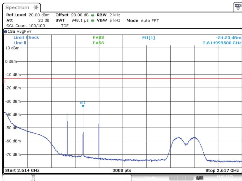
Band: BRS MBS; Frequency: 2.5720 GHz to 2.6140 GHz; Band edge: upper; Mod: GSM; Input power = 3 dB > AGC; Number of signals 2
