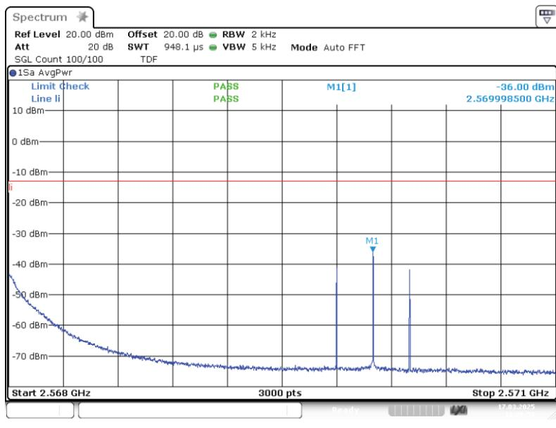
Band: BRS LBS; Frequency: 2.4960 GHz to 2.5680 GHz; Band edge: upper; Mod: GSM; Input power = 3 dB > AGC; Number of signals 2
