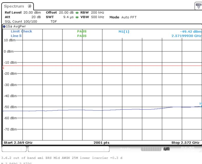
Band: BRS MBS; Frequency: 2.5720 GHz to 2.6140 GHz; Band edge: lower; Mod: AWGN 25M;
