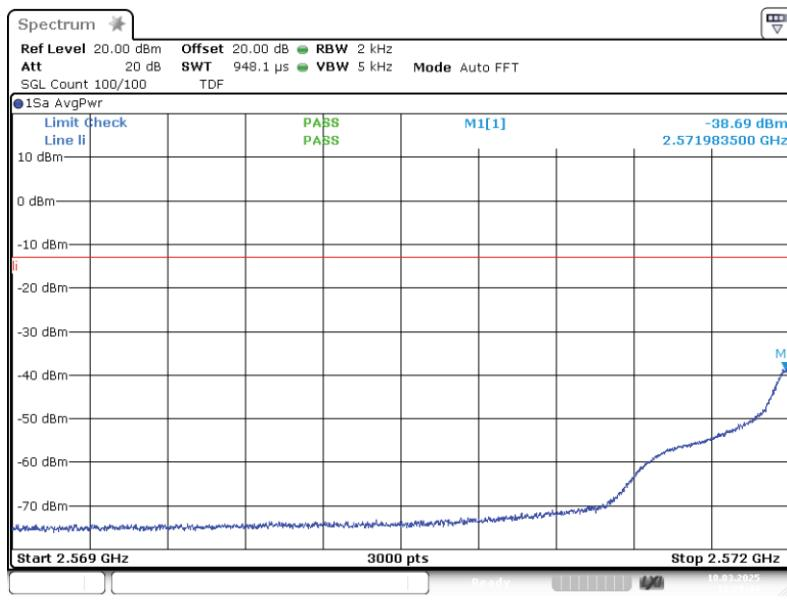
Band: BRS MBS; Frequency: 2.5720 GHz to 2.6140 GHz; Band edge: lower; Mod: GSM; Input power = 3 dB > AGC; Number of signals 2
