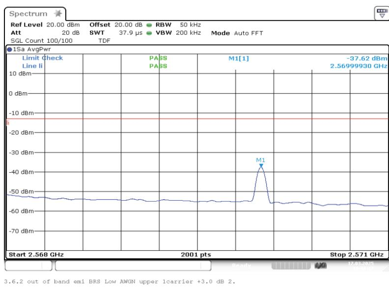
Band: BRS LBS; Frequency: 2.4960 GHz to 2.5680 GHz; Band edge: upper; Mod: AWGN 45M;
