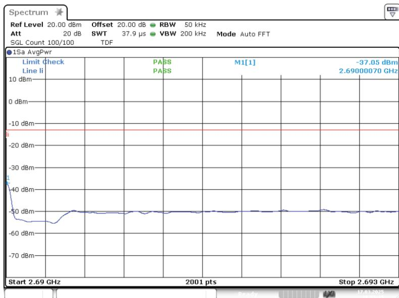
3.6.2 out of band emi BRS High AWGN upper 1carrier +3.0 dB 2
