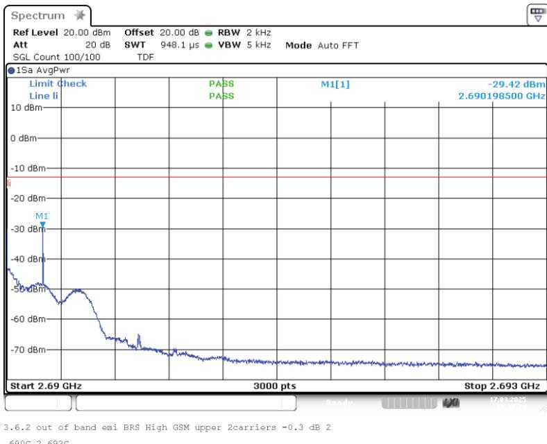
Band: BRS UBS; Frequency: 2.6180 GHz to 2.6900 GHz; Band edge: upper; Mod: GSM; Input power = 3 dB > AGC; Number of signals 2
