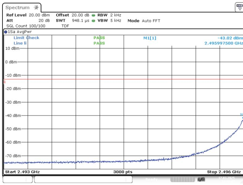
Band: BRS LBS; Frequency: 2.4960 GHz to 2.5680 GHz; Band edge: lower; Mod: GSM; Input power = 3 dB > AGC; Number of signals 2
