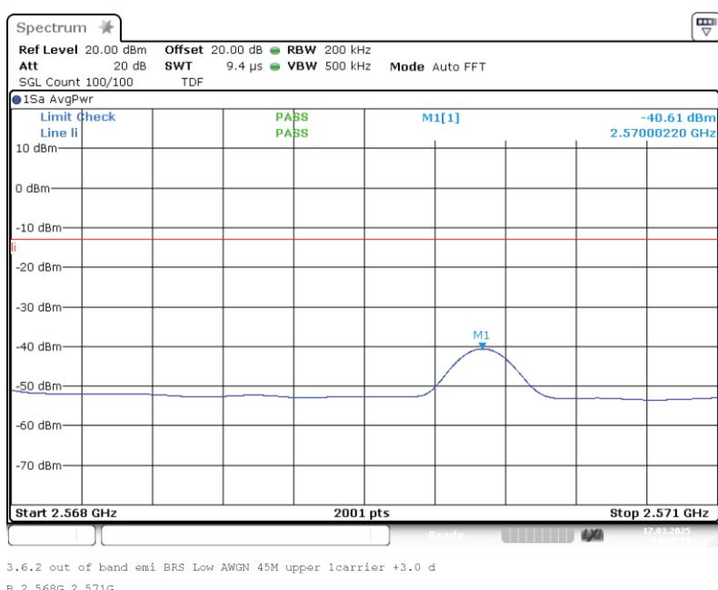
Band: BRS LBS; Frequency: 2.4960 GHz to 2.5680 GHz; Band edge: upper; Mod: GSM; Input power = 0.3 dB < AGC; Number of signals 1
