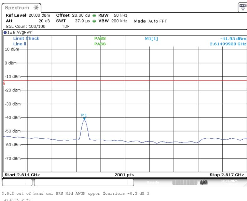
Band: BRS MBS; Frequency: 2.5720 GHz to 2.6140 GHz; Band edge: upper; Mod: AWGN;
