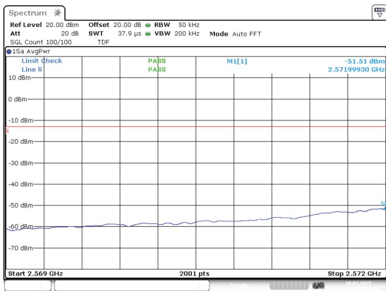
3.6.2 out of band emi BRS Mid AWGN lower lcarrier +3.0 dB 2.
