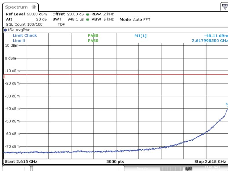
Band: BRS UBS; Frequency: 2.6180 GHz to 2.6900 GHz; Band edge: lower; Mod: GSM; Input power = 3 dB > AGC; Number of signals 1
