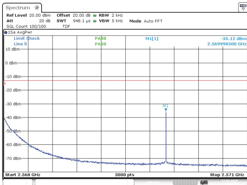
Band: BRS LBS; Frequency: 2.4960 GHz to 2.5680 GHz; Band edge: upper; Mod: GSM; Input power = 3 dB > AGC; Number of signals 1
