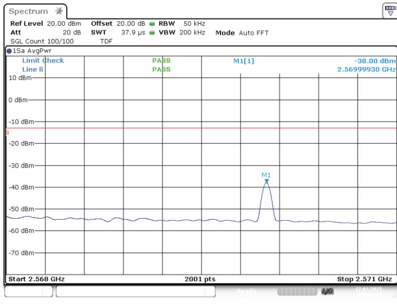
Band: BRS LBS; Frequency: 2.4960 GHz to 2.5680 GHz; Band edge: upper; Mod: AWGN;
