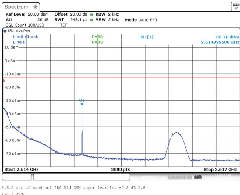
Band: BRS MBS; Frequency: 2.5720 GHz to 2.6140 GHz; Band edge: upper; Mod: GSM; Input power = 3 dB > AGC; Number of signals 1
