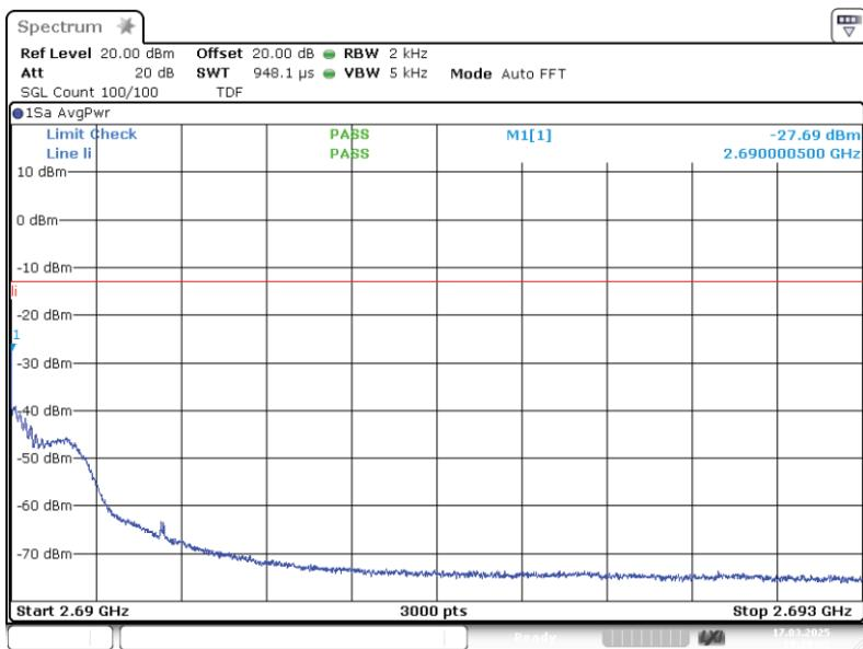
Band: BRS UBS; Frequency: 2.6180 GHz to 2.6900 GHz; Band edge: upper; Mod: GSM; Input power = 3 dB > AGC; Number of signals 1
