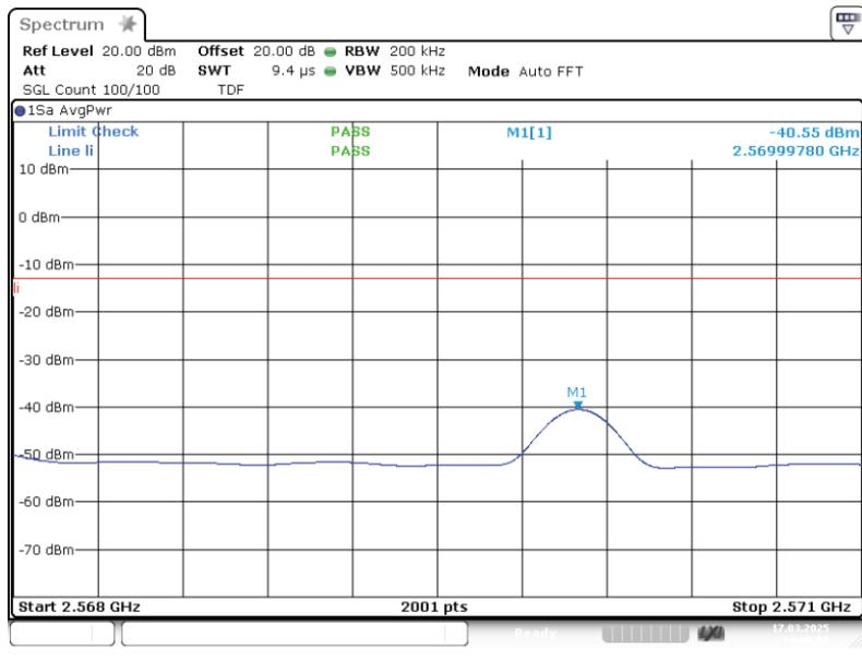
Band: BRS LBS; Frequency: 2.4960 GHz to 2.5680 GHz; Band edge: upper; Mod: AWGN 45M;
