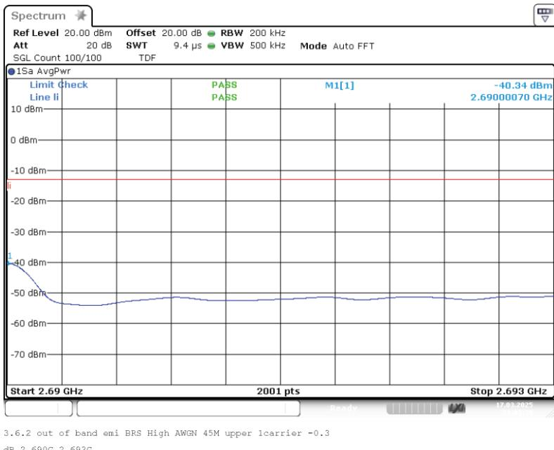
Band: BRS UBS; Frequency: 2.6180 GHz to 2.6900 GHz; Band edge: upper; Mod: AWGN 45M;
