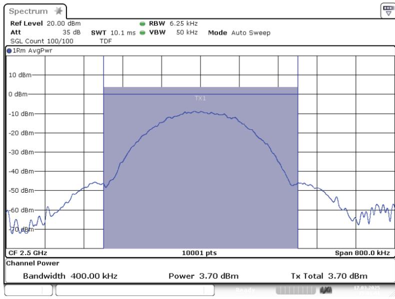
Band: BRS LBS; Frequency: 2.5000 GHz; Band edge: f0; Mod: GSM;
