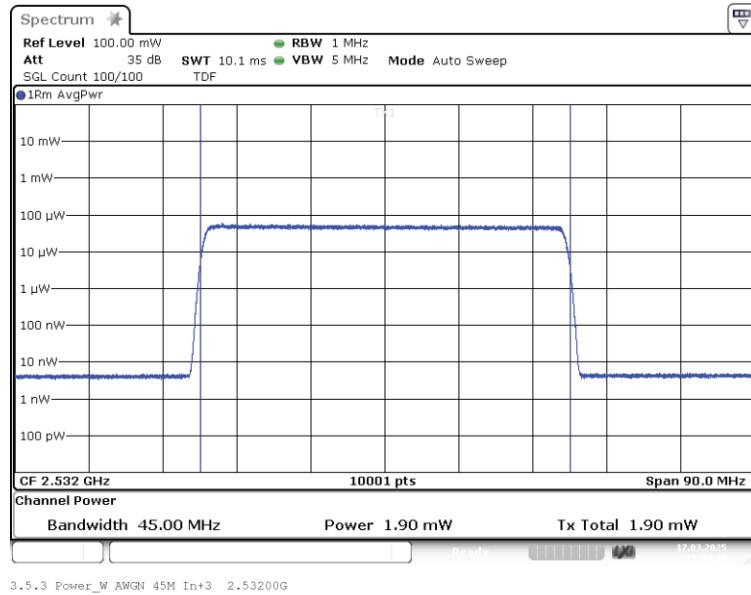
Band: BRS LBS; Frequency: 2.5320 GHz; Band edge: mid; Mod: AWGN 45M;
