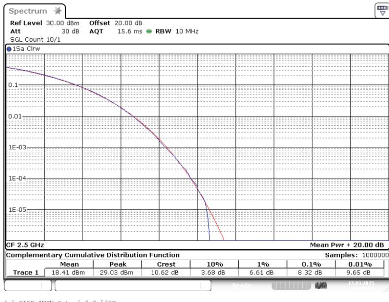
Band: BRS LBS; Frequency: 2,5000 GHz; Band edge: f0; Mod: AWGN; PAPR 3 dB > AGC
