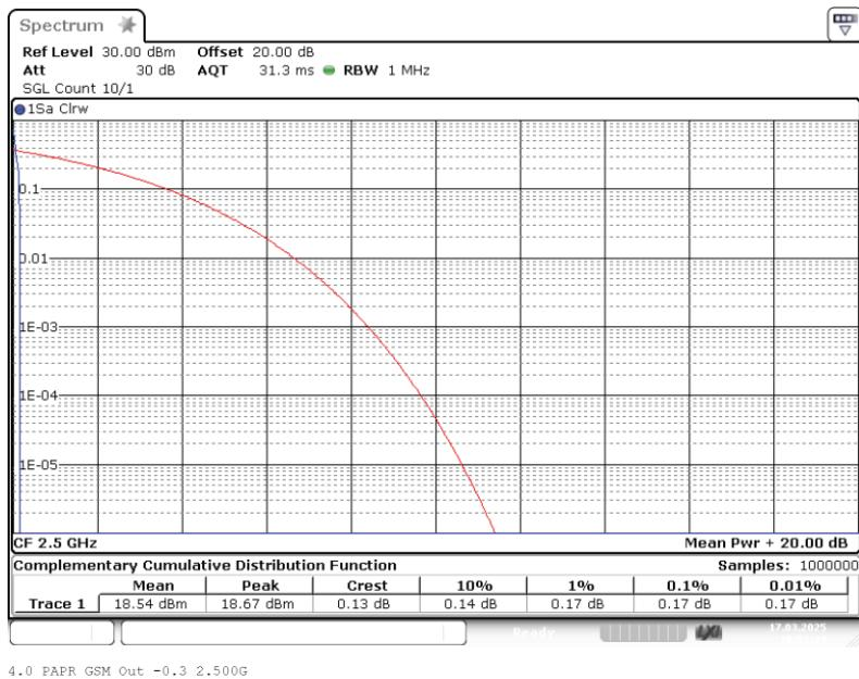
Band: BRS LBS; Frequency: 2,5000 GHz; Band edge: f0; Mod: GSM; PAPR 3 dB &gt; AGC
