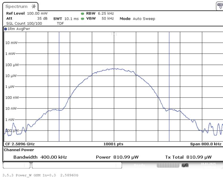
Band: BRS MBS; Frequency: 2.5896 GHz; Band edge: f0; Mod: GSM;
