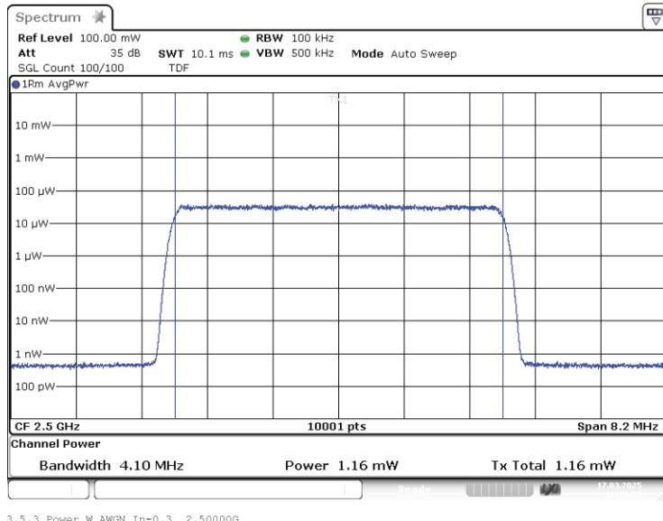
Band: BRS LBS; Frequency: 2.5000 GHz; Band edge: f0; Mod: AWGN;
