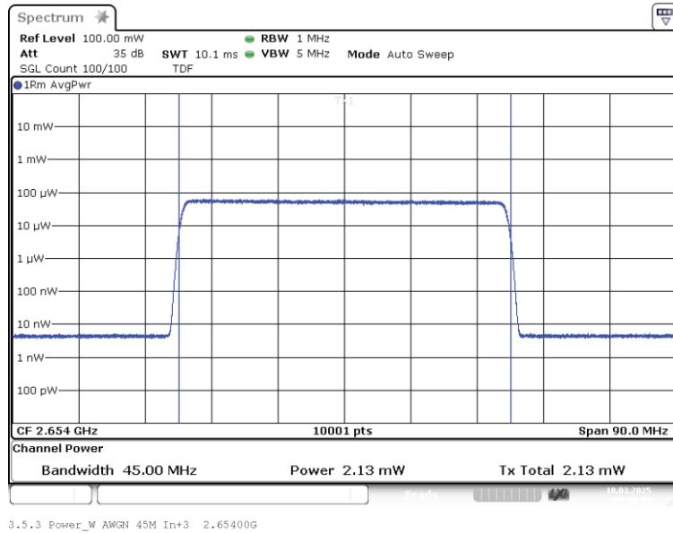
Band: BRS UBS; Frequency: 2.6540 GHz; Band edge: mid; Mod: AWGN 45M;
