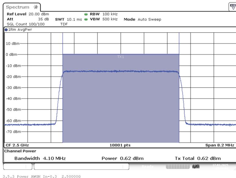
Band: BRS LBS; Frequency: 2.5000 GHz; Band edge: f0; Mod: AWGN;
