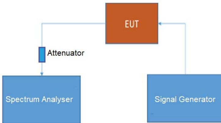
The attenuation of the measuring and stimulus path are known for each measured frequency and are considered.
