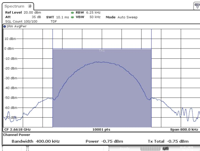
Band: BRS UBS; Frequency: 2.6618 GHz; Band edge: f0; Mod: GSM;
