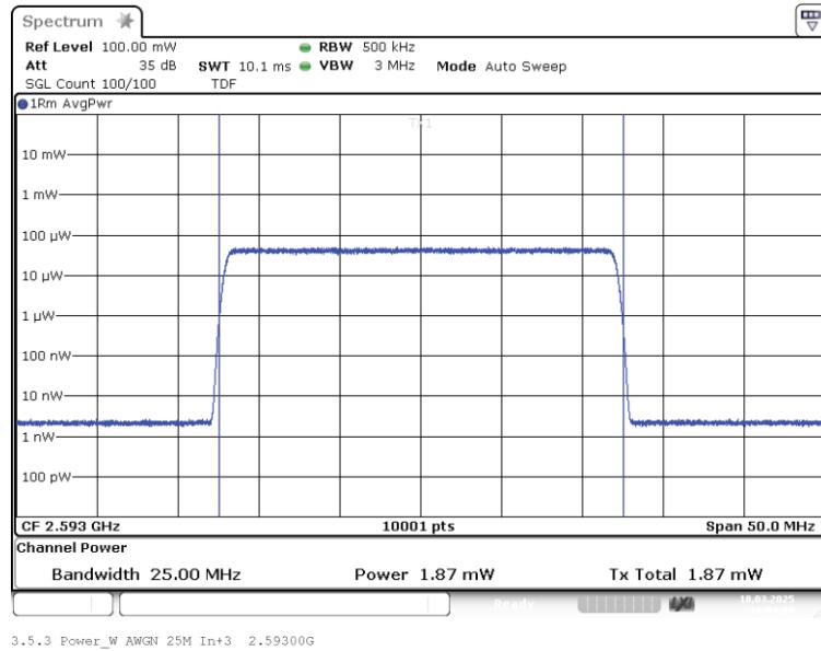
Band: BRS MBS; Frequency: 2.5930 GHz; Band edge: mid; Mod: AWGN 25M;
