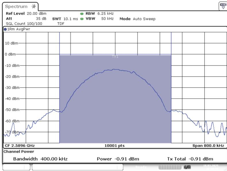
Band: BRS MBS; Frequency: 2.5896 GHz; Band edge: f0; Mod: GSM;
