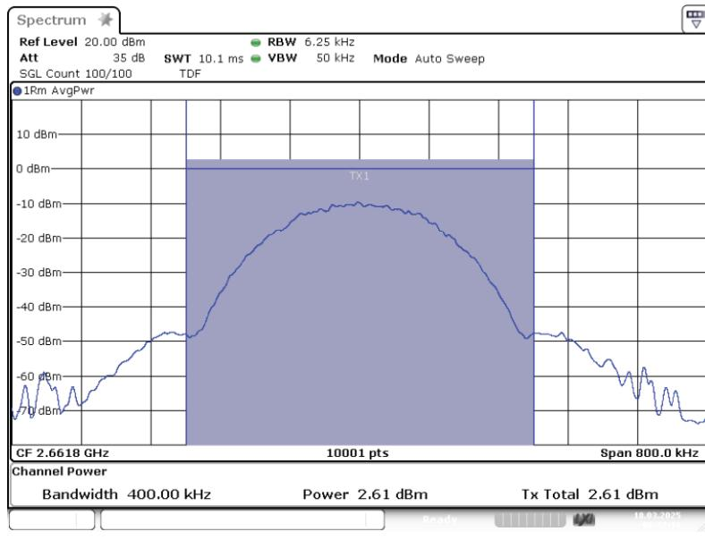
Band: BRS UBS; Frequency: 2.6618 GHz; Band edge: f0; Mod: GSM;
