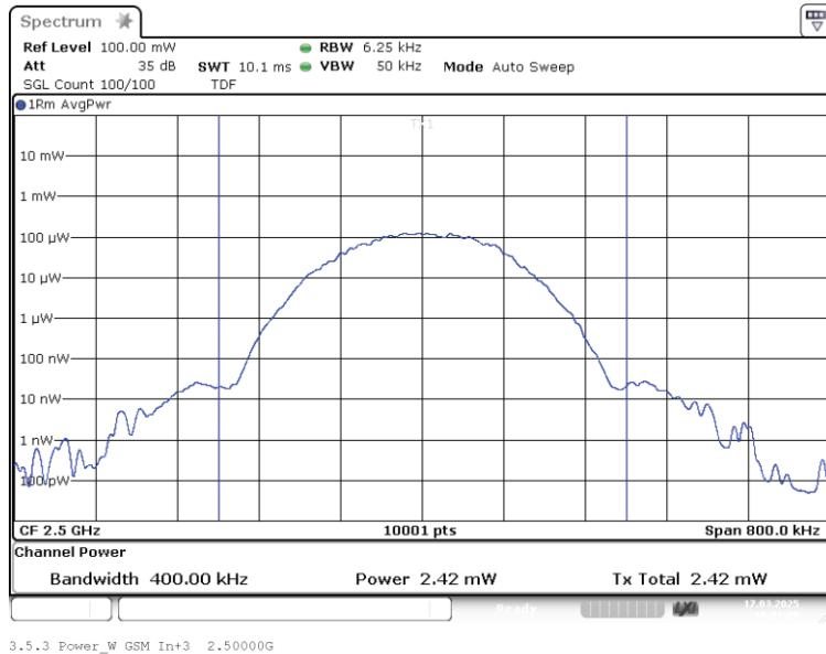
Band: BRS LBS; Frequency: 2.5000 GHz; Band edge: f0; Mod: GSM;
