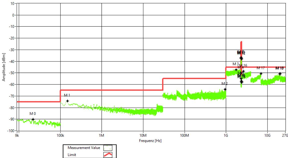
Frequency Band = WCS 2300; Test frequency = mid; Direction = RF downlink;
