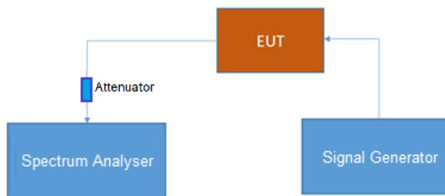
Test Setup step 2; Occupied Bandwidth/Input-versus-output spectrum
