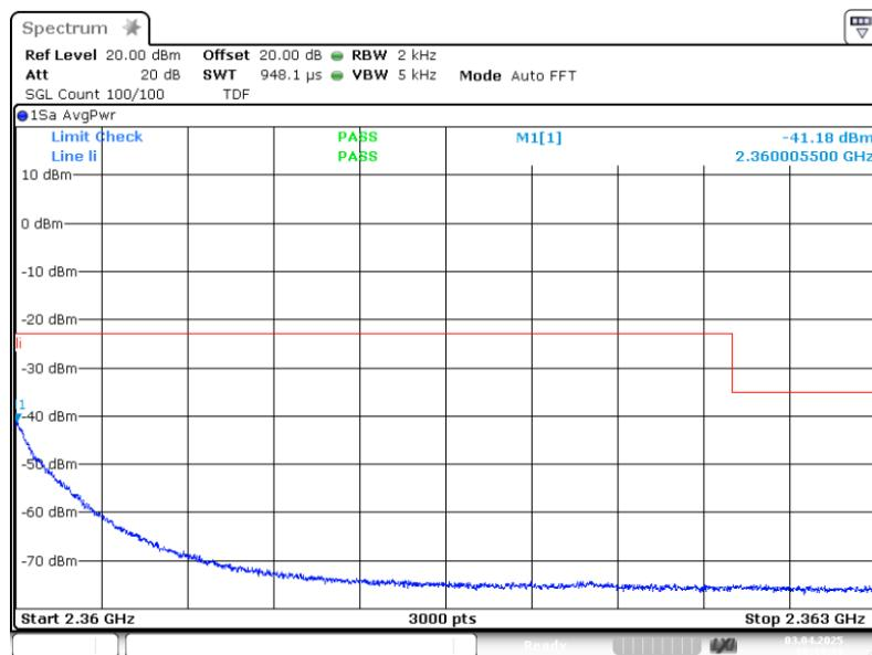
3.6.2 out of band emi WCS 2300 GSM upper lcarrier +3.0 dB 2.
