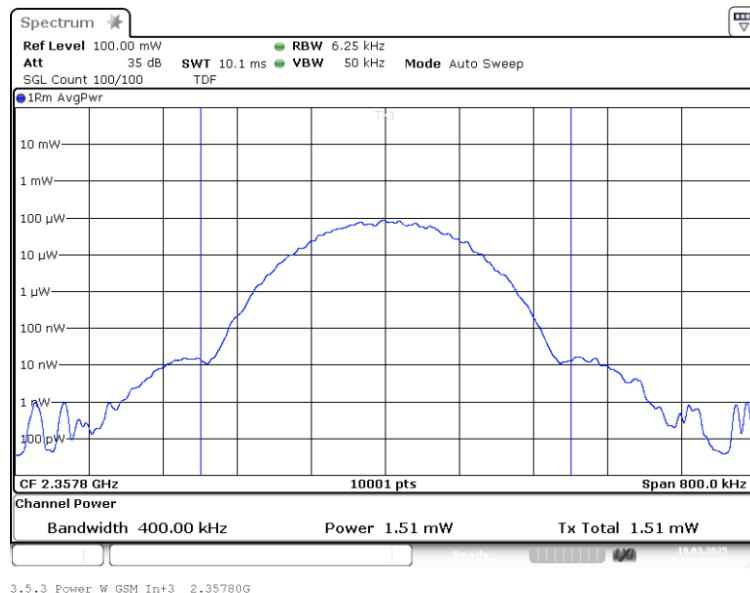
Band: WCS 2300; Frequency: 2.3578 GHz; Band edge: f0; Mod: GSM;
