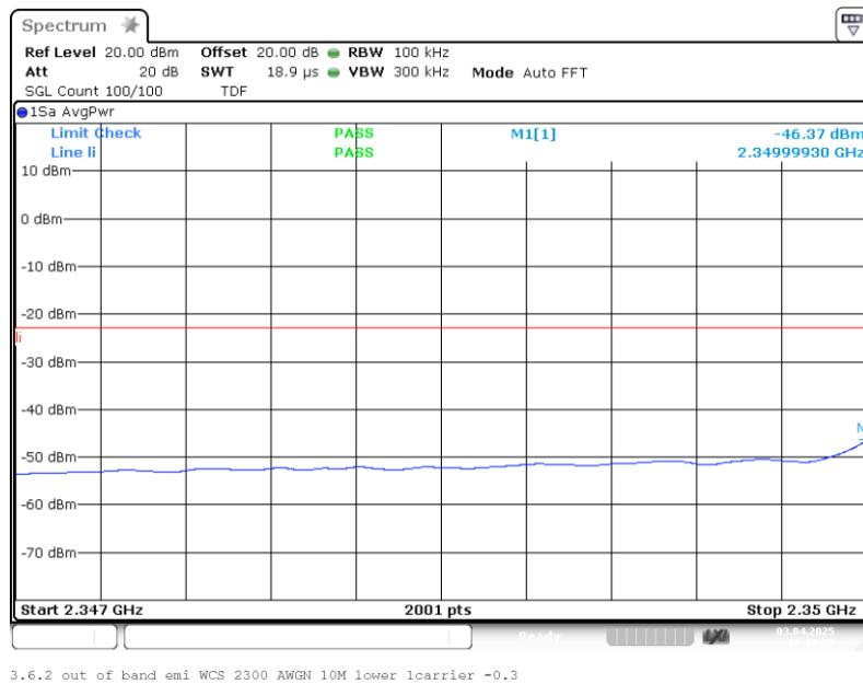
Band: WCS 2300; Frequency: 2,3500 GHz to 2,3600 GHz; Band edge: lower; Mod: AWGN 10M; Input power = 3 dB > AGC; Number of signals 1
