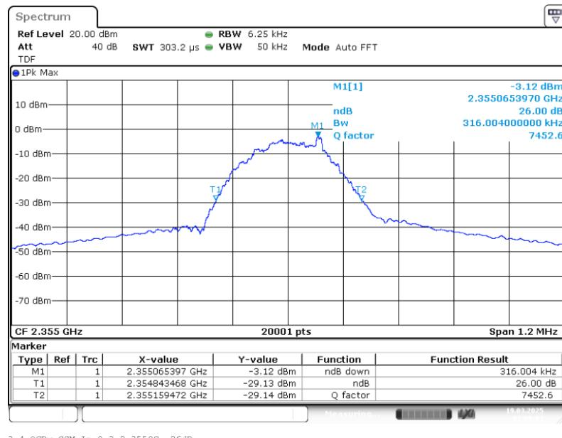
Band: WCS 2300; Frequency: 2.3550 GHz; Band edge: mid; Mod: GSM;
