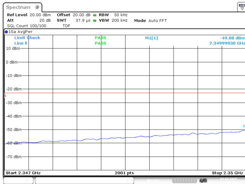
3.6.2 out of band emi WCS 2300 AWGN lower lcarrier -0.3 dB 2
