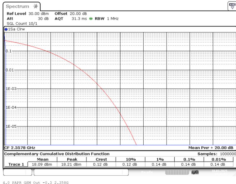
Band: WCS 2300; Frequency: 2.3578 GHz; Band edge: f0; Mod: GSM; PAPR 3 dB > AGC
