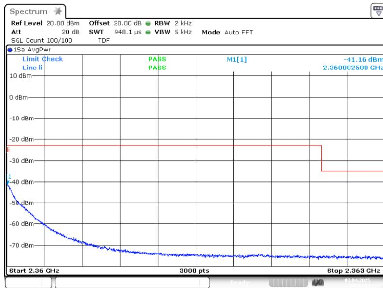
3.6.2 out of band emi WCS 2300 GSM upper lcarrier -0.3 dB 2.
