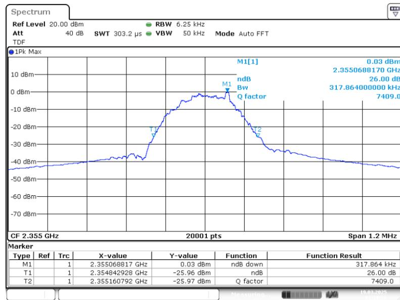
Band: WCS 2300; Frequency: 2.3550 GHz; Band edge: mid; Mod: GSM;
