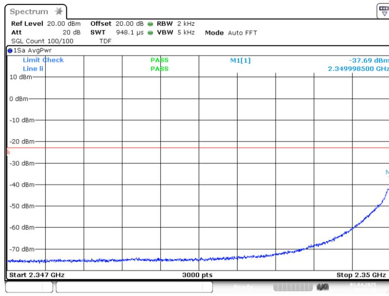
3.6.2 out of band emi WCS 2300 GSM lower lcarrier -0.3 dB 2.
