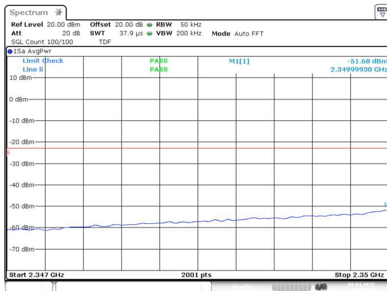
3.6.2 out of band emi WCS 2300 AWGN lower lcarrier +3.0 dB 2
