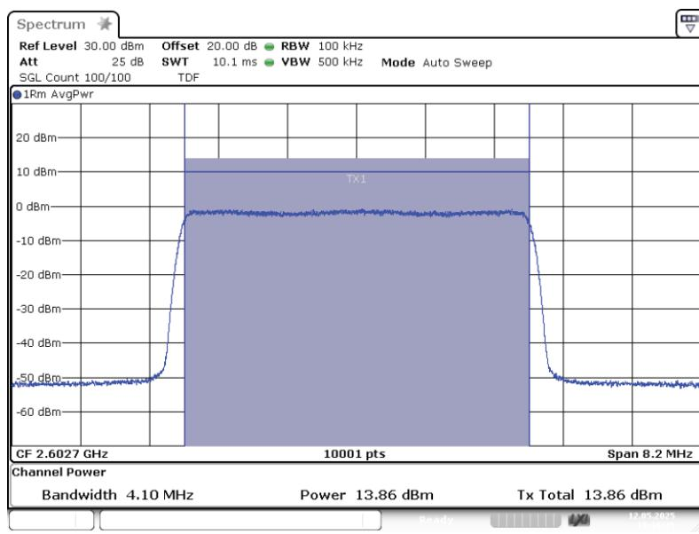
Band: BRS MBS, Antenna 1; Frequency: 2.6027 GHz; Band edge: f0; Mod: GSM;
