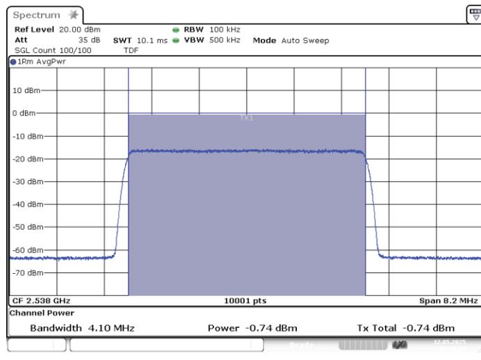
Band: BRS LBS, Antenna 1; Frequency: 2.5380 GHz; Band edge: f0; Mod: AWGN;
