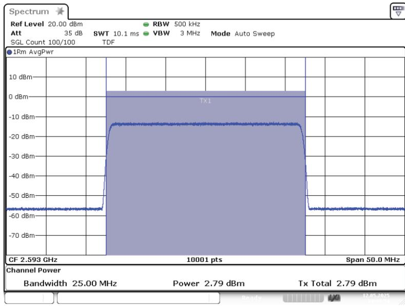
Band: BRS MBS, Antenna 1; Frequency: 2.5930 GHz; Band edge: mid; Mod: AWGN 25M;
