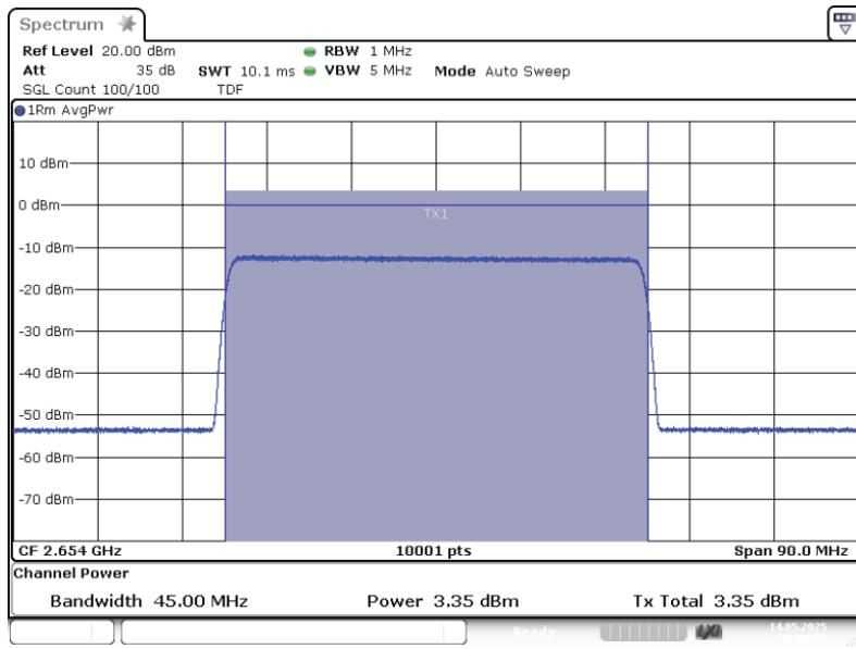
Band: BRS UBS, Antenna 1; Frequency: 2.6540 GHz; Band edge: mid; Mod: AWGN 45M;
