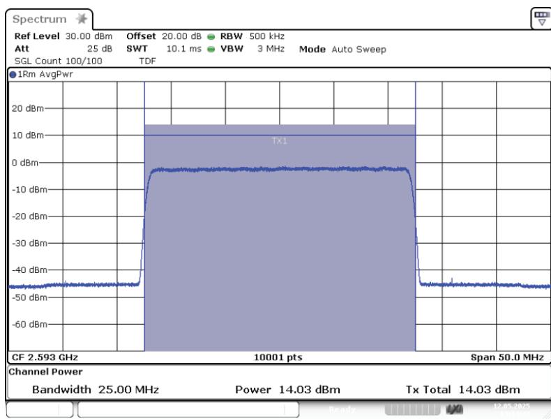
Band: BRS UBS, Antenna 1; Frequency: 2.6601 GHz; Band edge: f0; Mod: AWGN;
