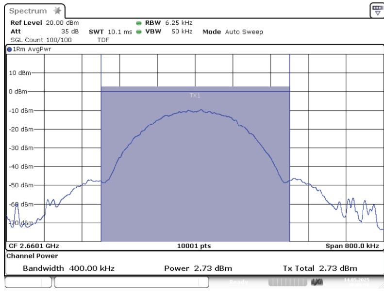
Band: BRS UBS, Antenna 1; Frequency: 2.6601 GHz; Band edge: f0; Mod: GSM;
