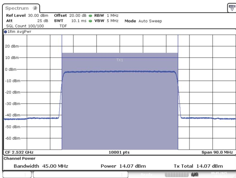
Band: BRS LBS, Antenna 1; Frequency: 2.5320 GHz; Band edge: mid; Mod: AWGN 45M;
