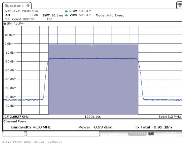
Band: BRS MBS, Antenna 1; Frequency: 2.6027 GHz; Band edge: f0; Mod: AWGN;
