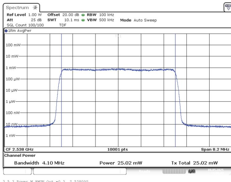
Band: BRS LBS, Antenna 1; Frequency: 2.5380 GHz; Band edge: f0; Mod: AWGN;
