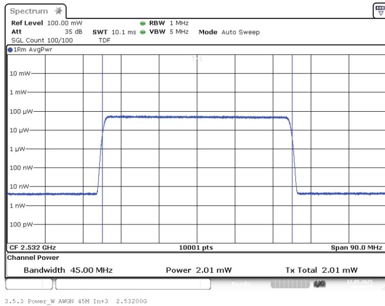
Band: BRS LBS, Antenna 1; Frequency: 2.5320 GHz; Band edge: mid; Mod: AWGN 45M;
