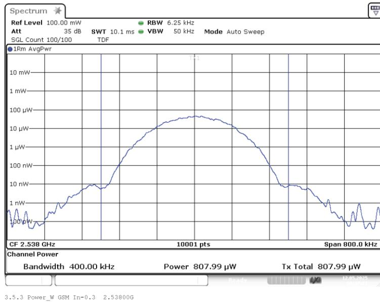
Band: BRS LBS, Antenna 1; Frequency: 2.5380 GHz; Band edge: f0; Mod: GSM;
