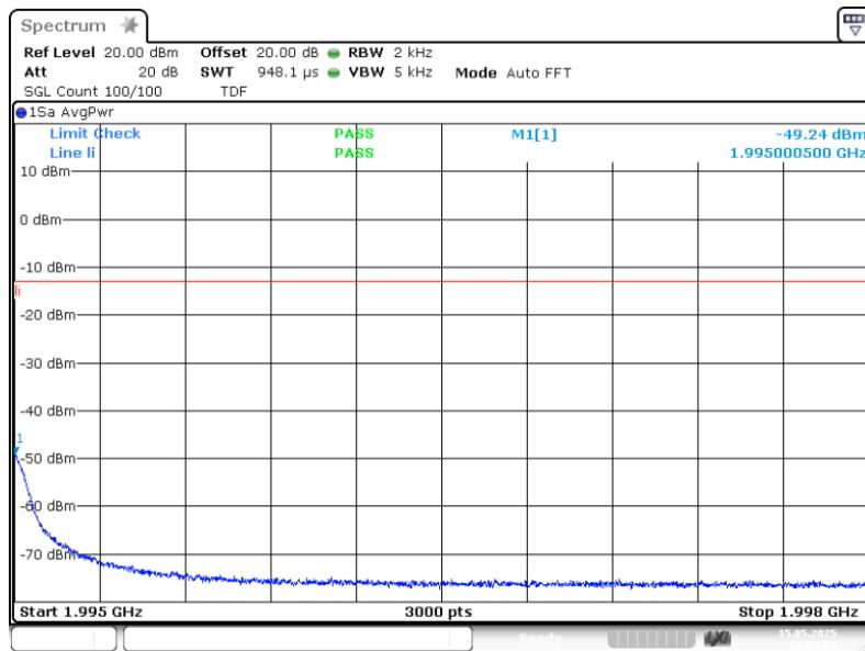
Band: PCS 1900, Antenna 1; Frequency: 1.9300 GHz to 1.9950 GHz; Band edge: upper; Mod: GSM; Input power = 3 dB > AGC; Number of signals 2
