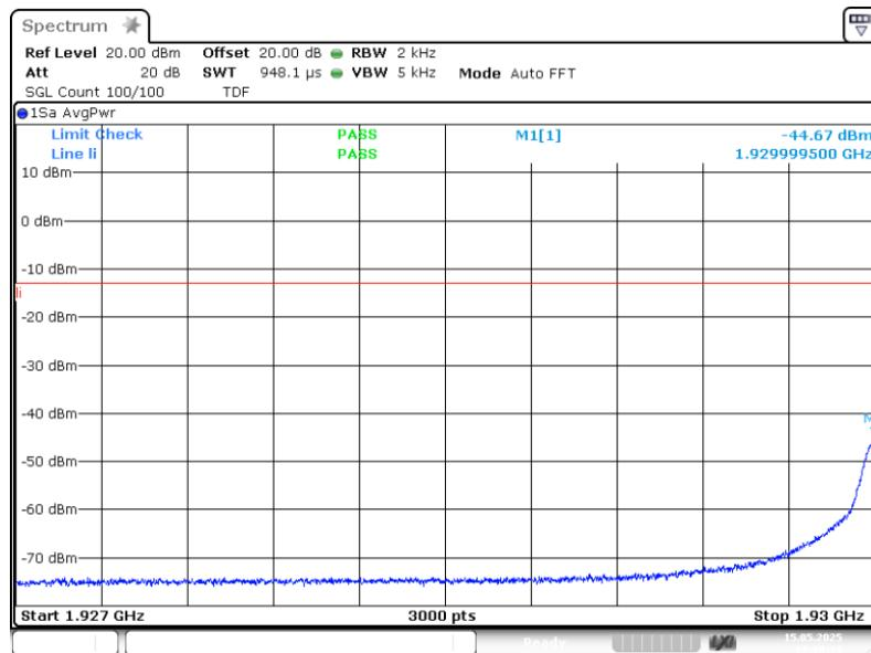
Band: PCS 1900, Antenna 1; Frequency: 1.9300 GHz to 1.9950 GHz; Band edge: lower; Mod: GSM; Input power = 3 dB > AGC; Number of signals 1
