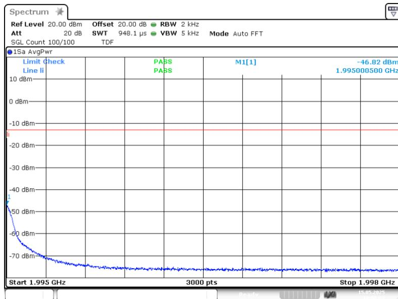
3.6.2 out of band emi PCS1900 A1 GSM upper 1carrier +3.0 dB
