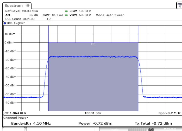
Band: PCS 1900, ANTENNA 1; Frequency: 1.9640 GHz; Band edge: f0; Mod: AWGN;
