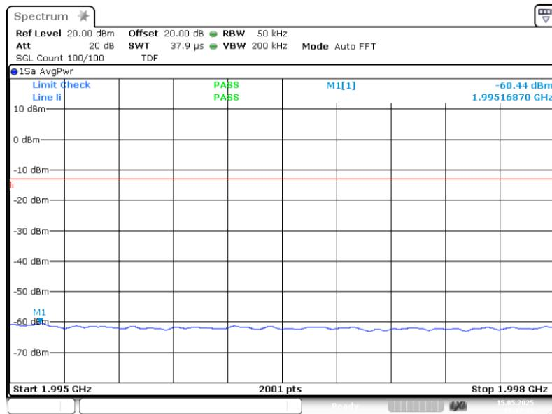
Band: PCS 1900, Antenna 1; Frequency: 1.9300 GHz to 1.9950 GHz; Band edge: upper; Mod: AWGN; Input power = 3 dB > AGC; Number of signals 2
