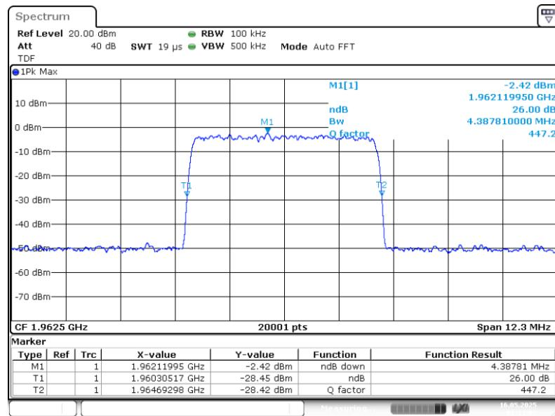
Band: PCS 1900 Antenna 1; Frequency: 1.9625 GHz; Band edge: mid; Mod: AWGN;
