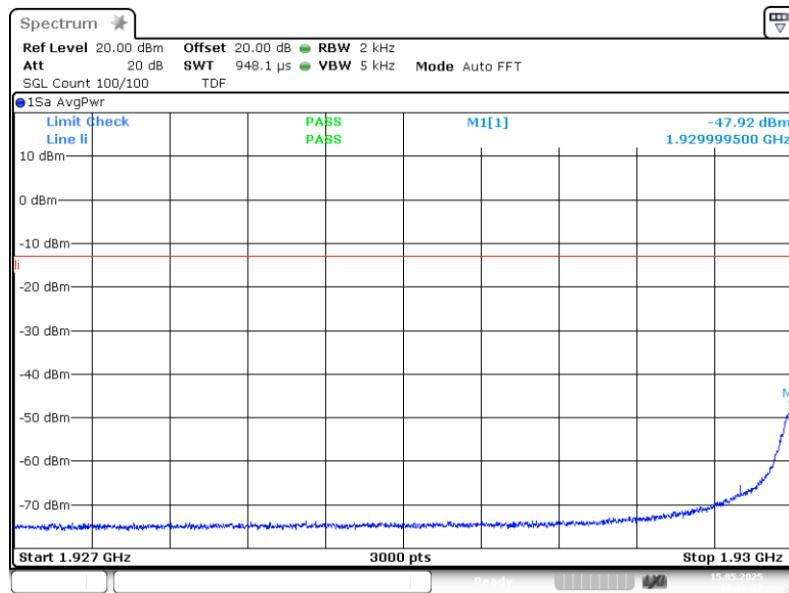
Band: PCS 1900, Antenna 1; Frequency: 1.9300 GHz to 1.9950 GHz; Band edge: lower; Mod: GSM; Input power = 3 dB > AGC; Number of signals 2
