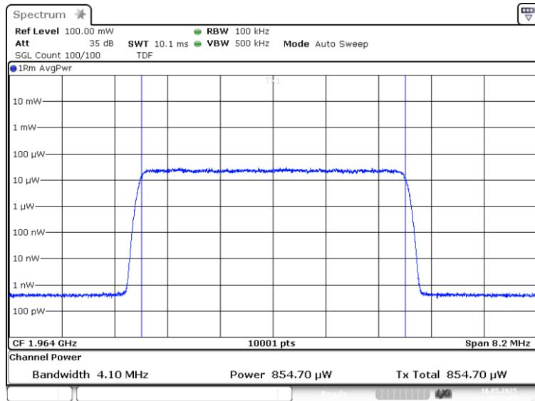
Band: PCS 1900, ANTENNA 1; Frequency: 1.9640 GHz; Band edge: f0; Mod: AWGN;
