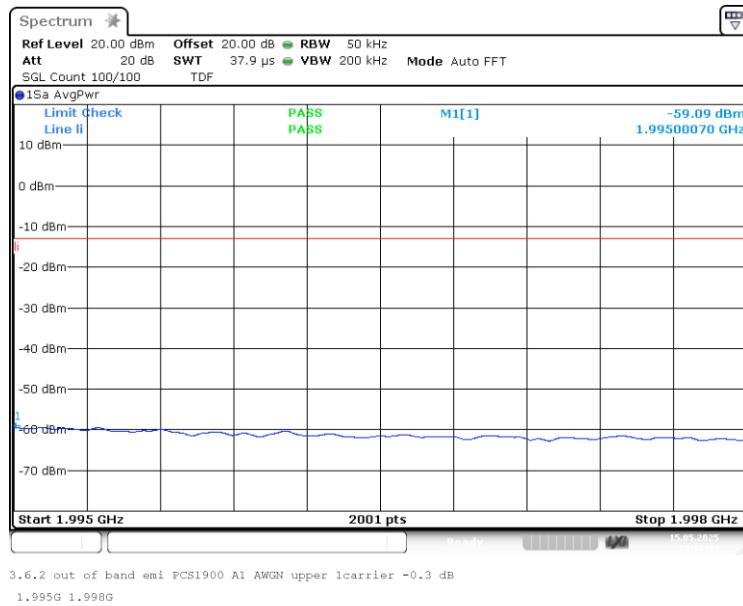
Band: PCS 1900, Antenna 1; Frequency: 1.9300 GHz to 1.9950 GHz; Band edge: upper; Mod: AWGN; Input power = 3 dB > AGC; Number of signals 1
