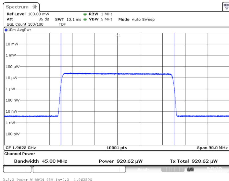
Band: PCS 1900, ANTENNA 1; Frequency: 1.9625 GHz; Band edge: mid; Mod: AWGN 45M;
