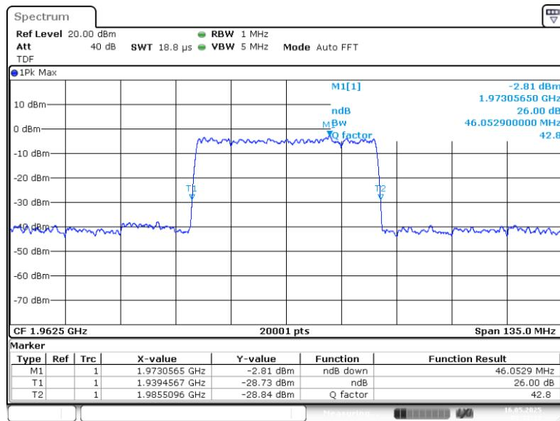
Band: PCS 1900 Antenna 1; Frequency: 1.9625 GHz; Band edge: mid; Mod: AWGN 45M; Output OCBw 3 dB > AGC
