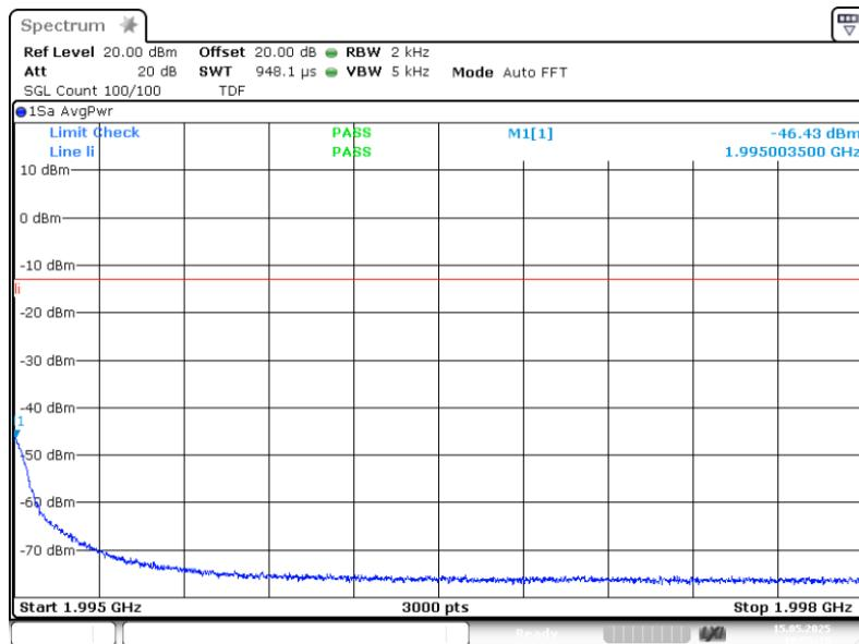
3.6.2 out of band emi PCS1900 A1 GSM upper 1carrier -0.3 dB
