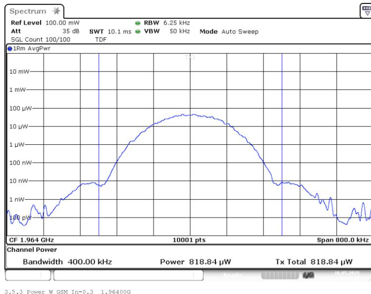
Band: PCS 1900, ANTENNA 1; Frequency: 1.9640 GHz; Band edge: f0; Mod: GSM;
