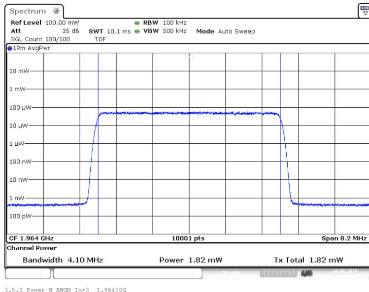
Band: PCS 1900, ANTENNA 1; Frequency: 1.9640 GHz; Band edge: f0; Mod: AWGN;
