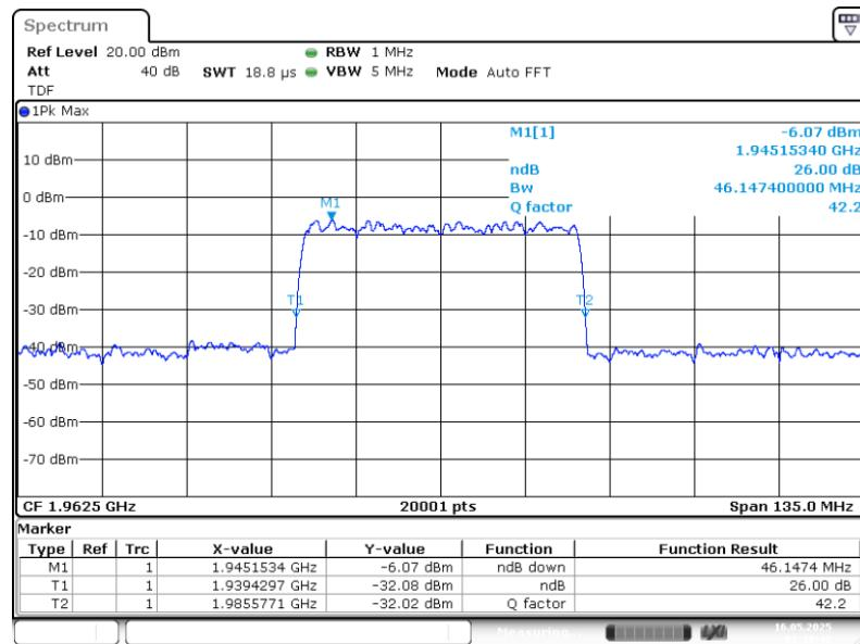
Band: PCS 1900 Antenna 1; Frequency: 1.9625 GHz; Band edge: mid; Mod: AWGN 45M;
