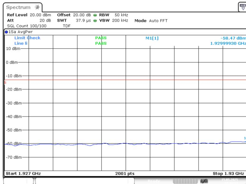
Band: PCS 1900, Antenna 1; Frequency: 1.9300 GHz to 1.9950 GHz; Band edge: lower; Mod: AWGN; Input power = 3 dB > AGC; Number of signals 2
