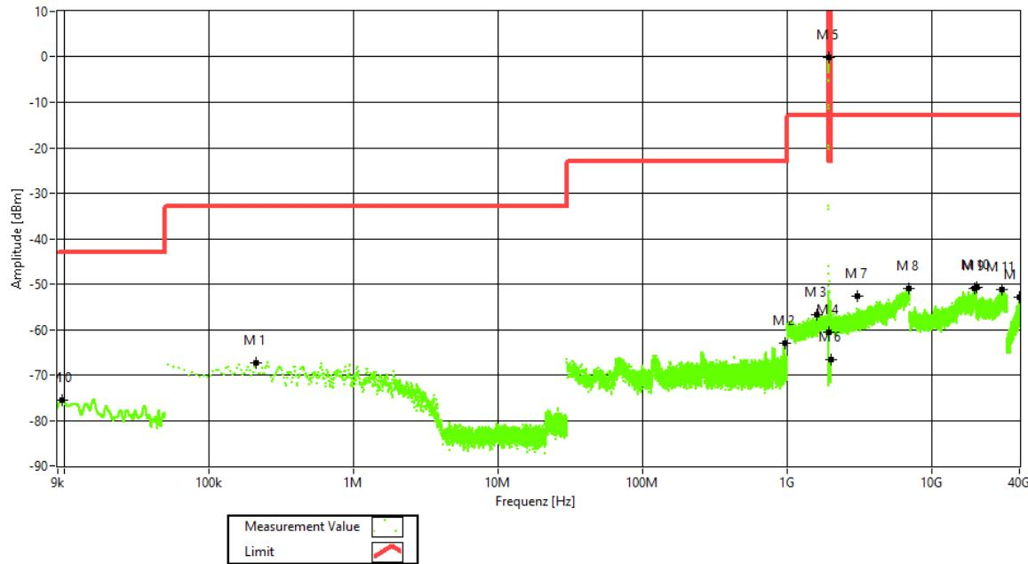
Frequency Band = PCS 1900, Antenna 1; Test frequency = mid; Direction = RF downlink;
