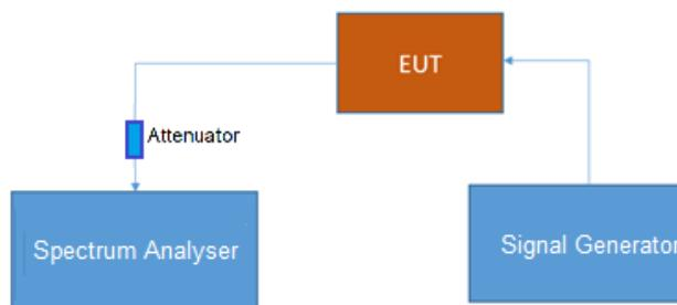
Test Setup step 2; Occupied Bandwidth/Input-versus-output spectrum
