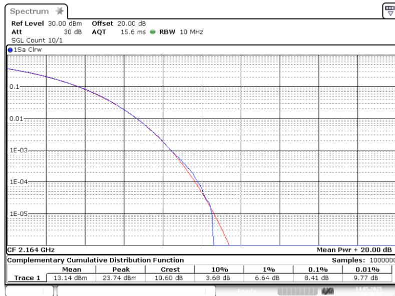
Band: AWS 1700, Antenna 1; Frequency: 2.1640 GHz; Bande edge: f0; Mod: AWGN;
