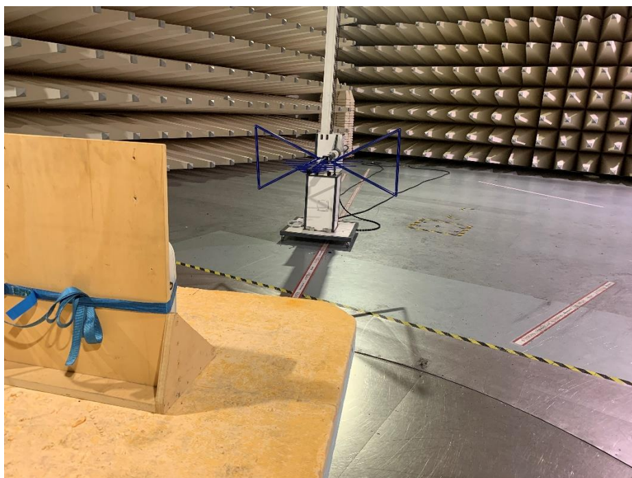
Photograph 3: Setup of radiated emissions measurement in the frequency range 30 – 1000 MHz
