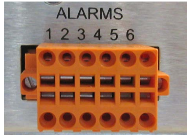
Mating connector inserted into WCS alarm port
