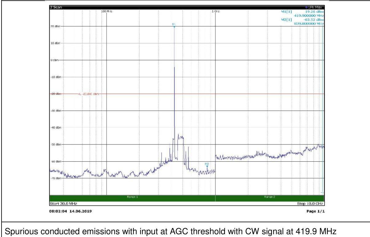
Spurious conducted emissions with input at AGC threshold with CW signal at 419.9 MHz
