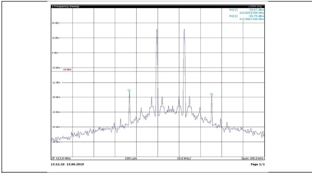
Out of band/out of block with input at AGC threshold + 3 dB with CW signal at 413 MHz
