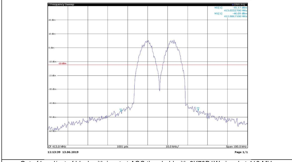
Out of band/out of block with input at AGC threshold with 8K70D1W signal at 413 MHz
