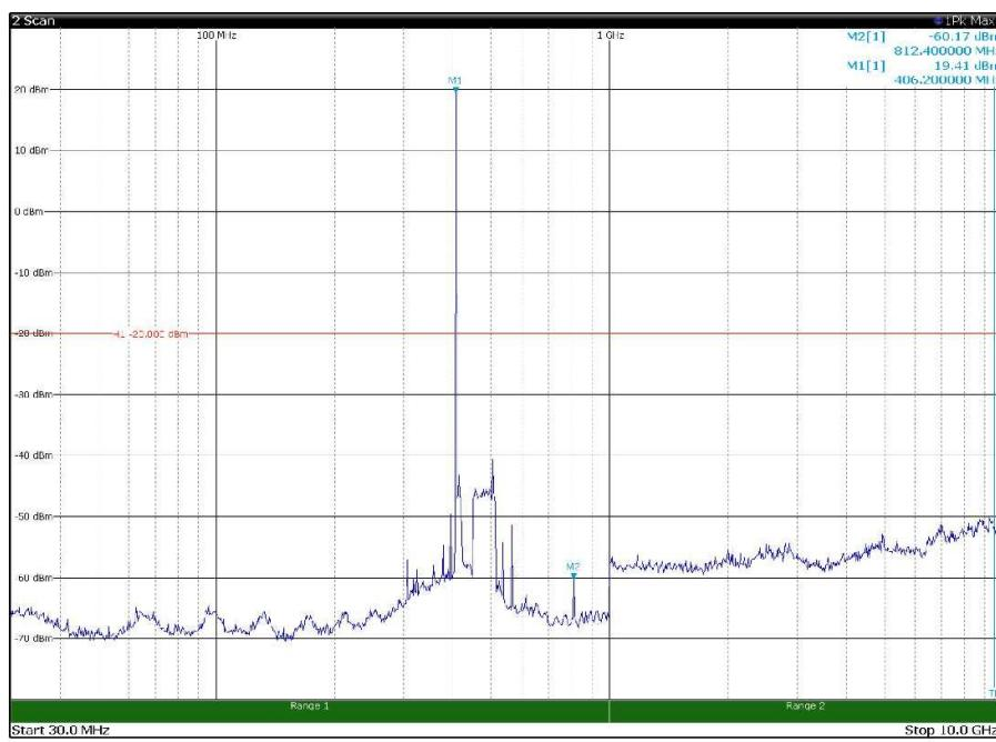
Spurious conducted emissions with input at AGC threshold with CW signal at 406.2 MHz
