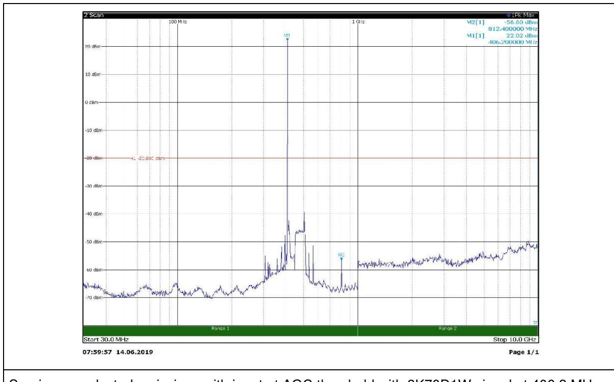
Spurious conducted emissions with input at AGC threshold with 8K70D1W signal at 406.2 MHz
