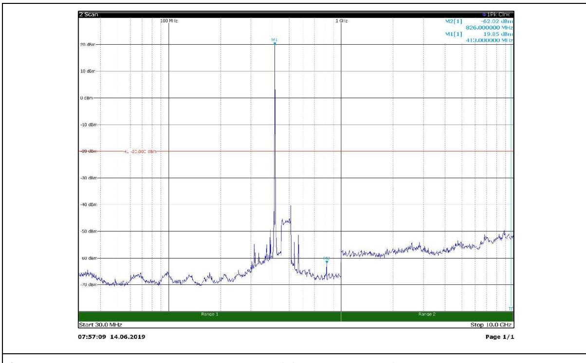
Spurious conducted emissions with input at AGC threshold with CW signal at 413 MHz
