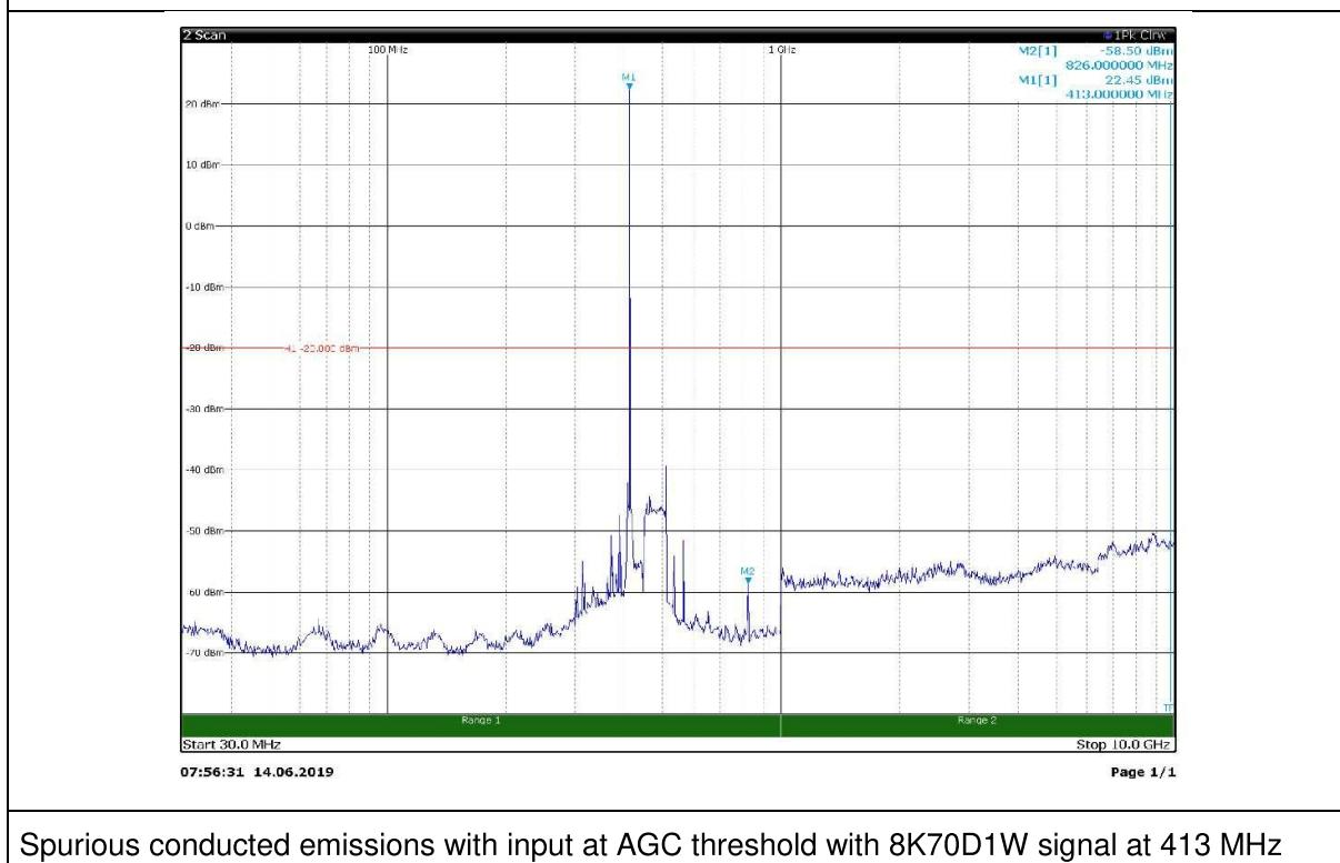
Spurious conducted emissions with input at AGC threshold with 8K70D1W signal at 413 MHz
