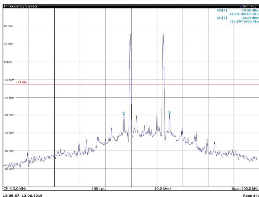
Out of band/out of block with input at AGC threshold with CW signal at 413 MHz
