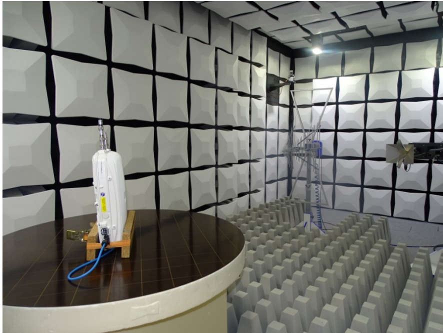
Photo 3: Test setup for radiated emissions measurements in fully-anechoic chamber (1 GHz to 27 GHz), rear side view
