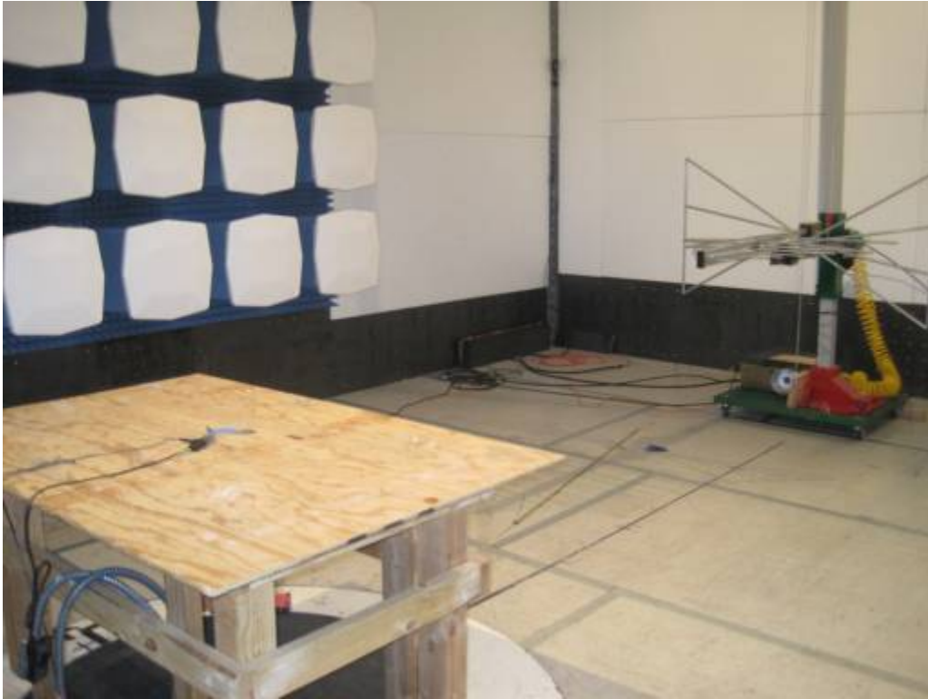
Radiated Emission 30MHz to 1GHz
