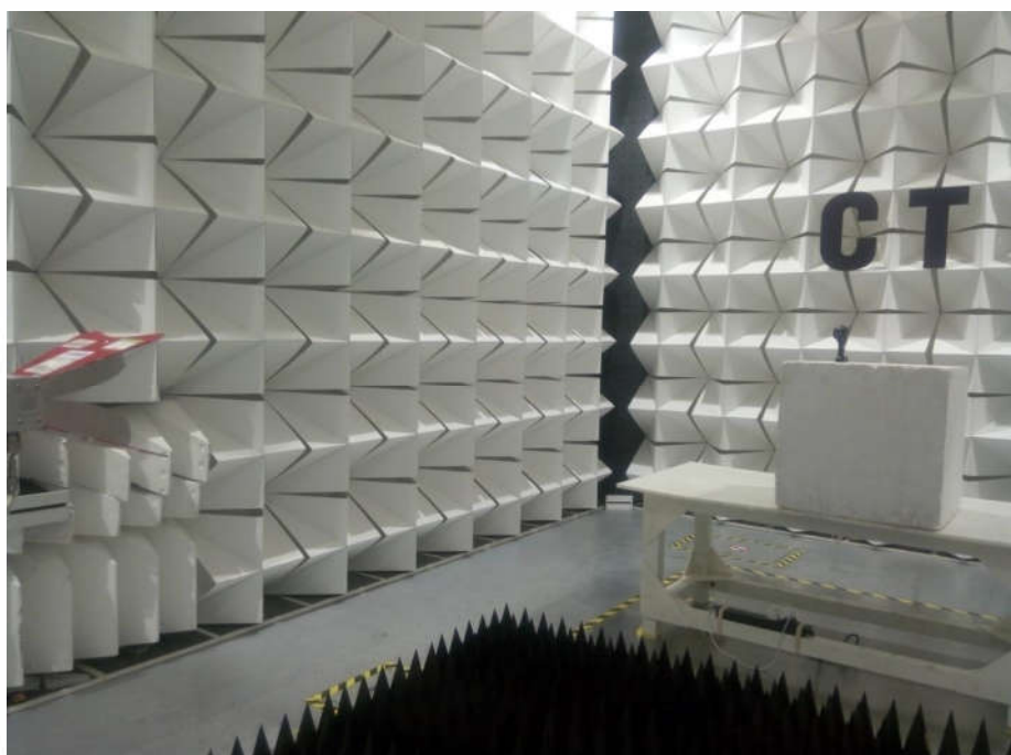
Radiated spurious emission Test Setup-2(Above 1GHz)
