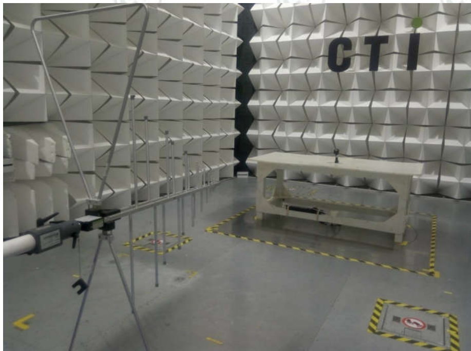
Radiated emission Test Setup-1(30MHz~1GHz)
