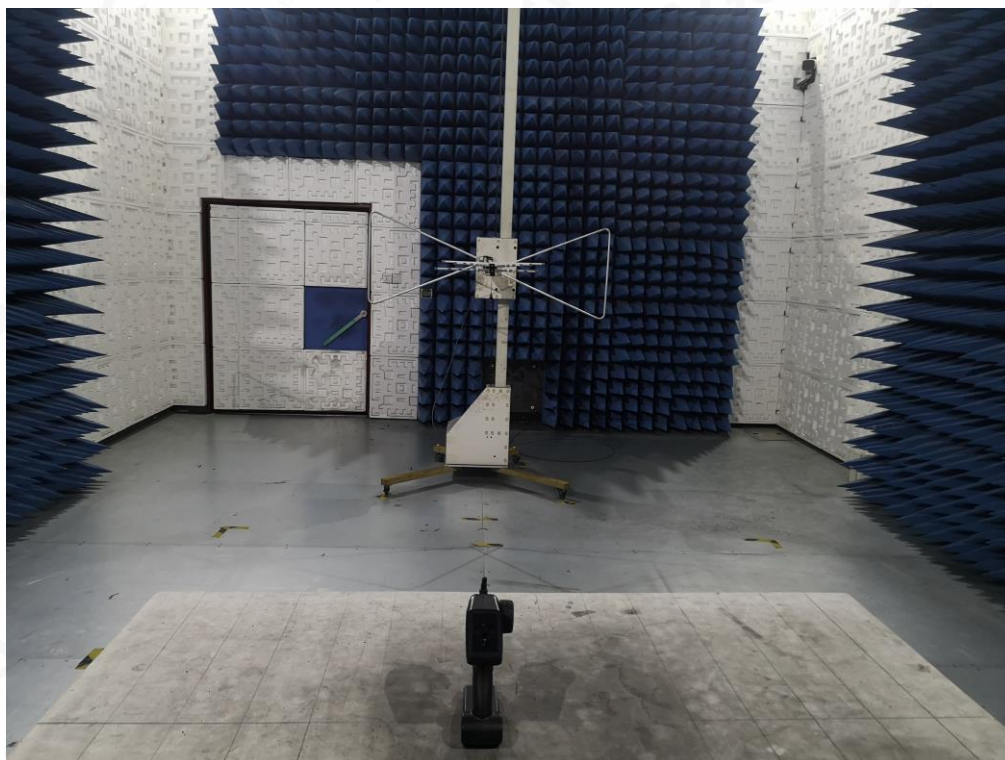
FCC RADIATED EMISSION TEST SETUP ABOVE 1GHZ
