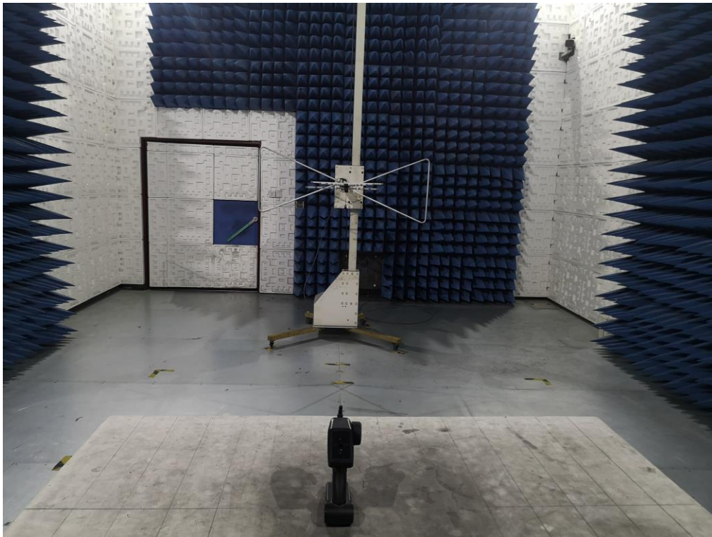
FCC RADIATED EMISSION TEST SETUP ABOVE 1GHZ
