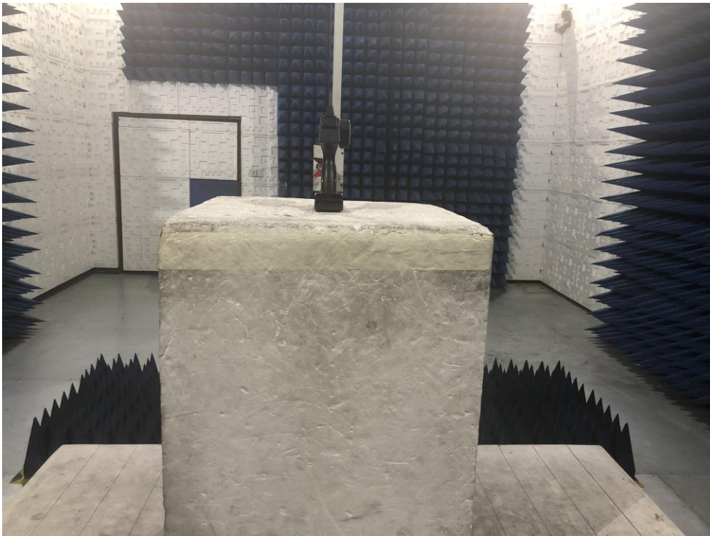
RADIATED EMISSION TEST SETUP ABOVE 1GHZ
