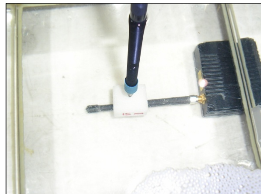
Figure 12: Positional Photograph of the SOLO Transmitter in Rear Facing Position.
