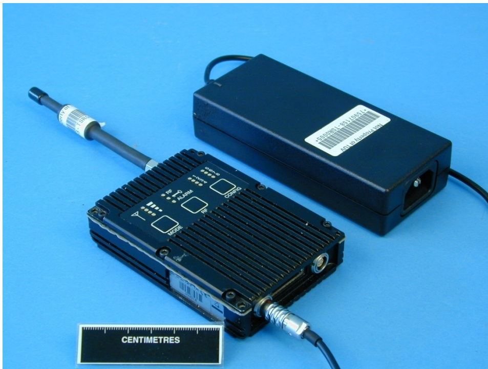
Figure 15: Device 1 – SOLO Transmitter with Power Supply Unit
