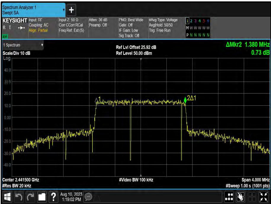
Figure 42 - 1.50 MHz Maximum 99% OBW
