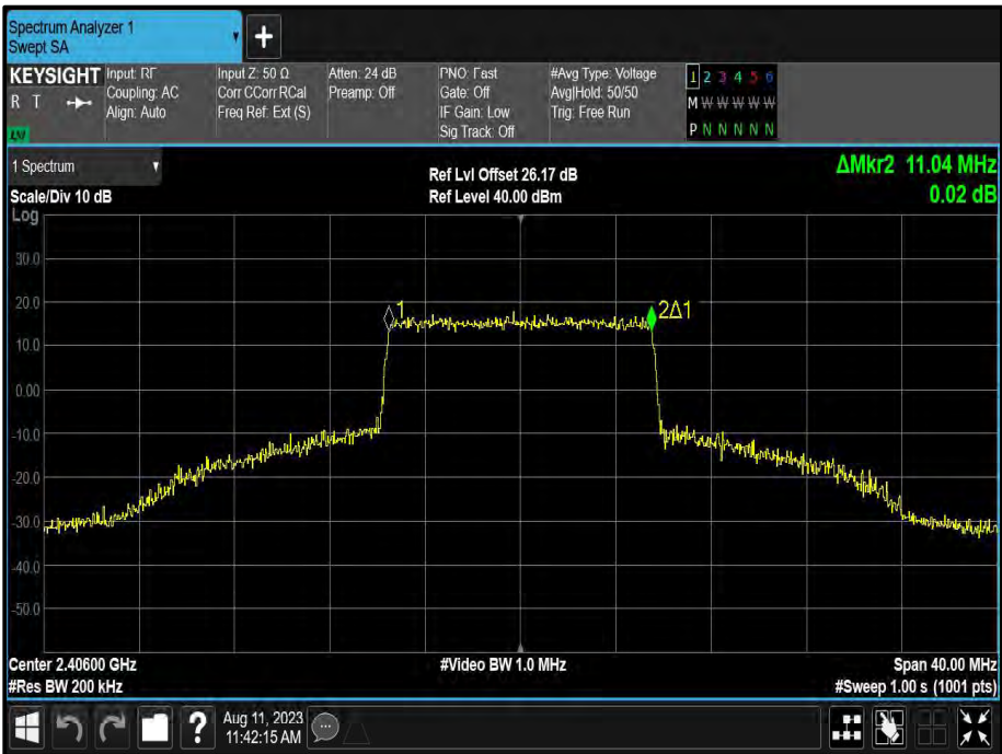
Figure 62 - 12.00 MHz Maximum 99% OBW
