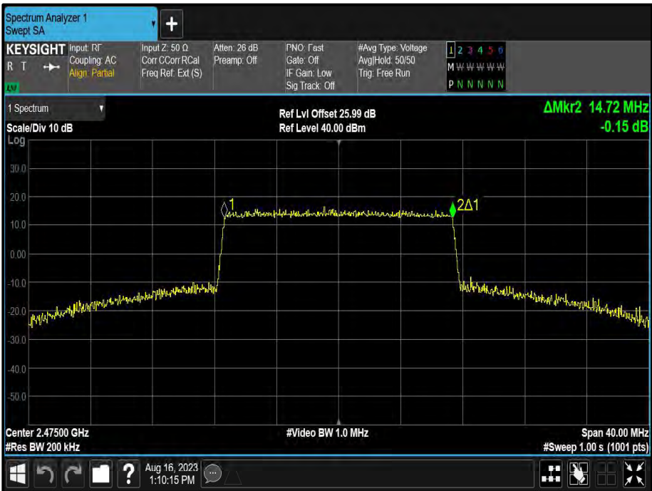
Figure 66 - 16.00 MHz Maximum 99% OBW
