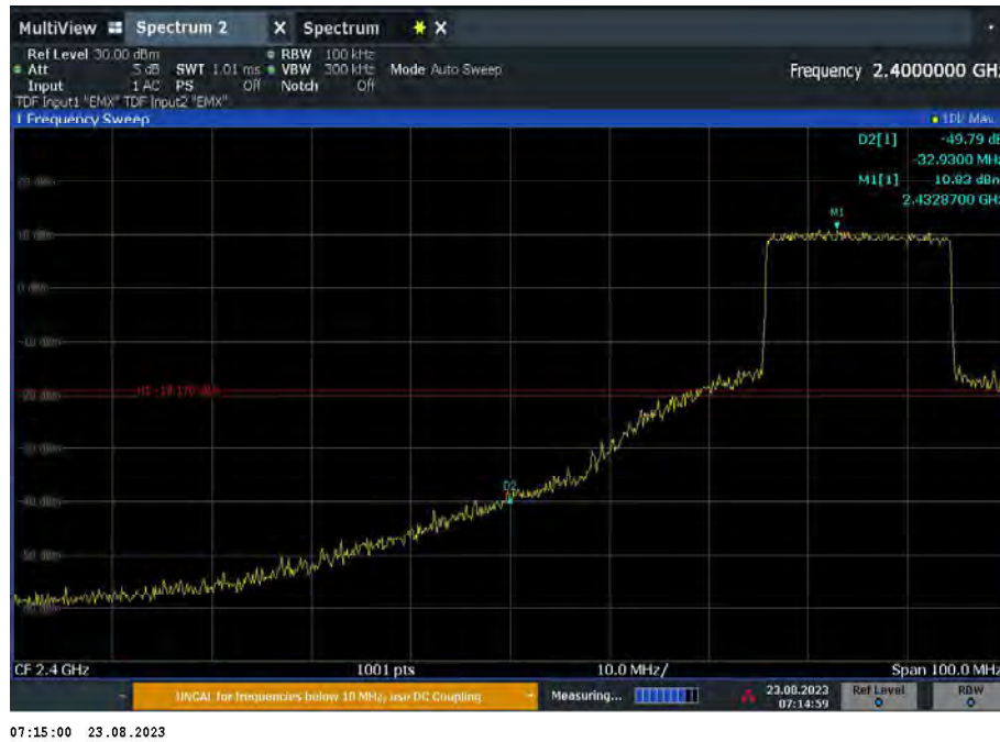
Figure 71 - Port A_Bot_Channel_MIMO_SDM_20MHz_X Plane, 2435 MHz, Band Edge Frequency 2400 MHz
