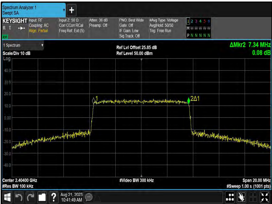
Figure 57 - 8.00 MHz Minimum 99% OBW
