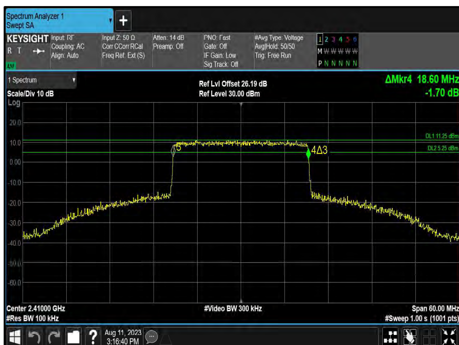
Figure 38 - 20.00 MHz Maximum 6 dB EBW
