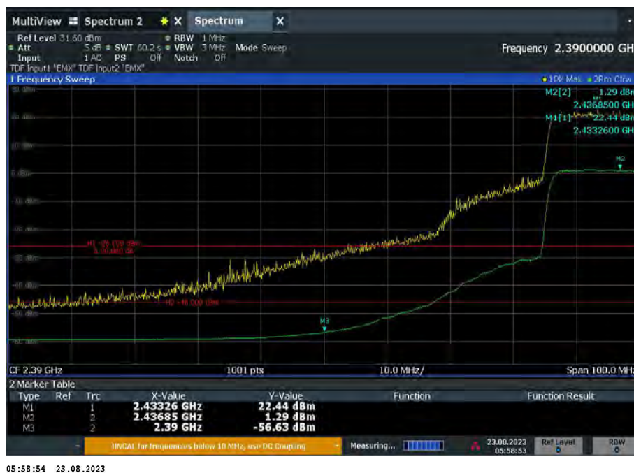
Figure 7 - Port B_Bot_Channel_MIMO_SDM_20MHz_X Plane, 2435 MHz, Band Edge Frequency 2390 MHz
