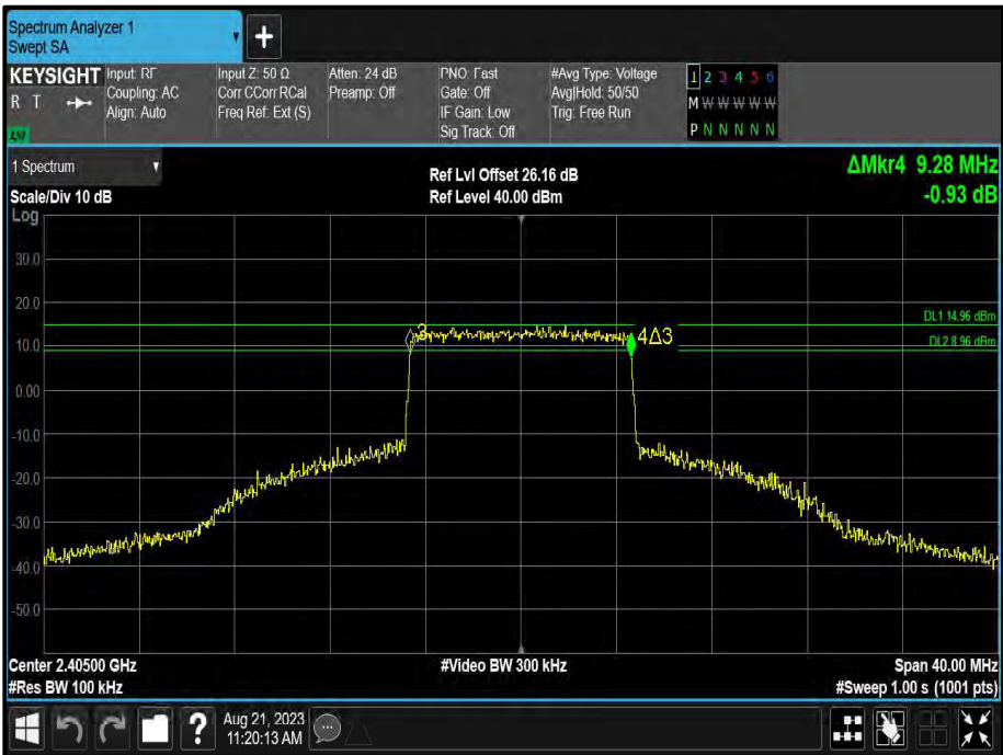
Figure 29 - 10.00 MHz Minimum 6 dB EBW
