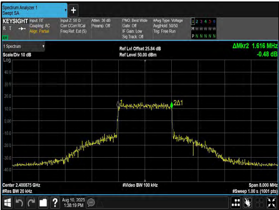
Figure 44 - 1.75 MHz Maximum 99% OBW
