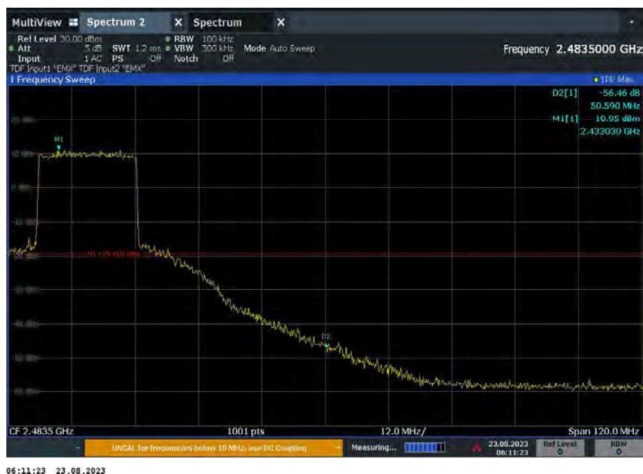
Figure 76 - Port B_Top_Channel_MIMO_SDM_20MHz_X Plane, 2438.5 MHz, Band Edge Frequency 2483.5 MHz
