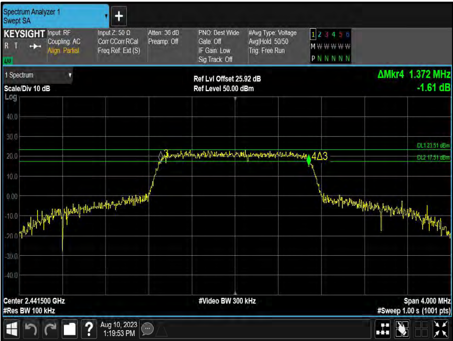
Figure 11 - 1.50 MHz Minimum 6 dB EBW
