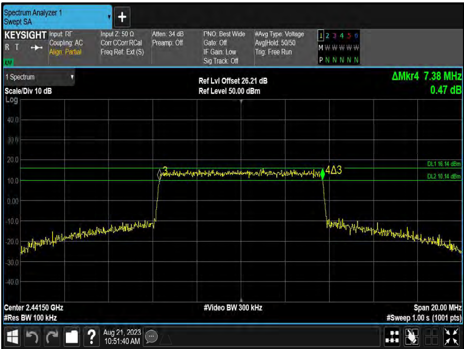
Figure 27 - 8.00 MHz Minimum 6 dB EBW
