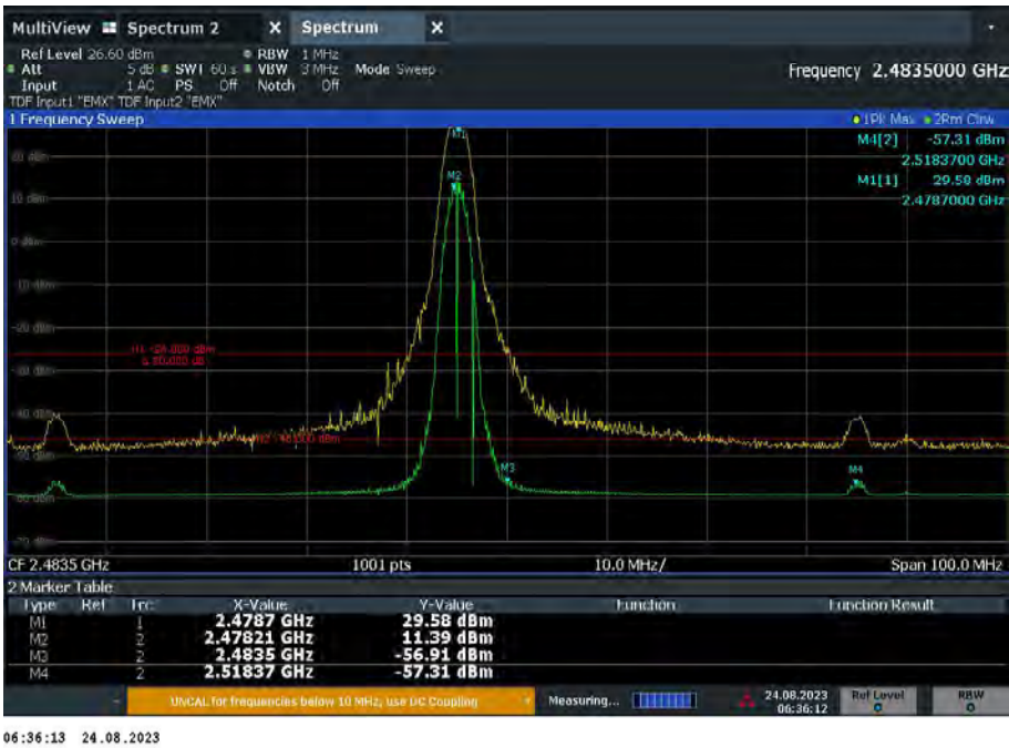
Figure 2 - Port A_Top_Channel_MIMO_SDM_1.25MHz_X Plane, 2478.50 MHz, Band Edge Frequency 2483.5 MHz
