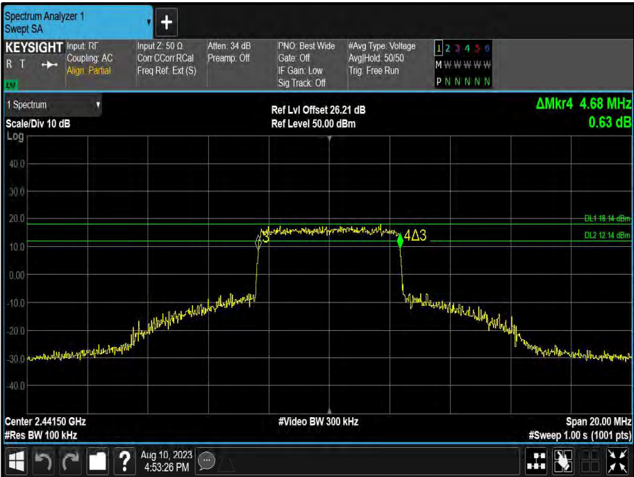
Figure 22 - 5.00 MHz Maximum 6 dB EBW
