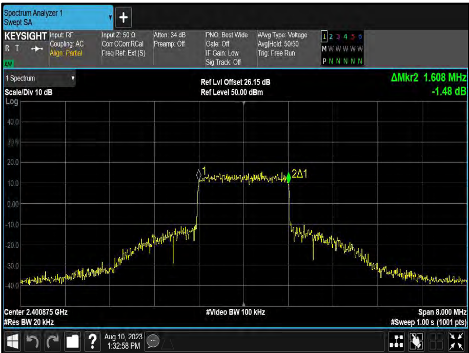
Figure 43 - 1.75 MHz Minimum 99% OBW
