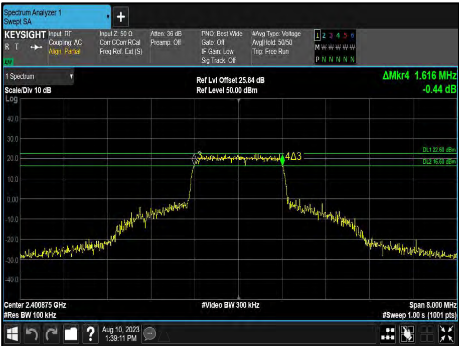
Figure 13 - 1.75 MHz Minimum 6 dB EBW
