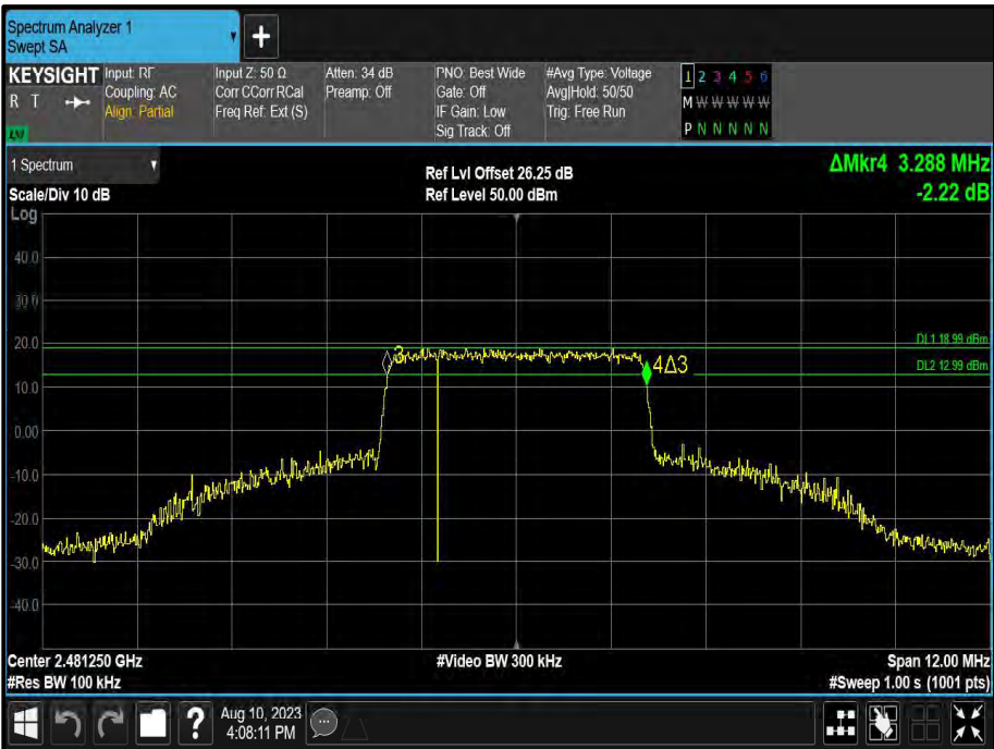
Figure 20 - 3.50 MHz Maximum 6 dB EBW
