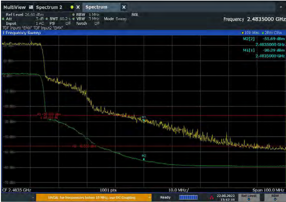
Figure 4 - Port A_Top_Channel_MIMO_SDM_20MHz_X Plane, 2438.5 MHz, Band Edge Frequency 2483.5 MHz
