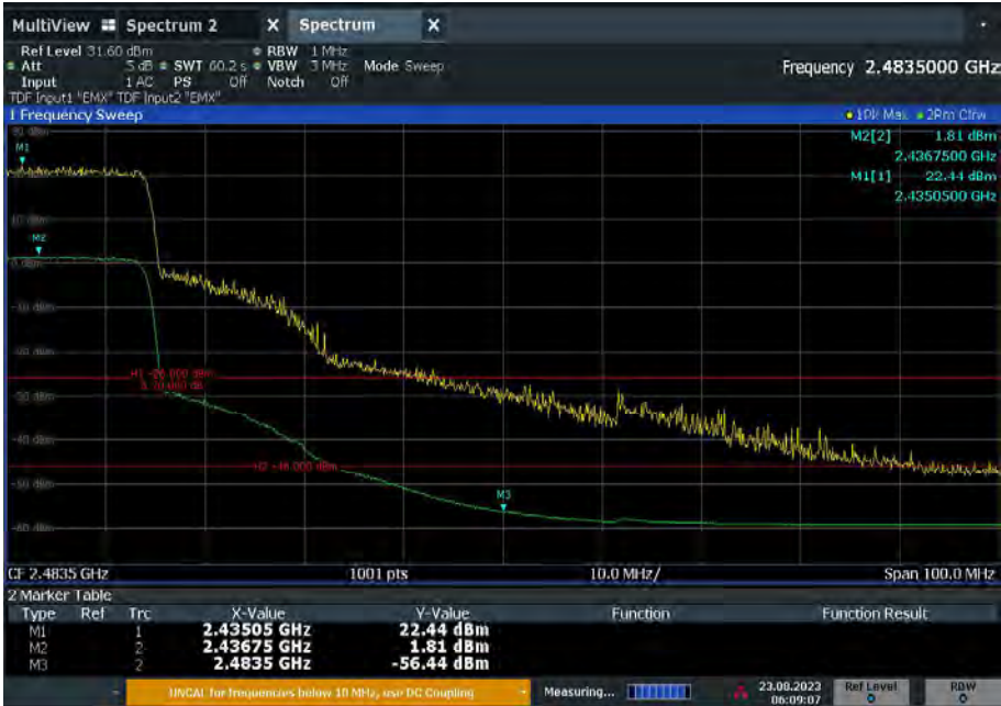
Figure 8 - Port B_Top_Channel_MIMO_SDM_20MHz_X Plane, 2438.5 MHz, Band Edge Frequency 2483.5 MHz
