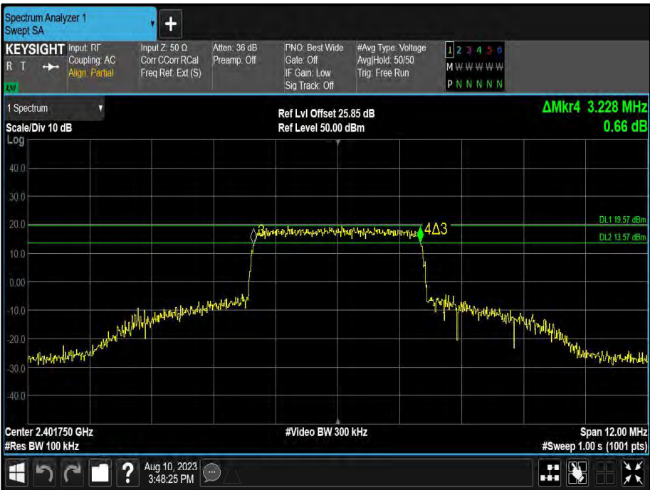
Figure 19 - 3.50 MHz Minimum 6 dB EBW
