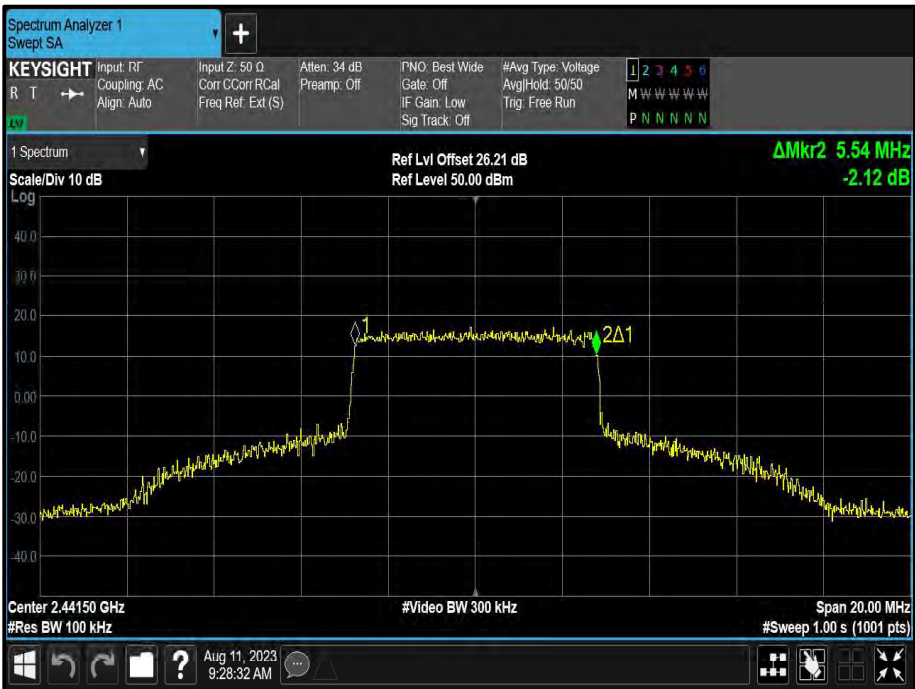
Figure 54 - 6.00 MHz Maximum 99% OBW
