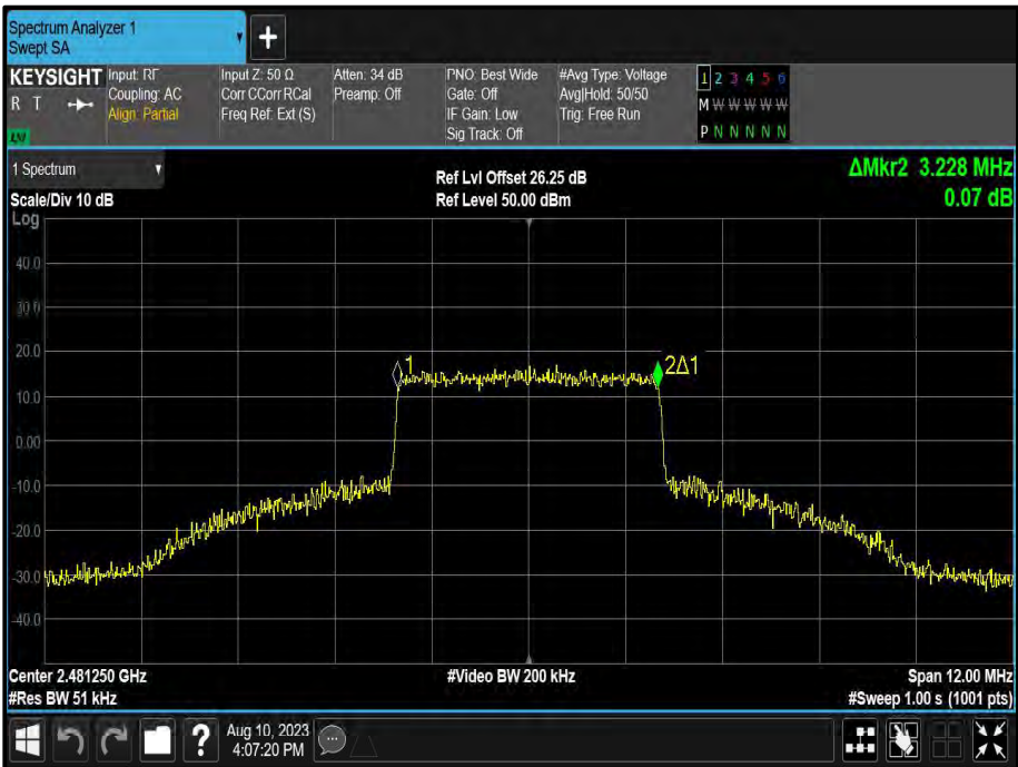
Figure 50 - 3.50 MHz Maximum 99% OBW
