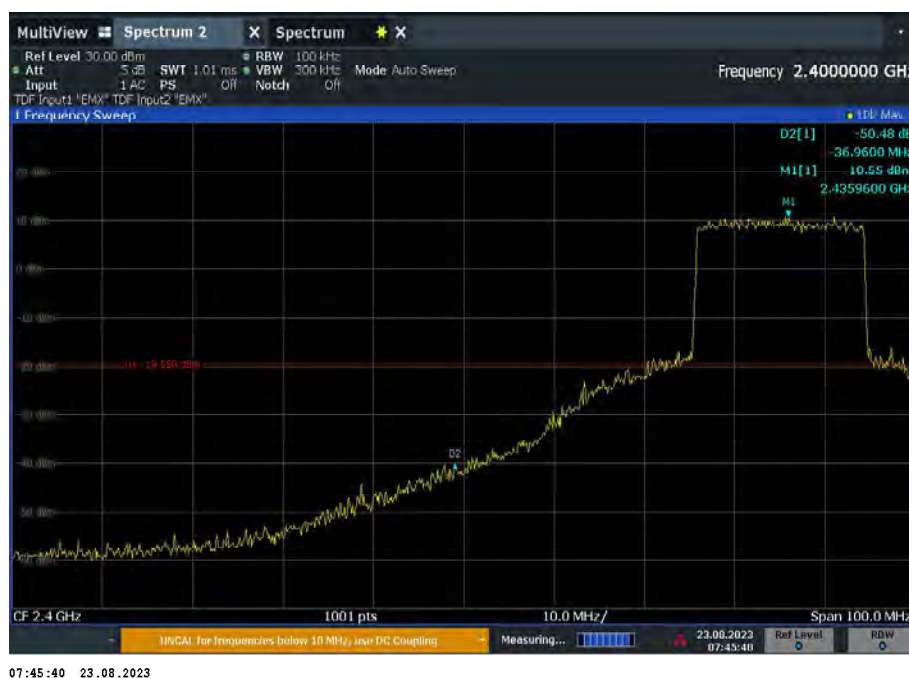
Figure 75 - Port B_Bot_Channel_MIMO_SDM_20MHz_X Plane, 2435 MHz, Band Edge Frequency 2400 MHz
