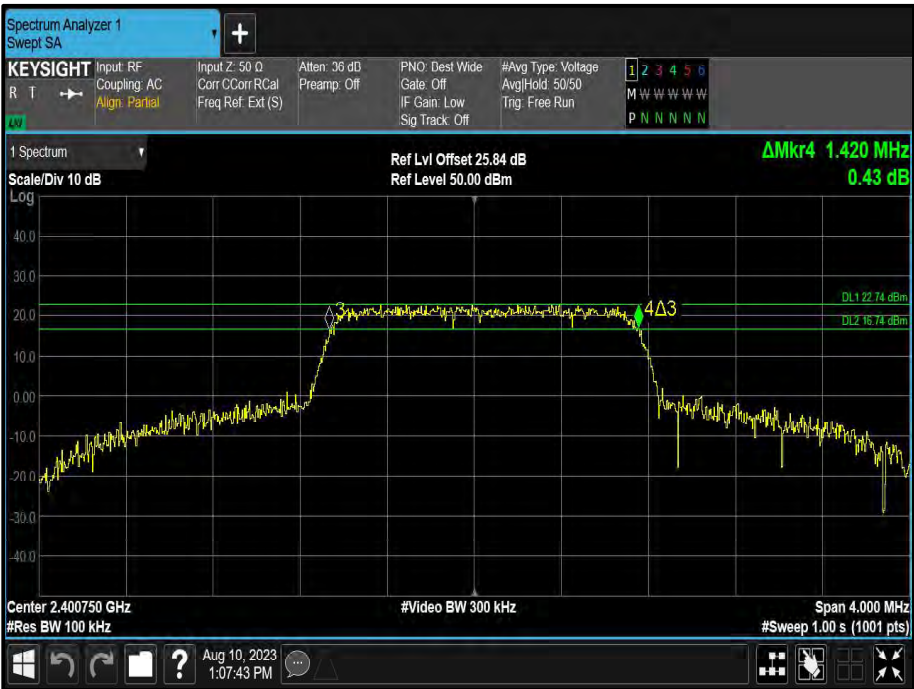
Figure 12 - 1.50 MHz Maximum 6 dB EBW
