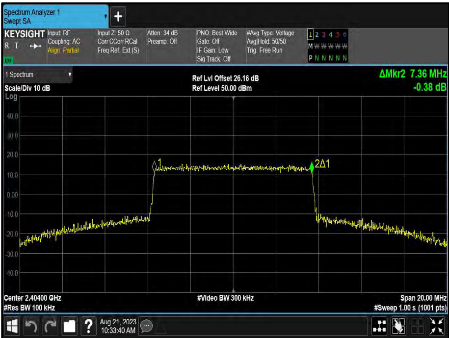
Figure 58 - 8.00 MHz Maximum 99% OBW
