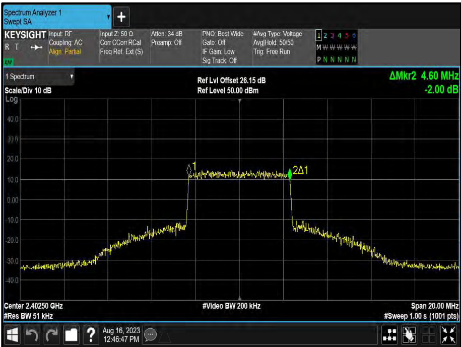
Figure 52 - 5.00 MHz Maximum 99% OBW
