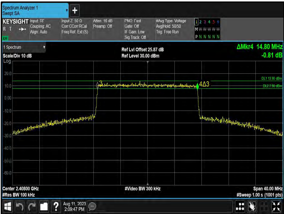
Figure 35 - 16.00 MHz Minimum 6 dB EBW
