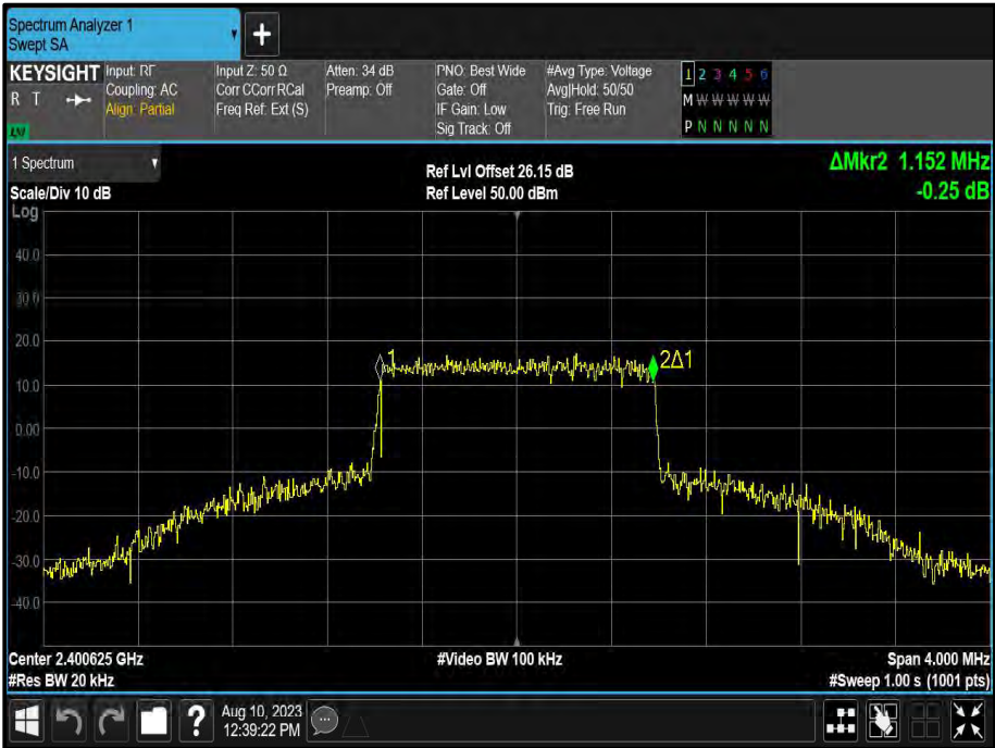
Figure 40 - 1.25 MHz Maximum 99% OBW
