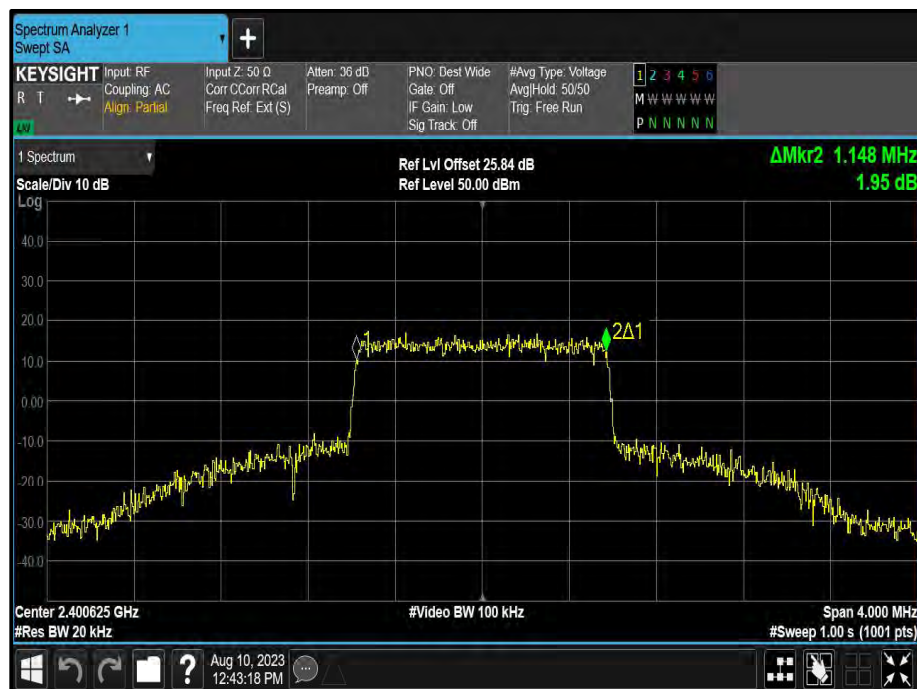
Figure 39 - 1.25 MHz Minimum 99% OBW
