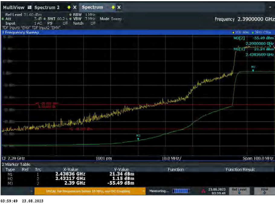
Figure 3 - Port A_Bot_Channel_MIMO_SDM_20MHz_X, 2435 MHz, Band Edge Frequency 2390 MHz
