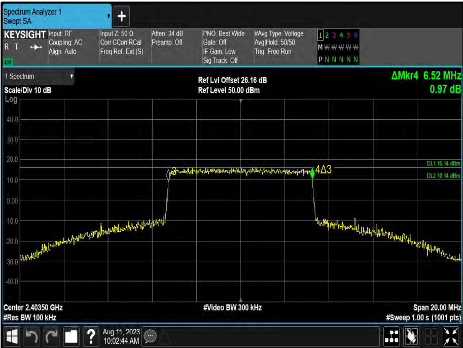
Figure 26 - 7.00 MHz Maximum 6 dB EBW
