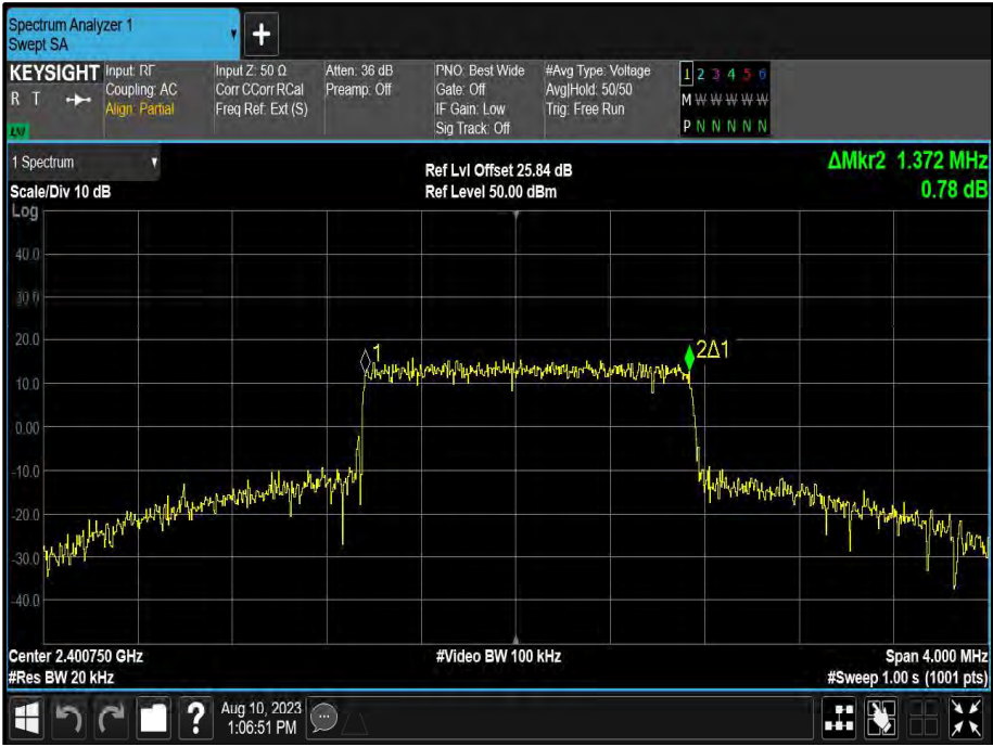
Figure 41 - 1.50 MHz Minimum 99% OBW
