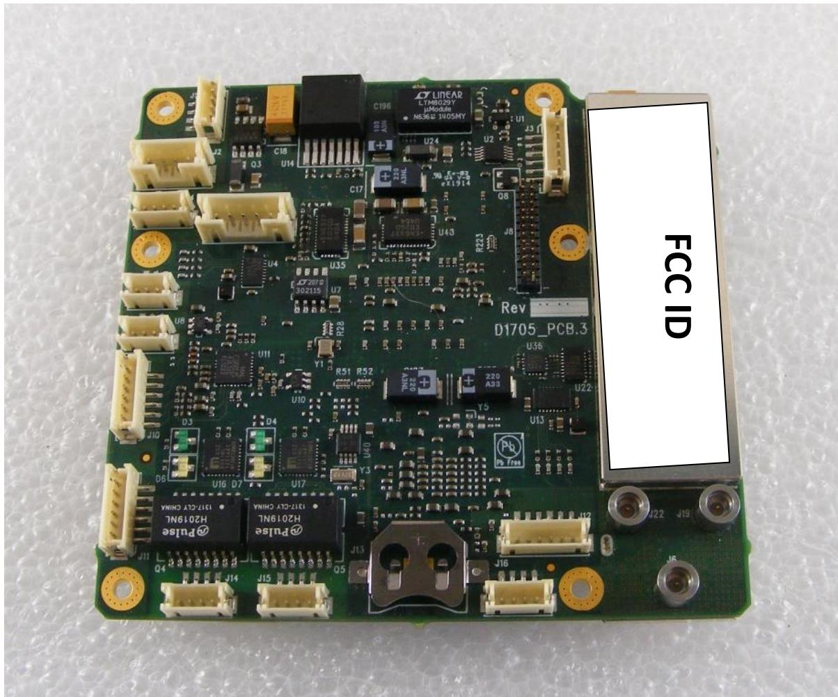
Diagram to show FCC ID is located on the shielding can, which is permanently fixed to the device.
